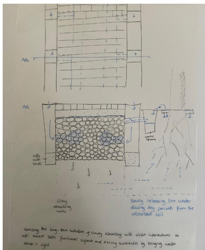
FIGURE 129 | SECTION INFILTRATION PRINCIPLE
