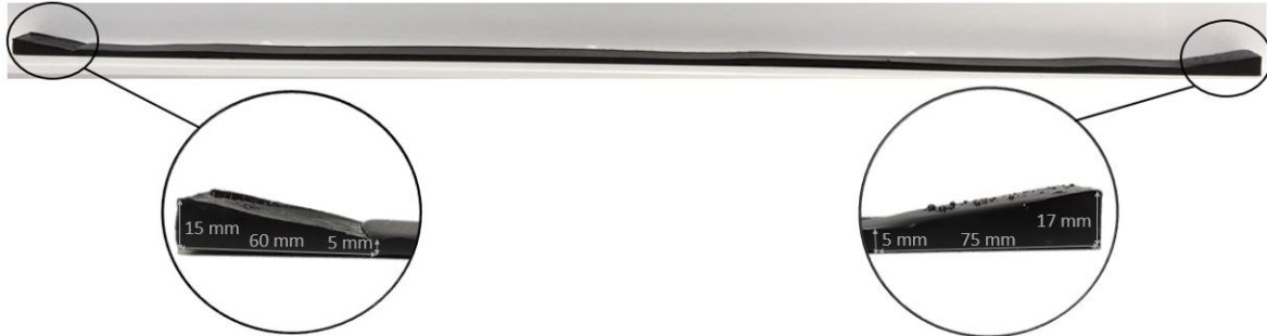
Figure 5.17: Result of a simplified PUR subframe based on the CAD data of a four-door vehicle
