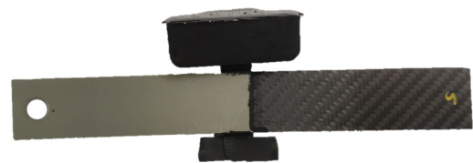
(a) Lap-shear specimen directly after PUR injection
