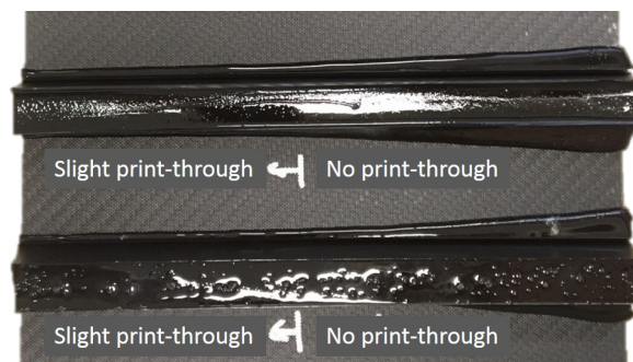
Figure 5.20: Image of a plate with spilling on the PUR edges without print-through on one side and sharp edge with print-through on the other
