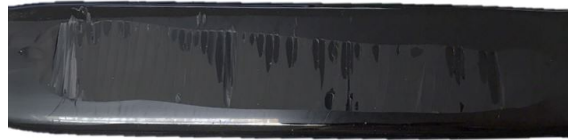
(b) Peel result of DA 620 on the PUR using primer
