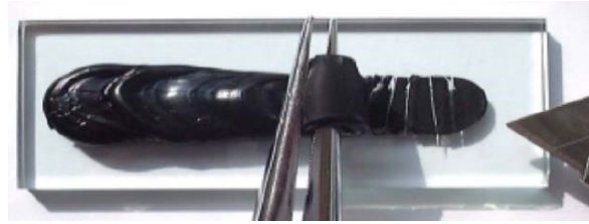
Figure 2.15: Peel-off test of an adhesive [39]
