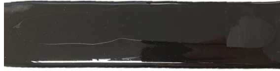
(a) Peel result of DA 620 on the PUR without pre-treatment
