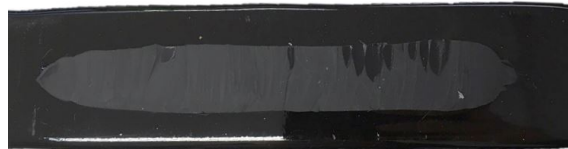
(c) Peel result of DA 620 on the PUR with mixing ratio 100:64
