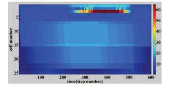
Fig. 7. Traffic density of every cell with traffic control when disturbance happens
