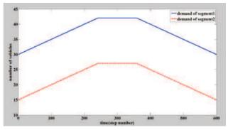
Fig. 4. Demand of origin 1 and 2. The peak demand of cell 1 is 42veh/step and cell 2 is 27veh/step.
