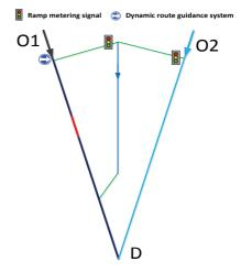
Fig. 2. Conceptual network of the case study. There are two origins and one destination in this network. The network contains five heterogeneous links. The black line represents freeway; red line represents disturbance areas; light blue line represents major arterial road, dark blue line is urban road and green line are ramps. There are two RMSs and one DRGS in this network control system.
