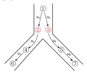
Fig. 1. Description of cells and links of a network. Red cells are decision cells.
