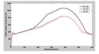
Fig. 10. Total vehicle number in the network of scenario 2 when N=1, 2, 5.
