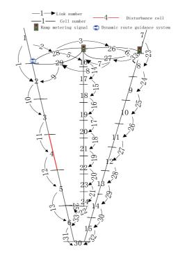
Fig. 3. The traffic network of the case study consist of two origins 1, 7 and one destination 30. Three paths from left to right are freeway, urban road and major arterial road. Numbers on the solid line denotes cell number; numbers on the dashed line denotes link number.
