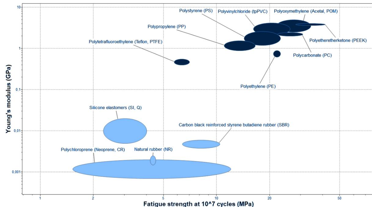
Figure C-2. Initial selection of materials for creating the flow cell connector.
