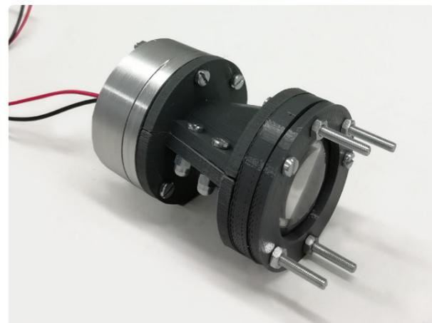
Figure D-2. Improved laser module embodiment design.
