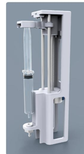
Figure F-1. The digital design of the initial fluid insertion system.
