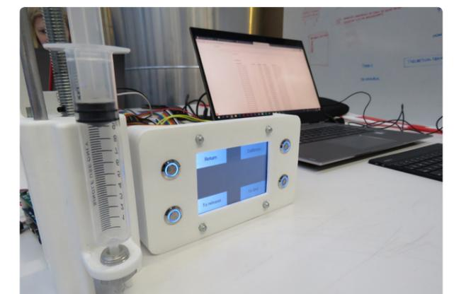
Figure F-3. Controlling the fluid insertion system using rough interface designs
