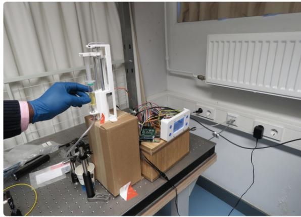
Figure F-4. Setup for validating the performance of the initial fluid insertion system.
