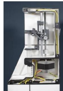
Figure 5. Fluid insertion system
