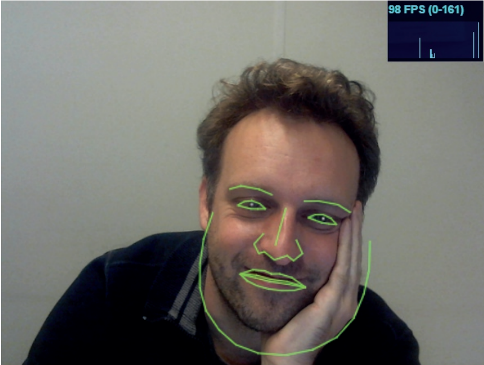
Figure 5.1: Face fitting model generated by CLM . This example shows a common face fitting error due to hand positioning.
