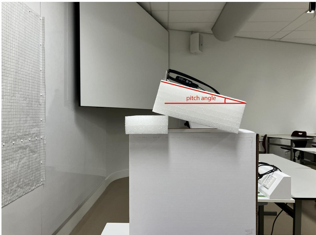
*Figure 3.7.* Setup for estimating the  $VD$  parameter. Graph paper consisting of  $1 \times 1$  cm squares was stuck to the wall, and the Tobii was located at a distance of approximately 1 m from the wall.
