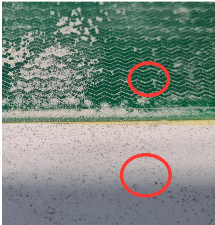
Figure C.4: Experimental observation finer dust stays on the electrodes than larger particles
