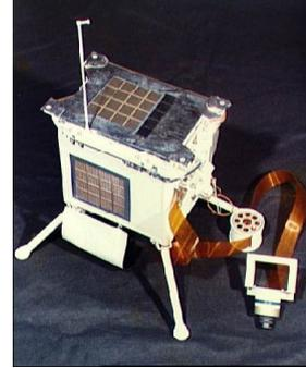
Figure 3.6: The LEAM detector unit, from [16]. On top the detector that measured the relevant data.
