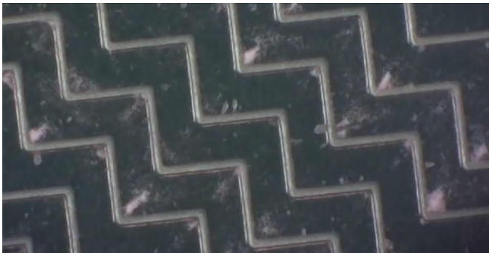
Figure 6.10: Small particles not removed
