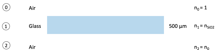
Figure 3.8: Sketch of the thick layer of glass.
