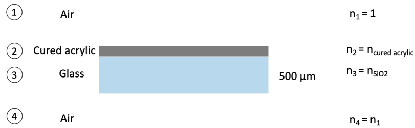
Figure 5.2: Structure of the two layers from the samples.
