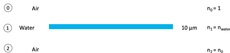
Figure 3.6: Structure of the multilayer.
