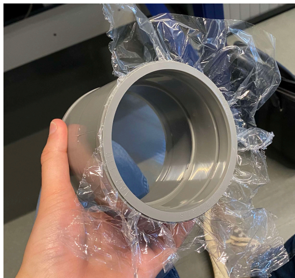
Figure E.3: Step 3: Foil stretched between PVC sleeve and pipe.
