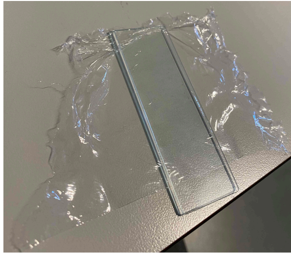
Figure E.2: Step 2: Foil stretched between glass substrates.
