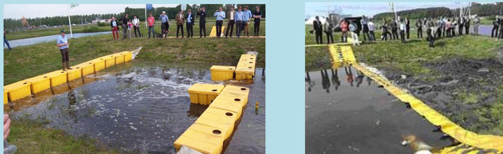
Figure 12: Box barrier (left) and Water gate (right) testing
