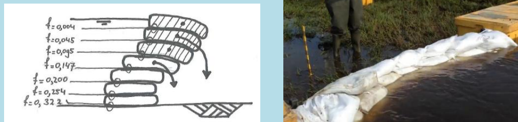
Figure 31: failure of a dike of sand bags (Stoop, 2013)
