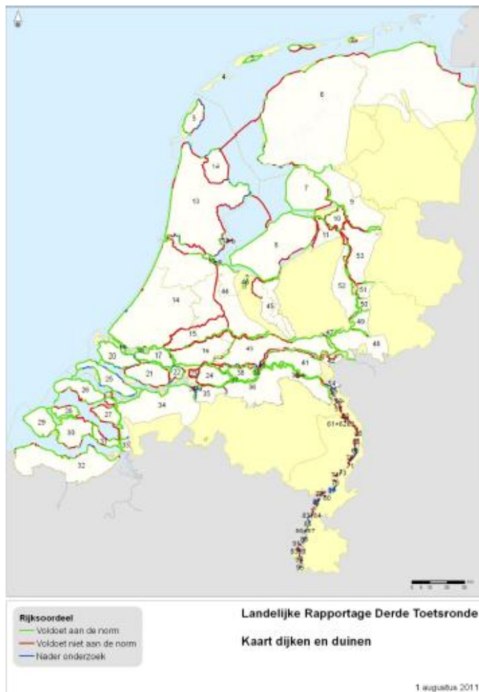
Figure 7: Result of assessment of flood defences [VNK]
