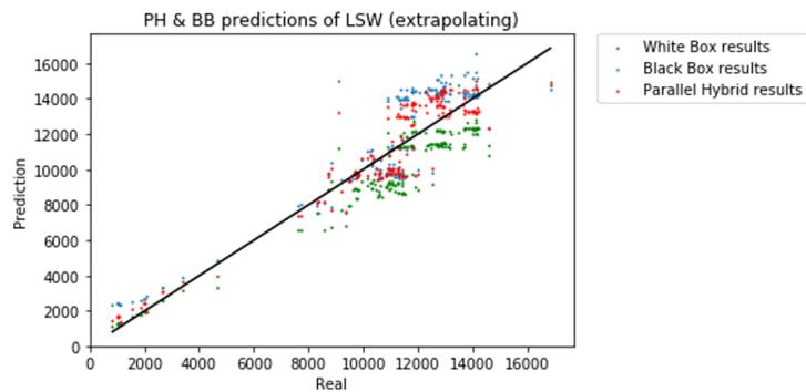
Figure 5.31: Predicting the lightship weight of future ships - Bulk carrier
