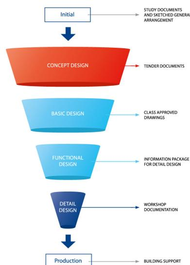
Figure 1.5: Design Phases at C-Job
