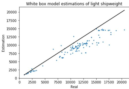
Figure 5.4: White box model results - Oil tanker
