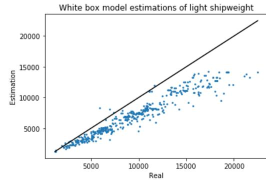
Figure 5.5: White box model results - Container ship
