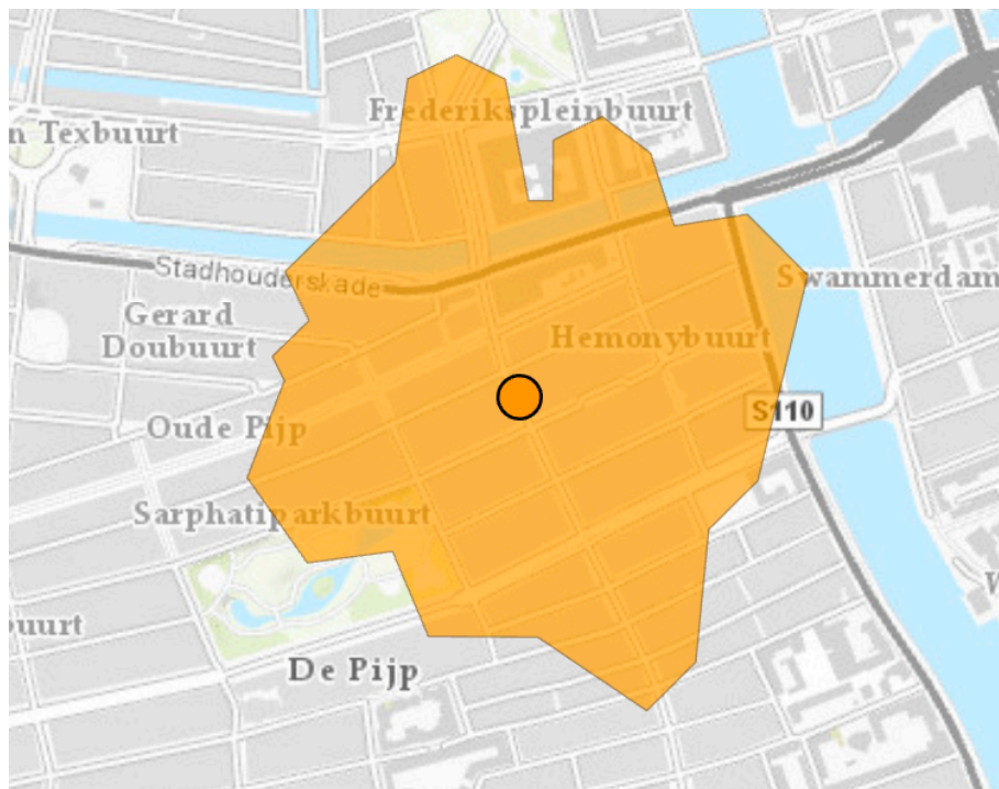
Figure 3.1: A walking coverage buffer area 400m away from a transit stop in Amsterdam, The Netherlands. The buffer is used in the development of supply and demand indicators through GIS analysis
