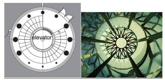
The monumentality of this part is achieved by clustering columns in big tubes which refers to the ancient architecture and express the eternity of monumentality. It functions as the main supporting structure of the building. It also integrated with functions of vertical transport, ventilation ducts and toilets. It imports light for top into the building with patterned window refers also to the ancient architecture.
