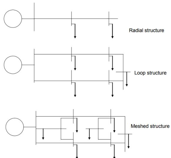
Figure 1.3: Grid topologies: Radial, Loop and Meshed structure
