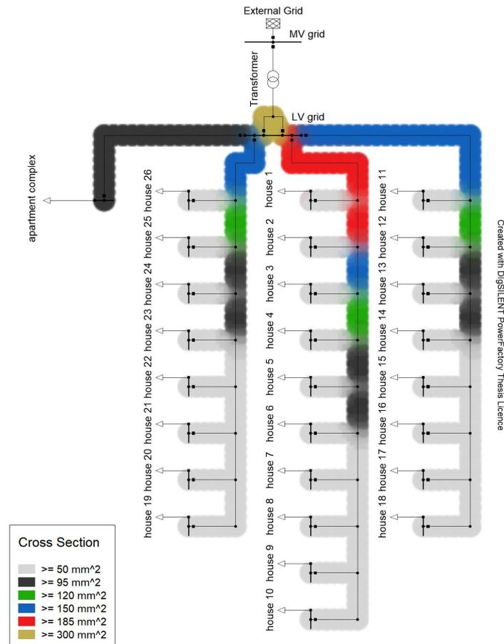
Figure 3.4: Single line diagram with cable cross-sections. Full diagram in Figure A.2.
