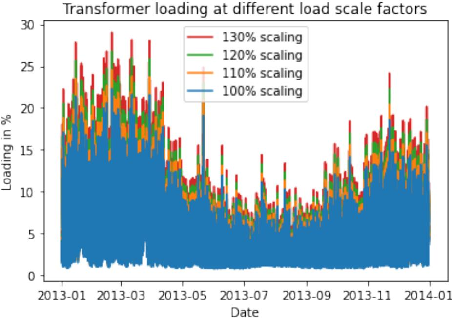
Figure A.7: Transformer loading at different load scale factors.
