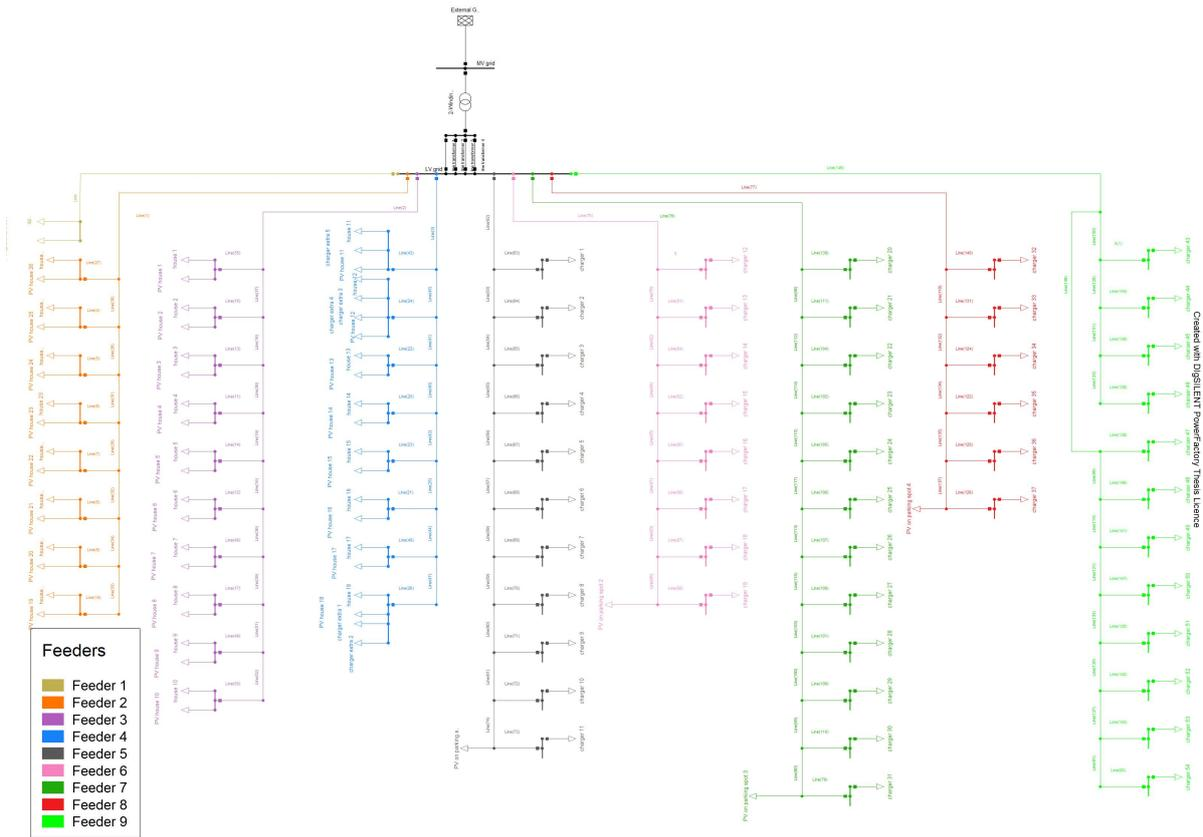
Figure 4.2: Single line diagram with loads, PV and EV charging stations. Full diagram in Figure A.10.
