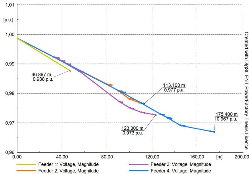
Figure 3.6: Consumer feeder voltage profile. Full diagram in Figure A.6.
