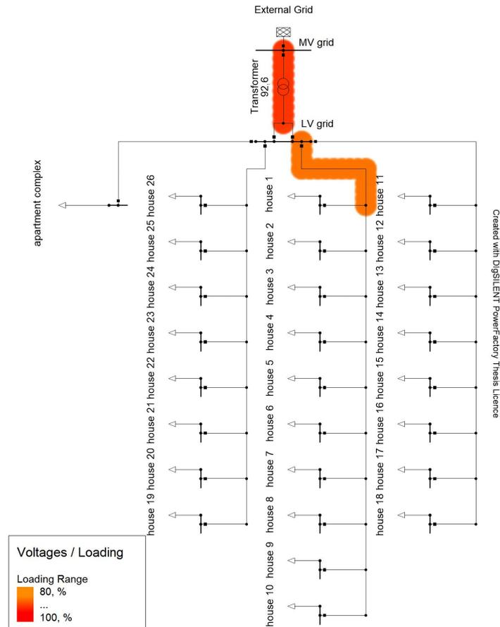
Figure 3.5: Consumer load flow. Full diagram in Figure A.3.
