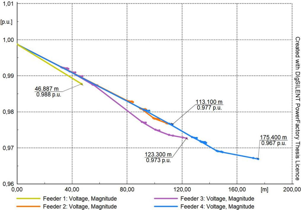
Figure A.6: Consumer feeder voltage profile.
