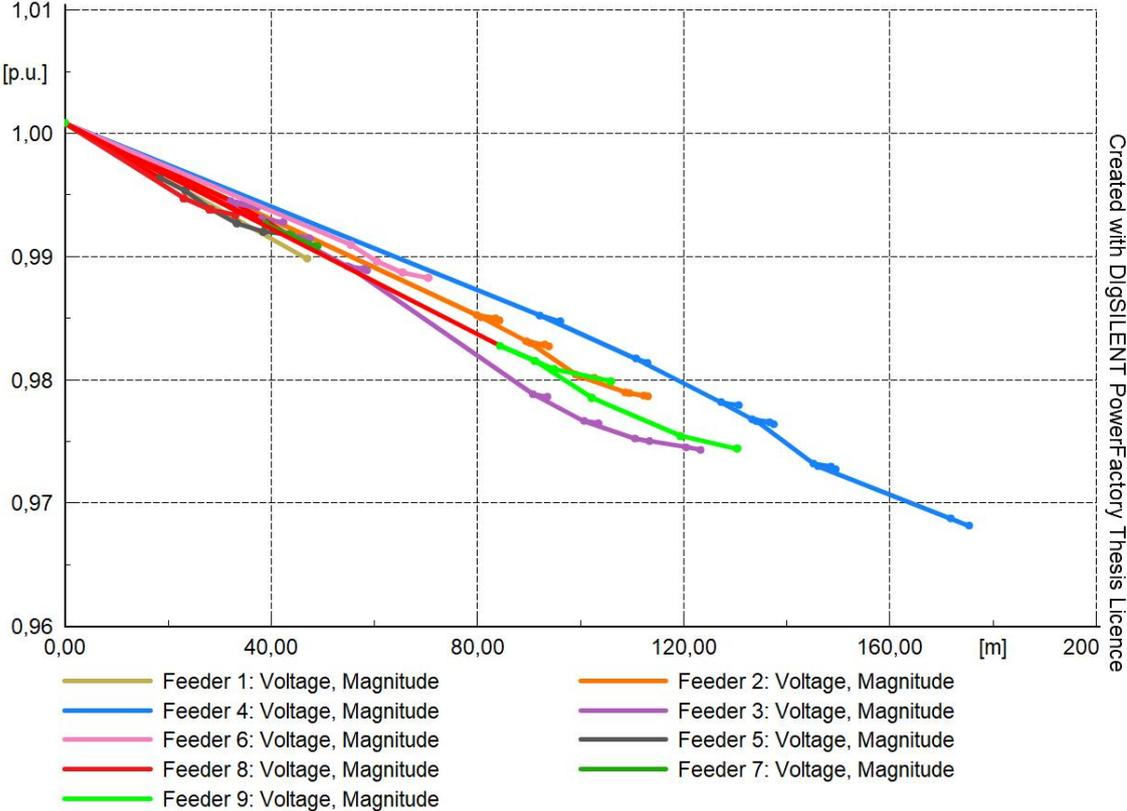
Figure A.15: Voltage profile feeders with loads and EV charging only.
