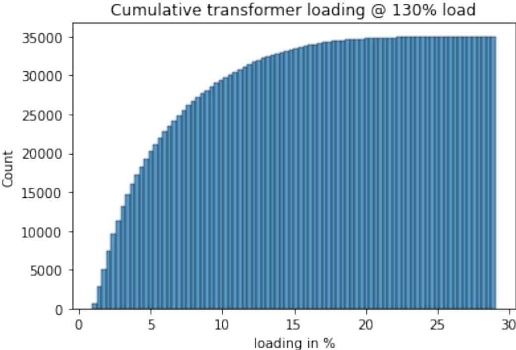
Figure A.8: Cumulative transformer loading at 130% load (year 2048).
