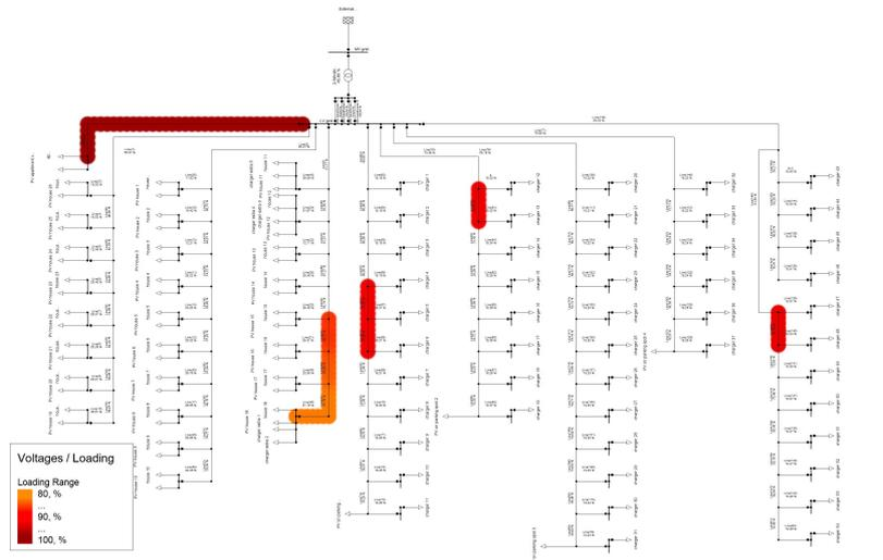
Figure 4.9: Component loading at 270% Load (year 2113). Full diagram in Figure A.17.
