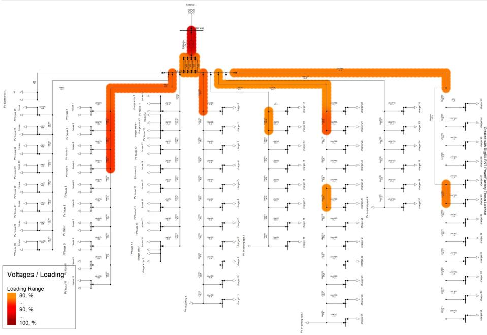
Figure 4.5: Load Flow with loads and EV charging only. Full diagram in Figure A.13.
