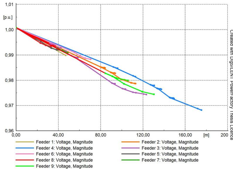
Figure 4.7: Voltage profile for feeders with loads and EV charging only. Full diagram in Figure A.15.
