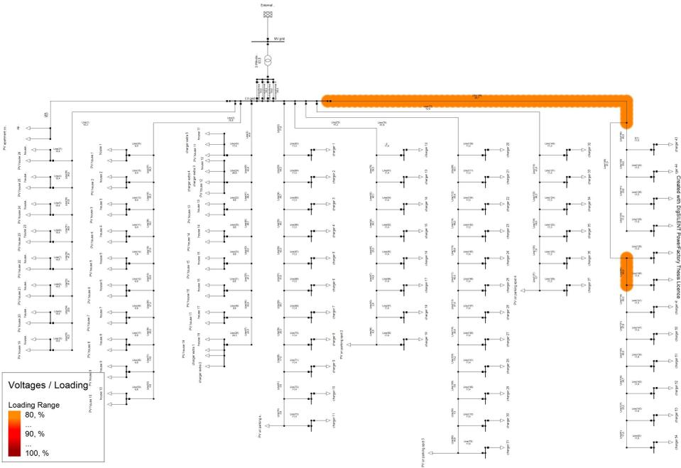
Figure 4.4: Load Flow with loads, PV and EV charging. Full diagram in Figure A.12.
