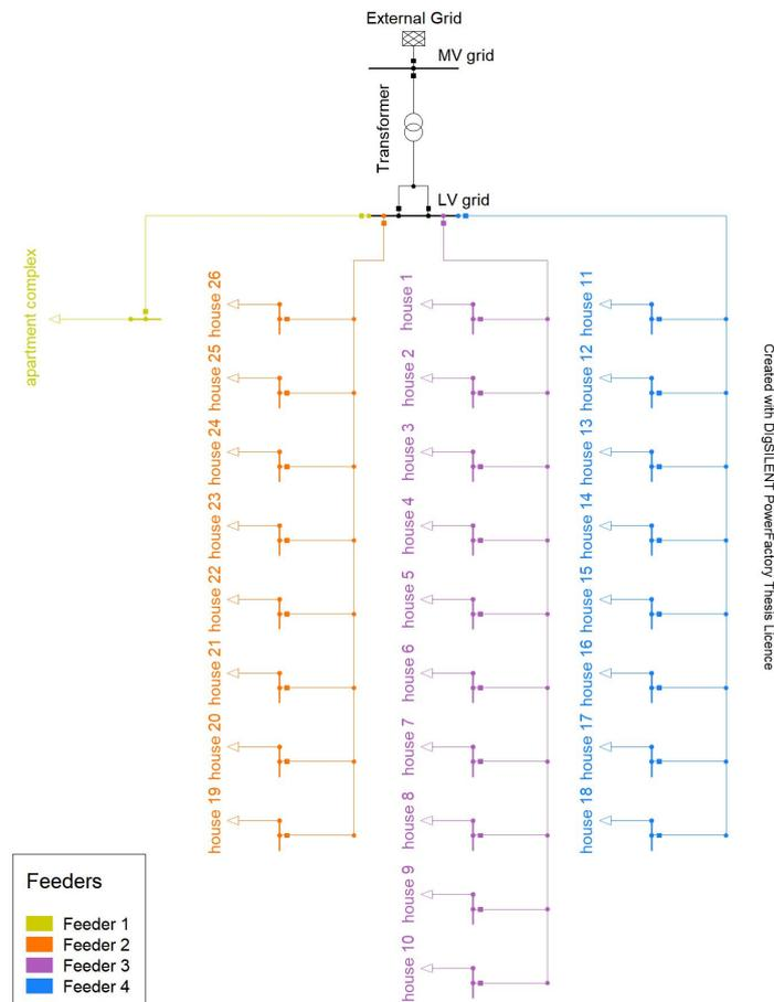
Figure 3.3: The feeder single line diagram. Full diagram in Figure A.1.
