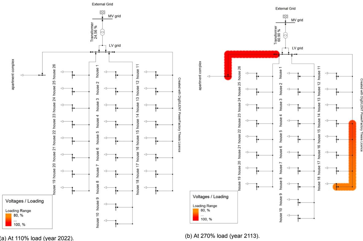
Figure 3.7: Component loading at different load scale factors. Full diagrams in Figure A.4 and Figure A.5 respectively.
