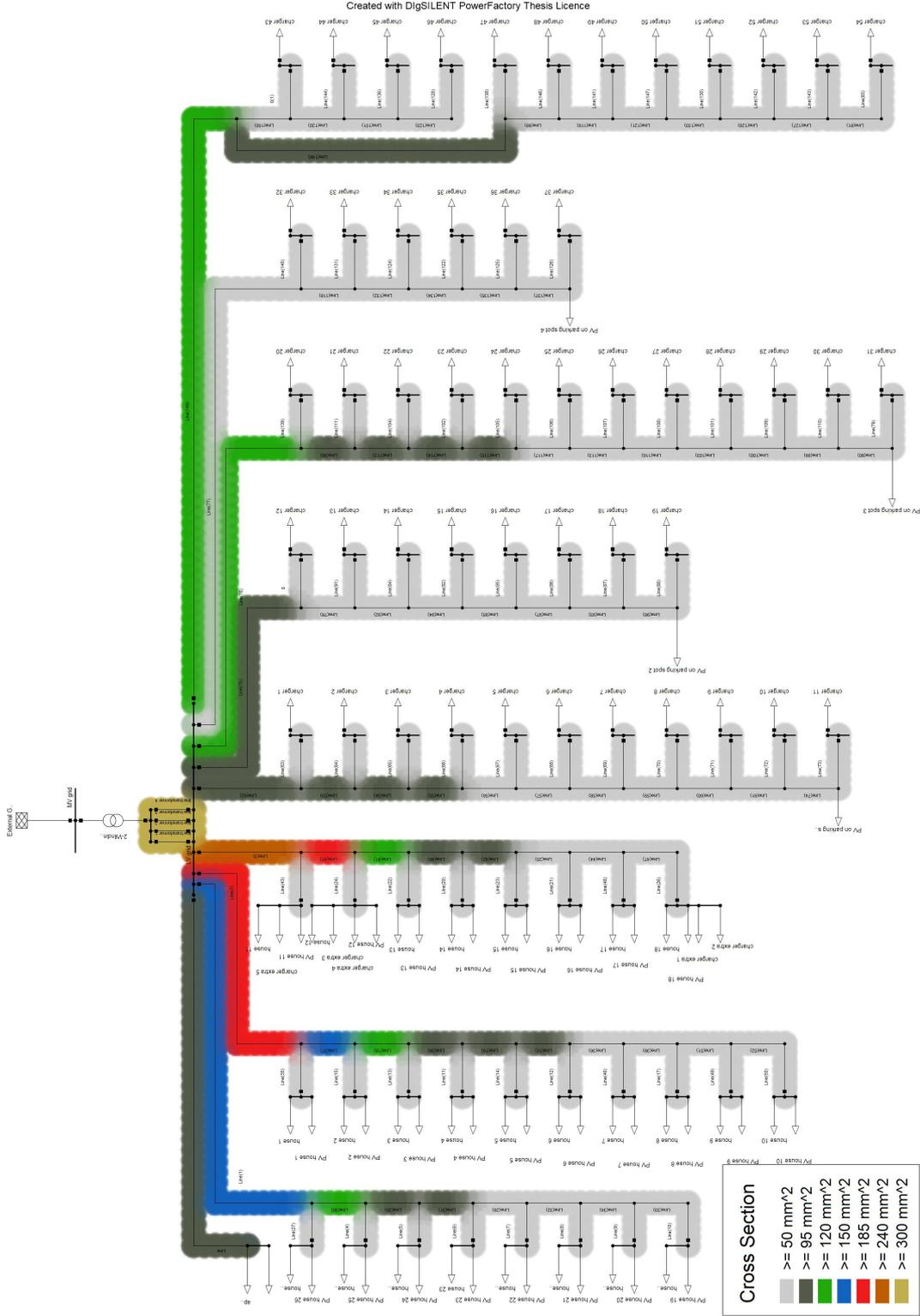
Figure A.11: Single line diagram with cable cross-sections.
