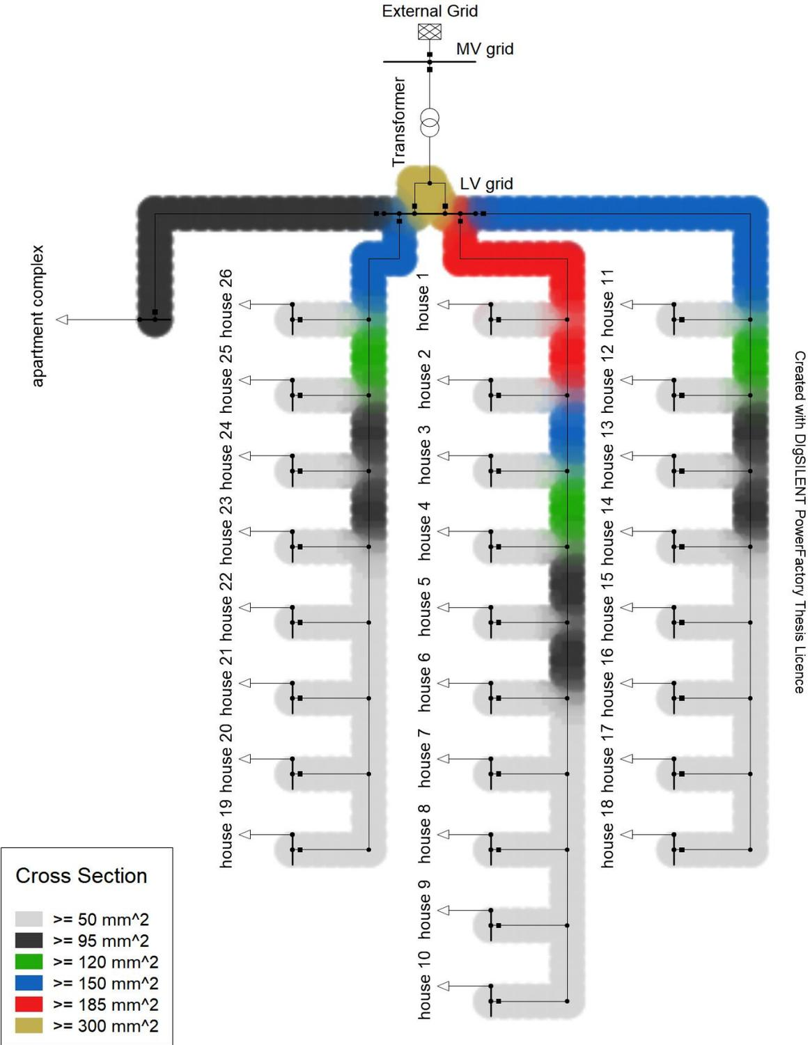
Figure A.2: Single line diagram with cable cross-sections.
