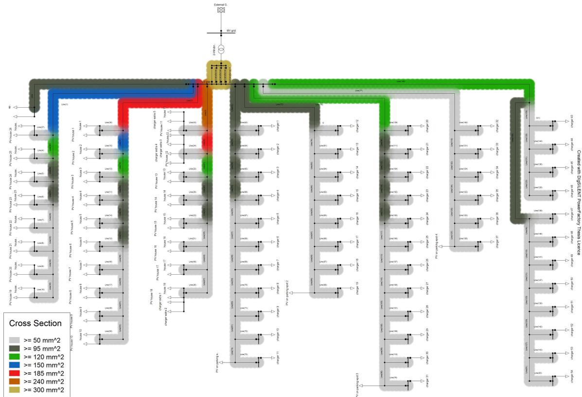
Figure 4.3: Single line diagram with cable cross-sections. Full diagram in Figure A.11.
