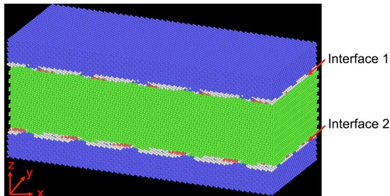
Figure 3-1 The initial, unrelaxed configuration, with periodic conditions in all three directions. Colours represent different crystallographic structures: bcc-blue; fcc-green; unidentified-white, hcp-red. The  $x$  direction in the figure coincides with the fcc  $[\bar{1}\bar{1}2]$  direction,  $y$  with fcc  $[1\bar{1}0]$ , and  $z$  with fcc  $[111]$ .
