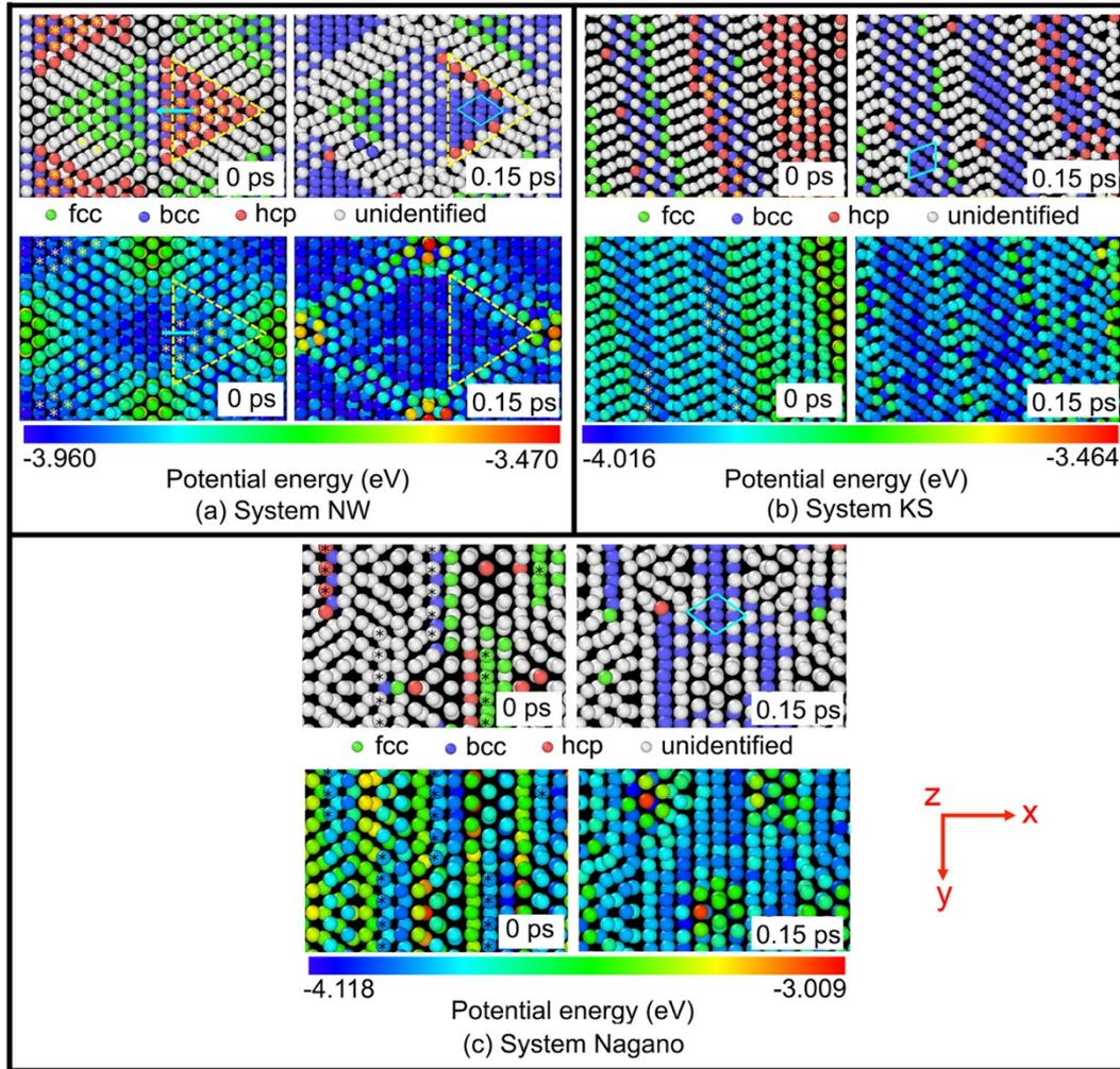
Figure 4-7 (a) Enlarged superposed view of  $(1\ 1\ 1)_{fcc}$  and  $(1\ 1\ 0)_{bcc}$  planes at the interface with NW OR at different simulation times; (b) Enlarged superposed view of  $(1\ 1\ 1)_{fcc}$  and  $(1\ 1\ 0)_{bcc}$  planes at the interface with KS OR at different simulation times; (c) Enlarged superposed view of  $(1\ 1\ \bar{2})_{fcc}$  and  $(1\ 1\ 0)_{bcc}$  planes at the interface in System Nagano at different simulation times.
