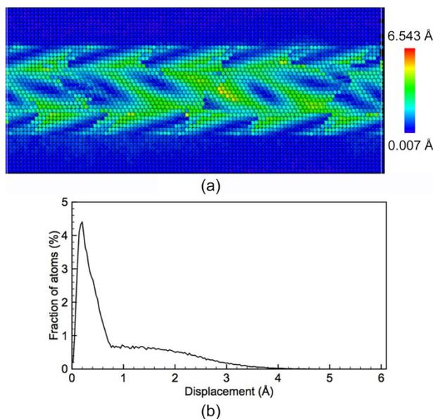
Figure 3-6 (a) View of the  $xz$  plane of the simulation system at 1000 ps with atoms coloured according to their displacements, (b) displacement distribution for atoms in the region between the black and yellow lines in figure 3-6(a).
