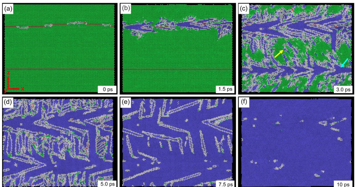
Figure 7-12 Time evolution of the nucleation and growth of bcc phase in fcc iron at 100 K with external strain in the y direction. Colours represent different phase structures: blue-bcc; green-fcc; red-hcp; white-unidentified.
