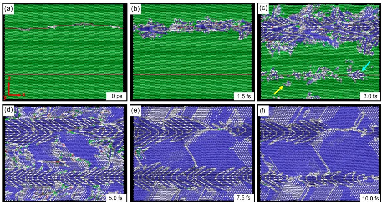
Figure 7-11 Time evolution of the nucleation and growth of bcc phase in fcc iron at 100 K with external strain in the  $x$  direction. Colours represent different phase structures: blue-bcc; green-fcc; red-hcp; white-unidentified.
