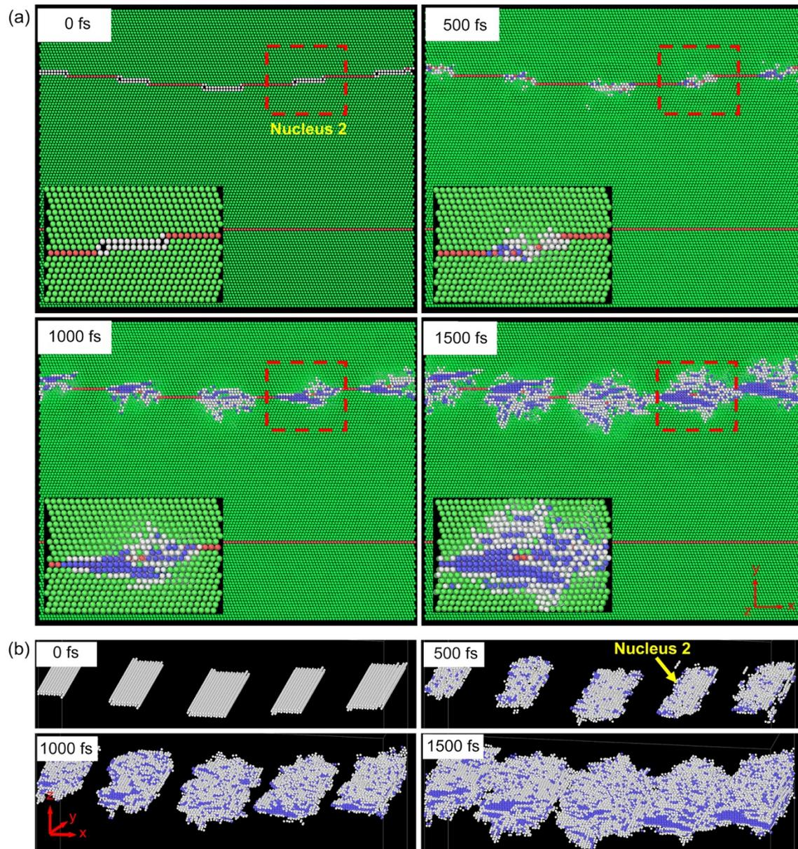
Figure 6-4 (a) Time evolution of the bcc nucleation at the edge dislocations at the STGB at different simulation times; (b) Time evolution of the bcc nucleation at the STGB, the fcc structure is excluded. The inserts in figure (a) are the enlarged views of the corresponding areas marked by the dashed red rectangles. Colours of atoms represent different phase structures: blue-bcc; green-fcc; red-hcp; white-unidentified.
