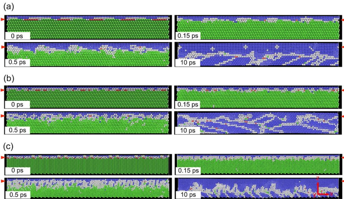
Figure 4-2 Propagation of one of the bcc/fcc interfaces of (a) System NW, (b) System KS and (c) System Nagano, respectively. The position of the original bcc/fcc interface is marked by a red triangle in each configuration.
