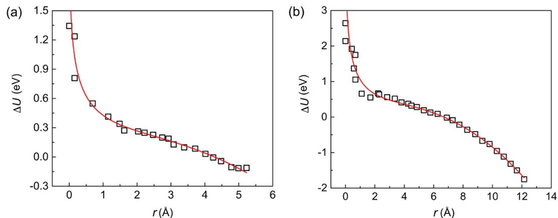
Figure 6-6 The relation between the energy change  $\Delta U$  per unit length along the core of the dislocation and radius  $r$  of the nuclei: (a) Nucleus 1 and (b) Nucleus 2. The black dots are the MD data. The energy change  $\Delta U$  is contributed by the bcc and unidentified structures. The red curves are fitted according to Equation (6-7).
