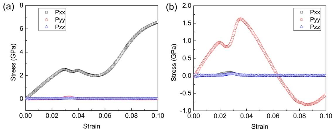
Figure 7-18 The stress-strain curves of Simulation cell 2: (a) with strain in the x direction, (b) with strain in the y direction.
