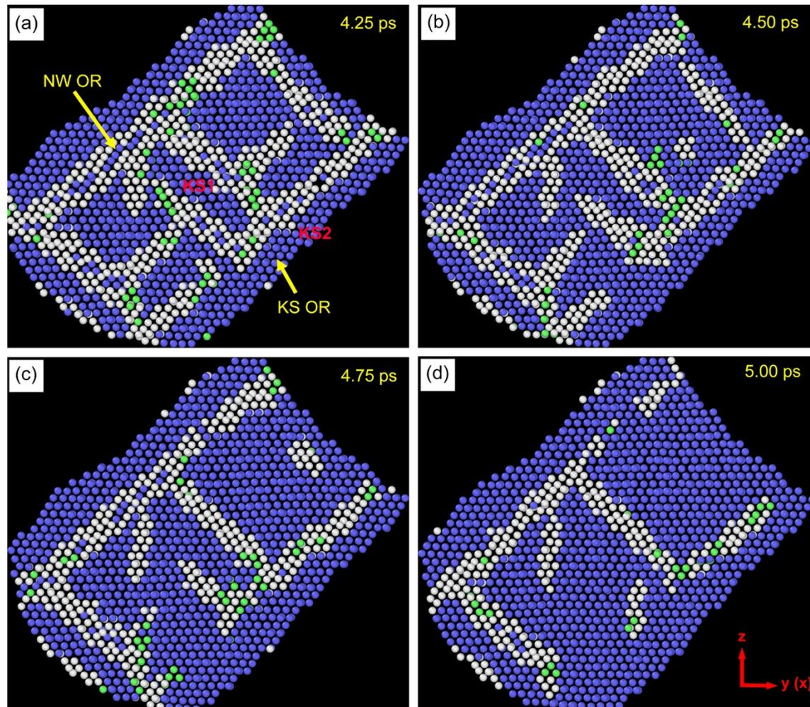
Figure 7-7 Enlarged snapshots of the grain coarsening by coalescence of bcc grains in identical orientation for the simulation cell at 50 K. The view direction is parallel to the  $[1\ \bar{1}\ 0]_{fcc}$  direction. The region in figures (a)-(d) corresponds to the area inside the yellow rectangle in figure 7-2. Colours represent different phase structures: blue-bcc; green-fcc; red-hcp; white-unidentified.
