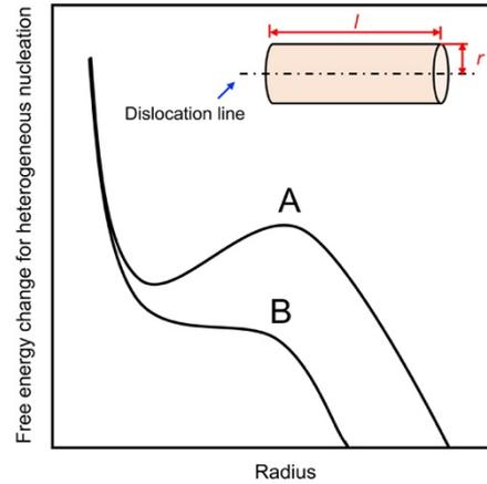
Figure 6-1 Free energy change per unit length of a cylindrical nucleus forming at a dislocation. No local maximum exists with  $\alpha$  greater than 1 (Curve B). A similar figure can be found in Reference [17]. The insert shows the nucleus with a cylindrical morphology,  $r$  and  $l$  represent the radius and the length of the nucleus,  $r \ll l$ .
