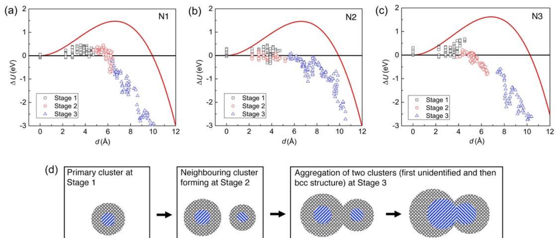
Figure 5-8 The energy  $\Delta U$  as a function of the nucleus size at different stages for nuclei: (a) N1, (b) N2 and (c) N3. (d) Scheme illustrating the three stages in figures (a)-(c). The energy  $\Delta U$  involves in both the bcc and unidentified structures, which correspond to the blue and grey regions in figure (d). The energy  $\Delta U$  at Stage 1 and 2 is only contributed by the primary cluster while that at Stage 3 is contributed by the aggregate.
