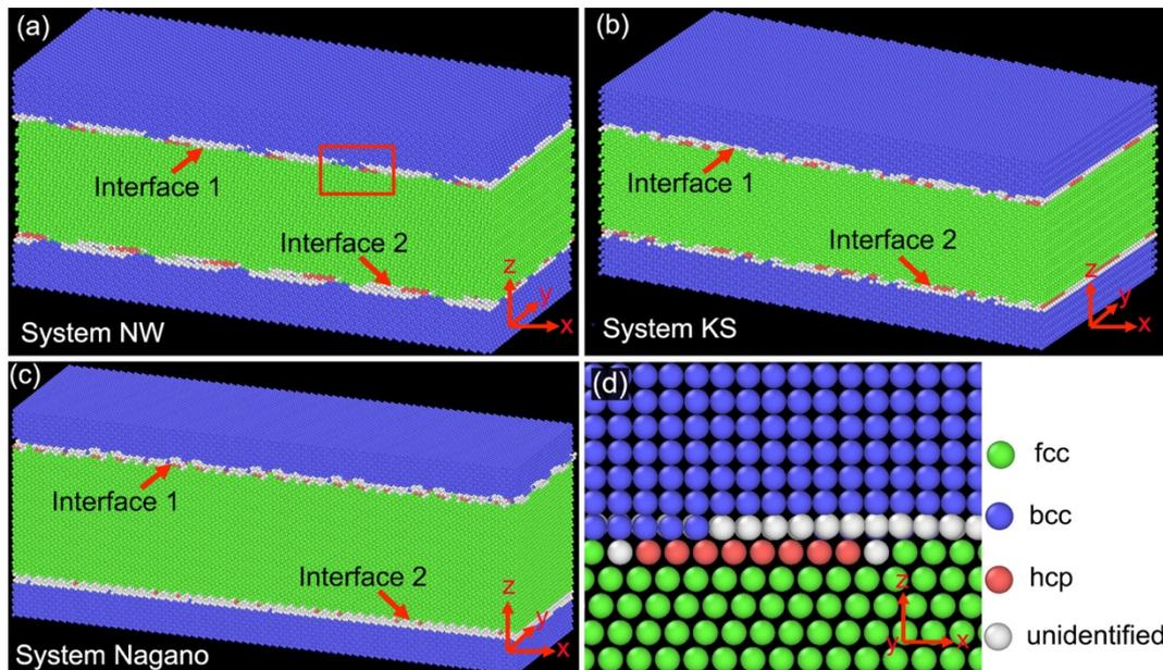
Figure 4-1 The initial, relaxed configurations of (a) System NW, (b) System KS and (c) System Nagano. (d) represents the enlarged region as inside the red rectangle in figure (a). Colours represent different phase structures: blue-bcc; green-fcc; red-hcp; white-unidentified.
