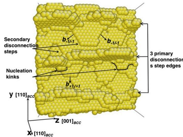
Figure 2-8 Cross-sectional view normal to the interface  $(1\ 1\ 0)_{bcc}$  during the transformation with only the bcc atoms indicated. Islands of the bcc nucleate on the edge of the primary disconnection steps and several secondary disconnections grow along their Burgers vectors direction in each terrace plane. Only bcc atoms are shown. [45]
