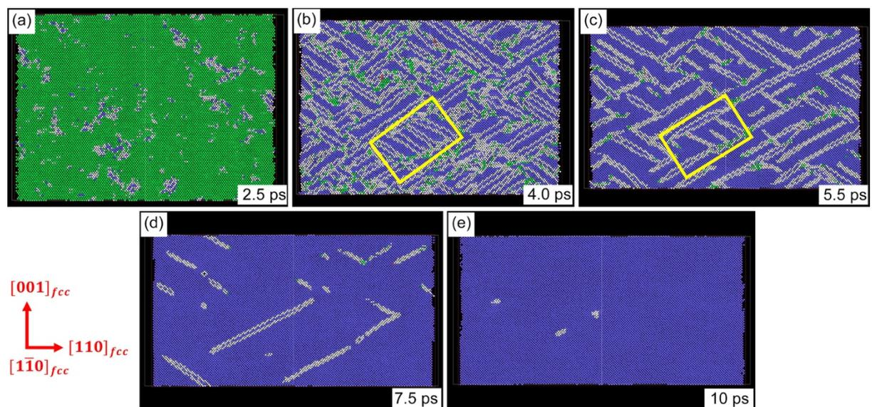
Figure 7-3 Time evolution of the structure in a slice of 3.5 Å in the  $[1 \bar{1} 0]_{fcc}$  direction indicating the fcc-to-bcc transformation in fcc iron under strain at 100 K. Colours represent different phase structures: blue-bcc; green-fcc; red-hcp; white-unidentified.
