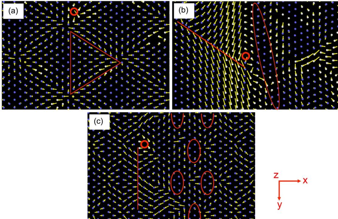
Figure 4-9 Snapshots of atoms with 3-dimensional displacement vectors for System NW (a), System KS (b) and System Nagano (c). The local regions involved in (a)-(c) belong to the mono fcc-plane at the interfaces and the corresponding displacements are calculated at 10 ps.
