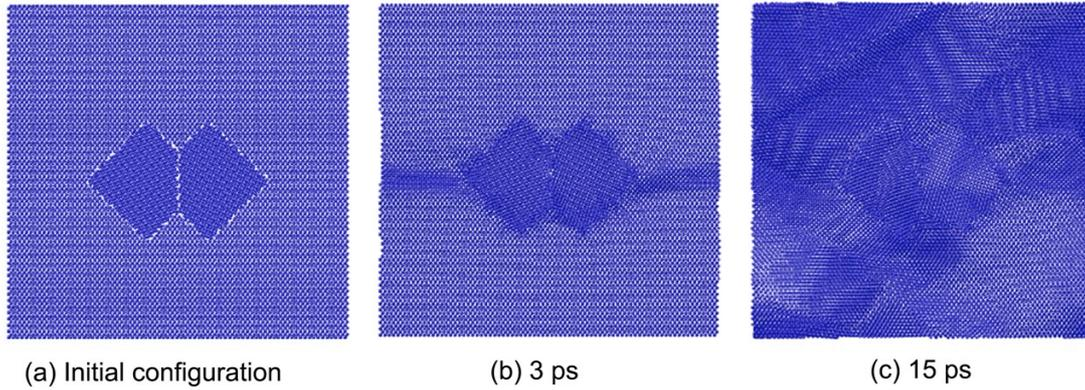
Figure 2-2 Cross-sectional view through the simulation crystallite containing a grain boundary at the beginning of the simulation, and at two times during the transformation at 0 K: (a) initial fully fcc configuration, (b) the fcc-to-bcc transformation initiating from the grain boundaries at 3 ps, (c) the final heterogeneous structure resulting from the fcc-to-bcc transformation at 15 ps [28].
