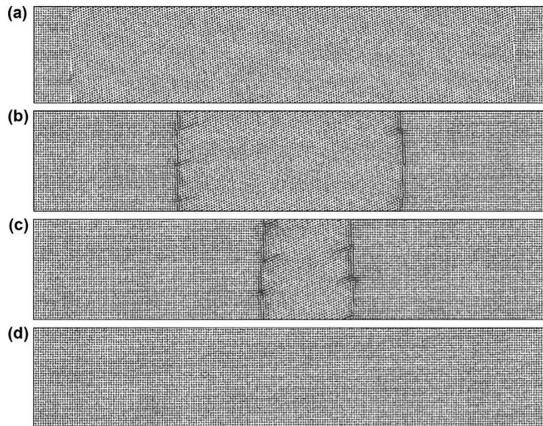
Figure 2-7 An example of the fcc-to-bcc transformation process for a temperature of 800 K. (a) The initial state of the simulation box shows a sandwich structure, with two bcc phases connecting the two sides of a fcc phase. (b and c) The positions of the interfaces at 5 and 10 ns. (d) The equilibrium bcc phase after the transformation. [44]
