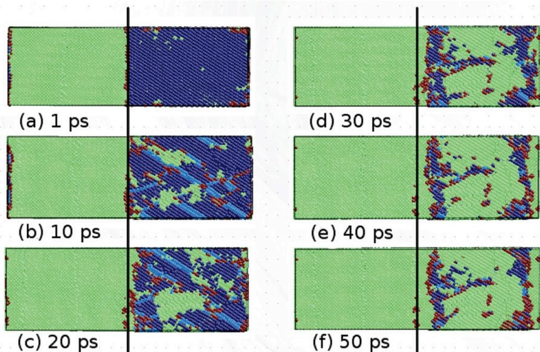
Figure 2-6 Snapshots showing the time evolution of the fcc-to-bcc transition (NW interface) at 100 K. The original position of the interface has been marked by a black line. Colours represent different crystallographic structures: green-bcc, dark blue-fcc, light blue-hcp, red-unknown. [42]
