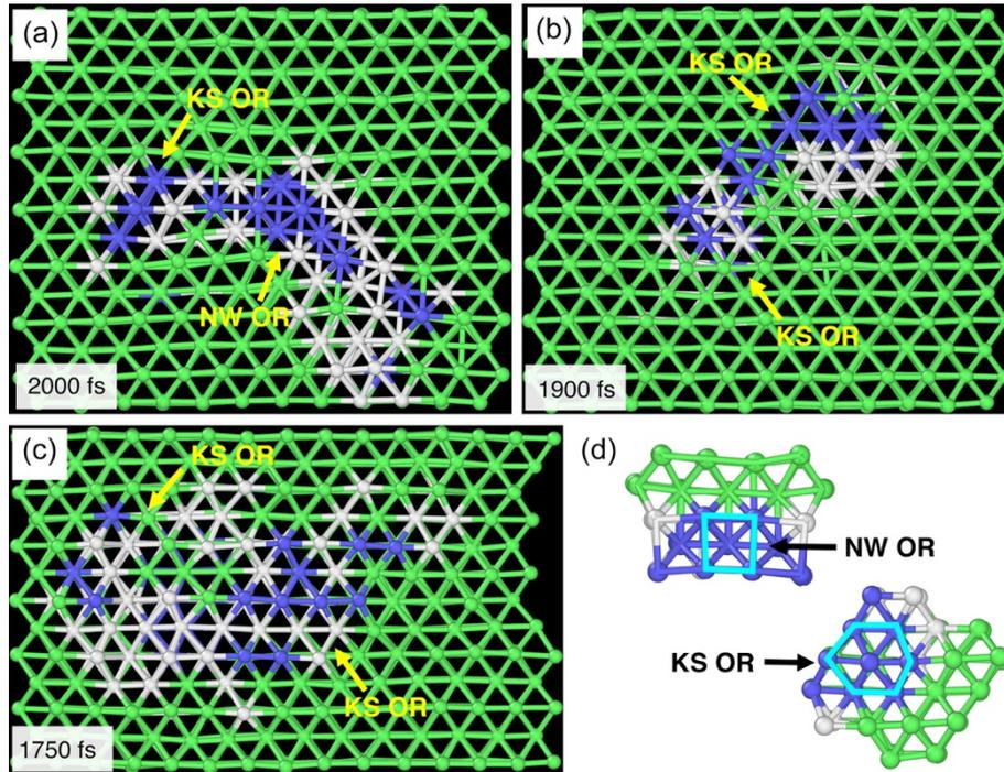
Figure 5-6 The orientation of the aggregated clusters for: (a) N1, (b) N2 and (c) N3. The view direction is parallel to  $[1\bar{1}0]_{fcc}$ . Bonds are created between atoms within the cutoff distance of 3.2 Å. Illustration of the NW and KS OR are highlighted in light blue in figure (d). Colours of atoms represent different phase structures: blue-bcc; green-fcc; white-unidentified.
