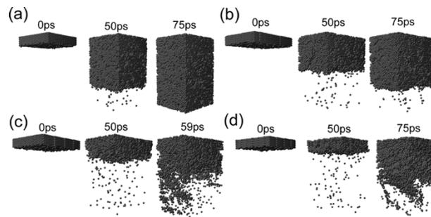
Figure 2-5 Snapshots of the calculation cell with the interface of (a) NW OR, (b) the intermediate OR with a rotation angle of  $2.00^\circ$  from NW, (c) the intermediate OR with a rotation angle of  $4.00^\circ$  from NW OR and (d) KS OR during relaxation. Only atoms with bcc configuration are shown in (a)-(d) for clarity. [38]
