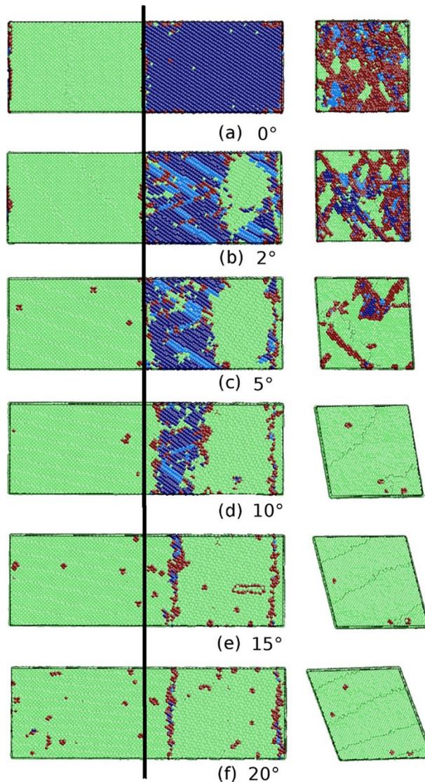
Figure 2-11 Snapshots showing the local structure of the fcc-bcc biphasic system at a temperature of 300 K for shear angles of up to 20°. The pictures on the left show the phase evolution in the  $y$ - $z$  plane; those on the right show the original interface plane ( $x$ - $z$  plane) in the middle of the system. The colors denote the local crystal structure. Green: bcc; dark blue: fcc; light blue: hcp; red: unknown. The original interface position is marked by a black line. [43]
