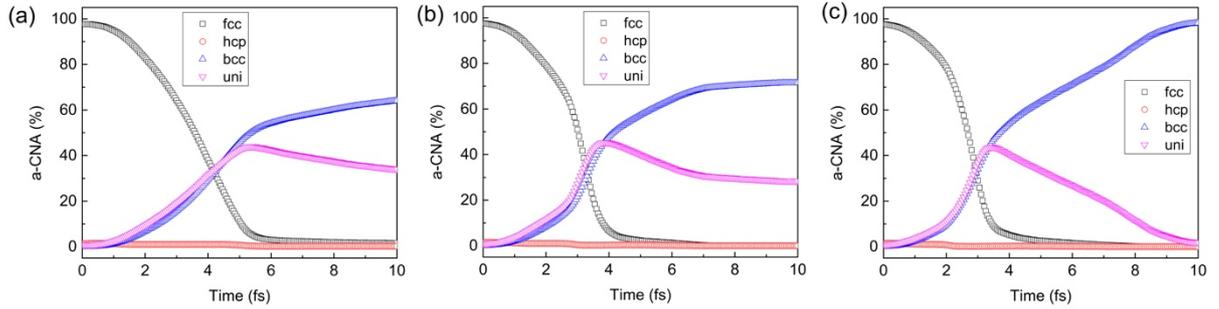
Figure 7-13 The phase fractions of Simulation cell 2: (a) without external strain, (b) with strain in the x direction, (c) with strain in the y direction.
