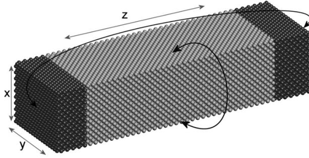
Figure 2-4 A typical starting configuration for interface type C, a system with only one nonperiodic direction (the  $y$  direction). Bcc atoms are dark; fcc atoms are light. The  $x$  direction in the figure coincides with the  $[1\ 0\ 0]_{fcc}$  direction,  $y$  with  $[0\ 1\ 0]_{fcc}$ , and  $z$  with  $[0\ 0\ 1]_{fcc}$ . [6]
