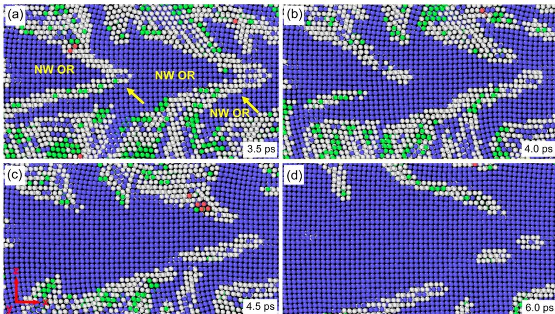
Figure 7-17 Grain coarsening by coalescence of neighbouring bcc grains with the identical orientation in the simulation cell under strain in the  $y$  direction.
