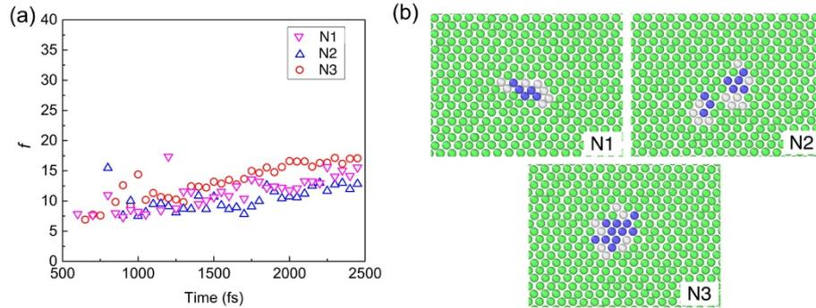
Figure 5-4 (a) Shape parameter  $f$  of nuclei N1-N3; (b) Monolayer of the  $(1 \bar{1} 0)_{fcc}$  plane indicating the lattice matching between the bcc and fcc phases for N1 (1550 fs), N2 (1800 fs) and N3 (1250 fs), respectively. Colours of atoms represent different phase structures: blue-bcc; green-fcc; white-unidentified.
