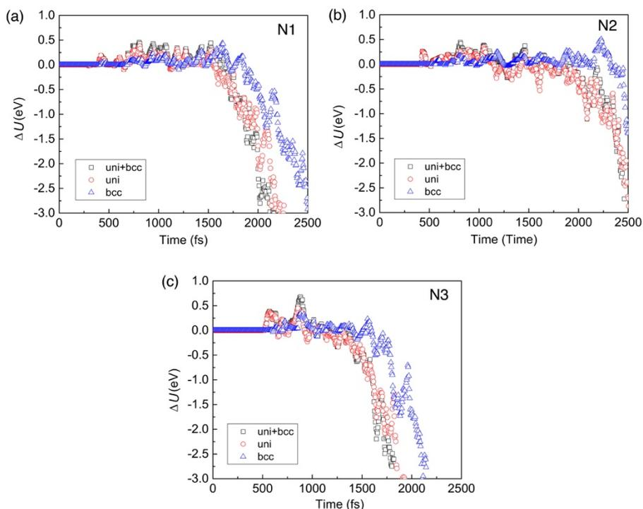
Figure 5-11 Contributions of the bcc and unidentified structures to the energy change of the bcc nucleus as a function of simulation time: (a) N1, (b) N2 and (c) N3. The labels “uni” and “bcc” in (a)-(c) represent unidentified and bcc structures.
