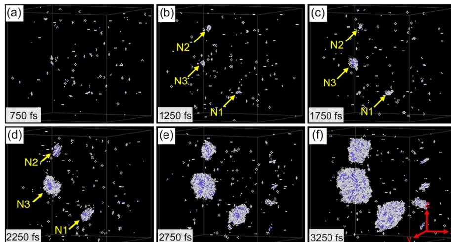
Figure 5-2 Configurations of bcc nucleation at 160 K. Colours of atoms represent phase structures: blue-bcc; white-unidentified. Atoms in the fcc structure are not displayed.
