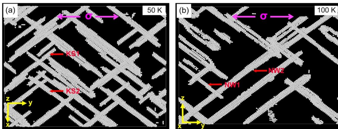
Figure 7-9 (a) Snapshot of the simulation cell at 50 K at 6.5 ps; (b) Snapshot of the simulation cell at 100 K at 9.0 ps. In figures (a) and (b), only the unidentified atoms acting as the grain boundaries are displayed.
