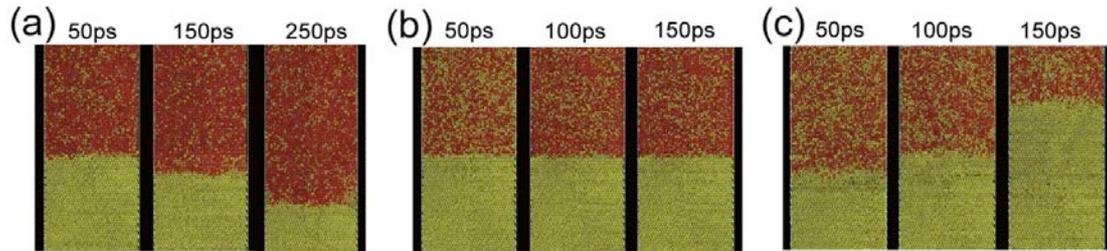
Figure 2-9 Snapshots of the fcc-bcc configuration with the NW orientation relationship during relaxation at various temperatures: (a) 1511 K (below A3 temperature of the ‘Finnis-Sinclair’ potential), (b) 1516 K (the A3 temperature) and (c) 1521 K (above the A3 temperature). Brown and yellow spheres represent atoms with the bcc and fcc configurations, respectively. [27]
