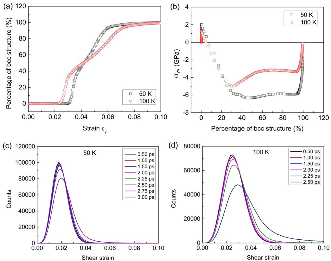
Figure 7-5 The fraction of bcc phase as a function of the external strain  $\epsilon_y$  at 50 K and 100 K; (b) The stress in the y direction  $\sigma_{yy}$  as a function of the fraction of bcc phase at 50 K and 100 K; (c) Histogram of shear strain of atoms
