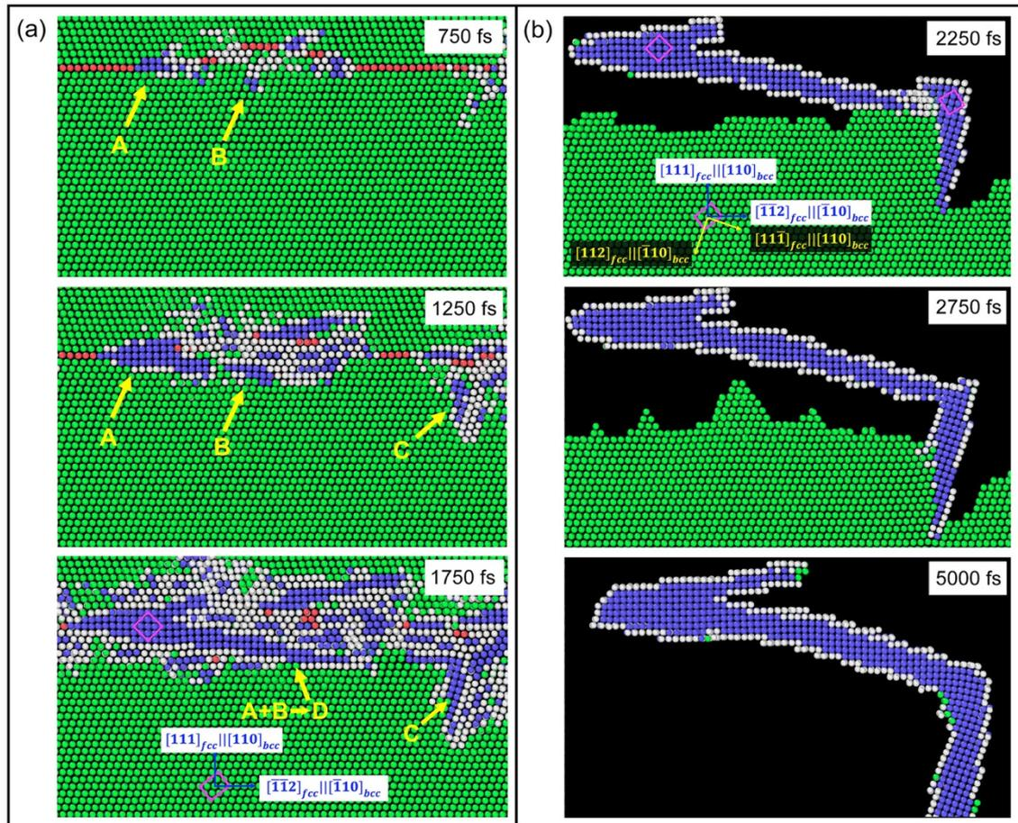
Figure 7-14 Snapshots showing the impingement of bcc grains: (a) in the NW OR forming from the same variant; (b) in the NW OR forming from different variants. The simulation cell is under no external strain. Only the two bcc grains that merge are included in figure (b), while the other bcc grains are excluded for a better view of the merging process.
