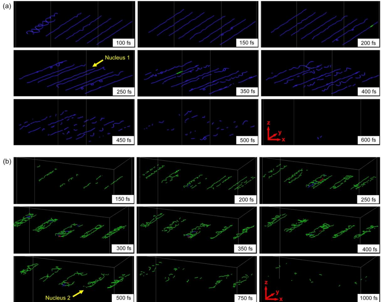
Figure 6-5 Time evolution of the dislocation lines at: (a) LAGB 2, (b) STGB, respectively. Colours of the dislocation lines represent different dislocation types: blue -  $\frac{1}{2} \langle 110 \rangle$ ; green -  $\frac{1}{6} \langle 112 \rangle$ ; red - other.
