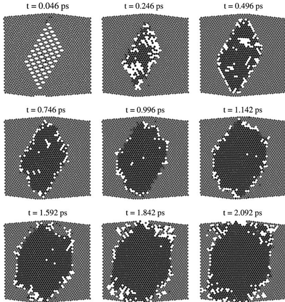
Figure 2-3 Graphical illustration of simulation cell (viewed along the  $[0\ 1\ 1]_{fcc}$  direction) as a function of relaxation time (given above each image) showing the gradual formation of a structure with 8-coordinated atoms (dark gray) first within the intersection volume followed by growth into the fault bands and unfaulted fcc matrix.
