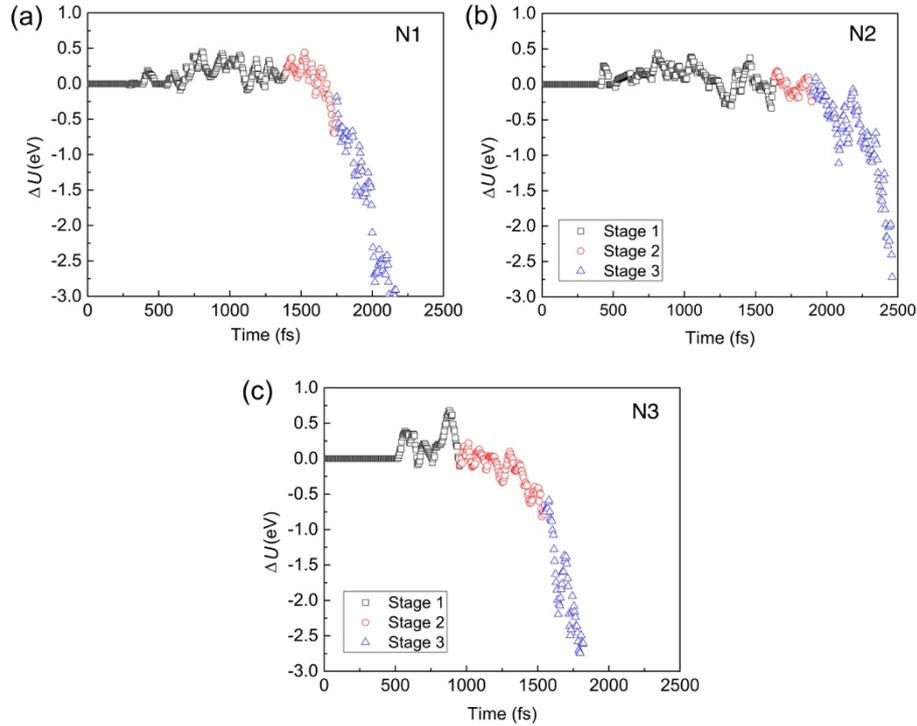
Figure 5-9 The energy change in Stage 1 to 3 as a function of time for the bcc nucleus: (a) N1, (b) N2 and (c) N3. The energy change is contributed by atoms both in the bcc and unidentified structure. The dots with energy change smaller than -3.0 eV are excluded.
