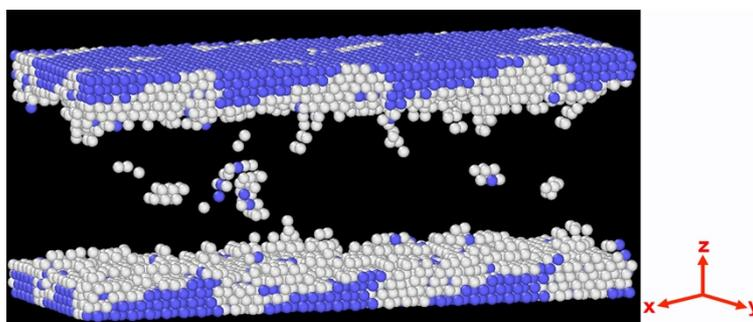
Figure 3-5 Three-dimensional snapshot of the volume shown in figure 3-4 at 0.50 ps. All the fcc and hcp phases were deleted leaving only the bcc phase and unknown phase. The colours denote the local crystal structure as in figure 3-1.
