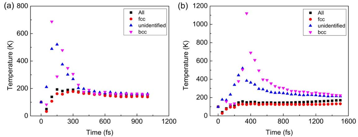
Figure 6-10 (a) Temperature of different structures in the selected volume for Nucleus 1; (b) Temperature of different structures in the selected volume for Nucleus 2.
