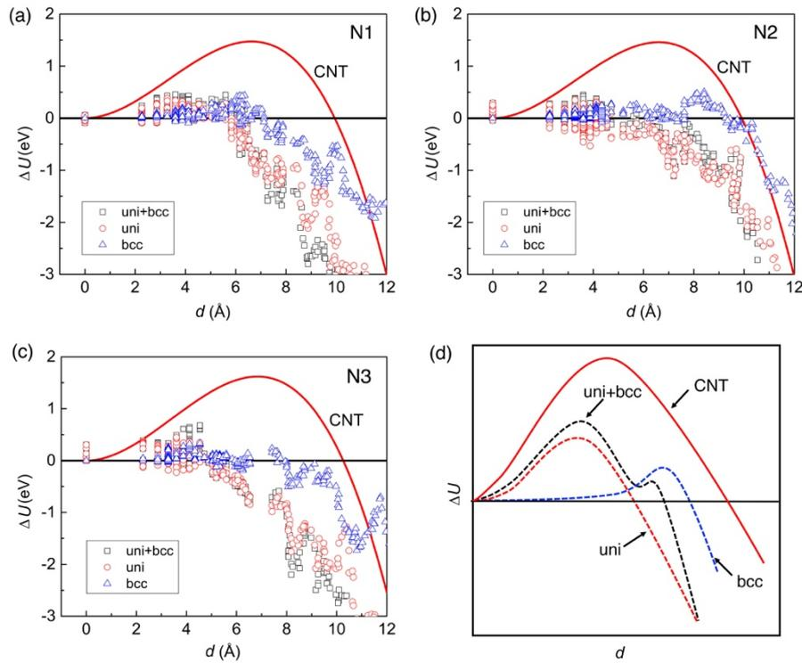
Figure 5-10 Contributions of the bcc (blue triangles) and unidentified (red circles) structures to the energy change of the bcc nuclei (black squares) as a function of the nucleus size: (a) N1, (b) N2 and (c) N3. The solid red curves in figures (a)-(c) show the prediction by the CNT. (d) Schematic picture of the energy  $\Delta U$  in (a)-(c). The labels “uni” and “bcc” in (a)-(d) represent unidentified and bcc structures.
