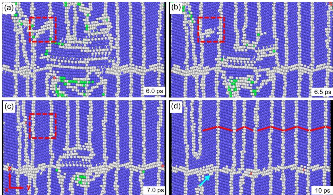
Figure 7-16 Snapshots illustrating the grain coarsening by coalesce of neighbouring bcc grains as well the twinning structures in simulation cell under strain in the  $x$  direction.
