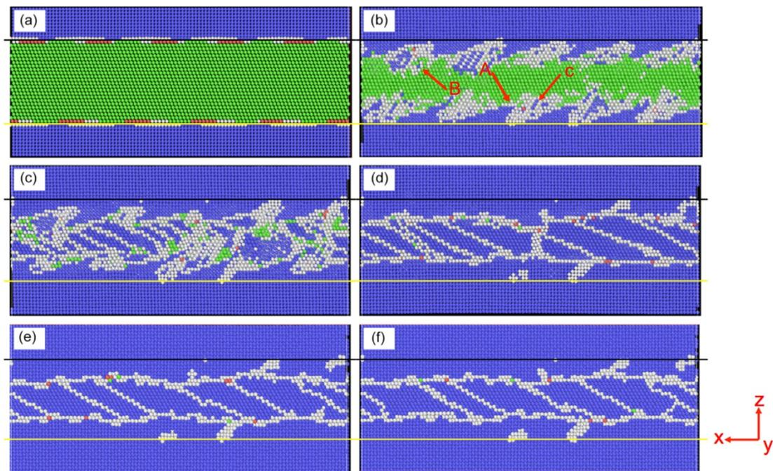
Figure 3-2 Snapshots showing the time evolution of the fcc-bcc transition: (a) 0 ps, (b) 1 ps, (c) 2.5 ps, (d) 10 ps, (e) 100 ps, (f) 1000 ps. The original positions of the interface 1 and 2 are marked by a black line and a yellow line, respectively. The colours denote the local crystal structure as in figure 3-1.
