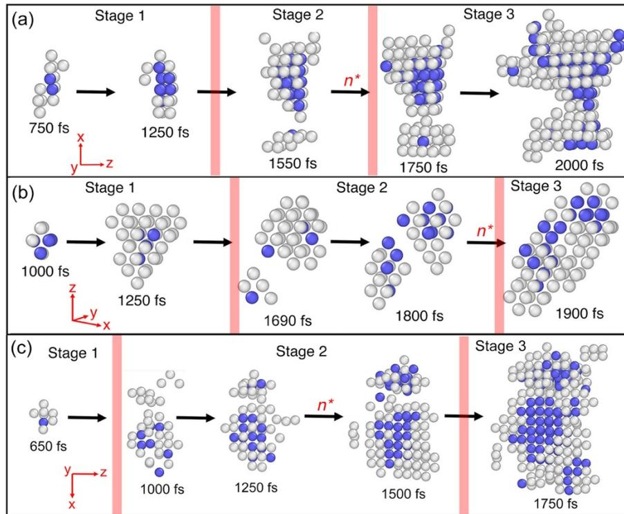
Figure 5-5 Nucleation process by aggregation of neighbouring clusters: (a) N1, (b) N2 and (c) N3.  $n^*$  represents the occurrence of the critical nucleus size. Colours of atoms represent different phase structures: blue-bcc; white-unidentified. Atoms in the fcc structure are excluded in figures (a) to (c).
