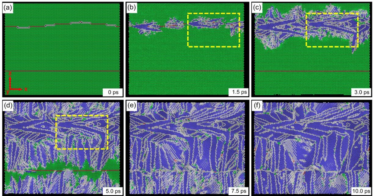
Figure 7-10 Time evolution of the nucleation and growth of bcc phase in fcc iron at 100 K without external strain.
