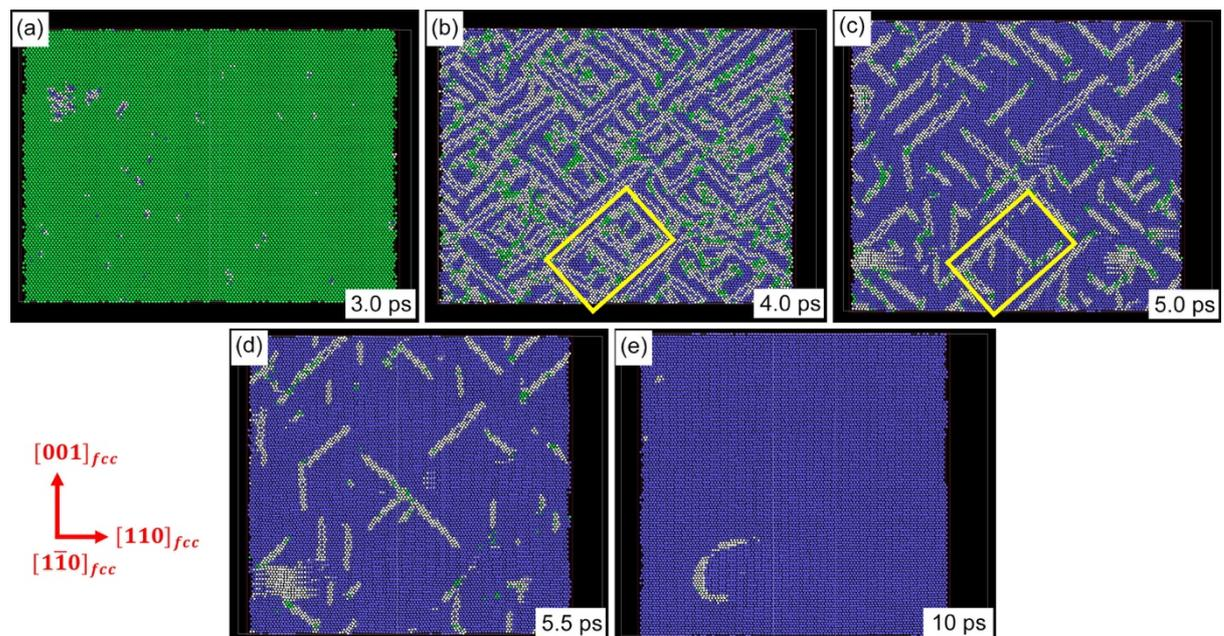
Figure 7-2 Time evolution of the structure in a slice of 3.5 Å in the  $[1 \bar{1} 0]_{fcc}$  direction indicating the fcc-to-bcc transformation in fcc iron under strain at 50 K. Colours represent different phase structures: blue-bcc; green-fcc; red-hcp; white-unidentified.
