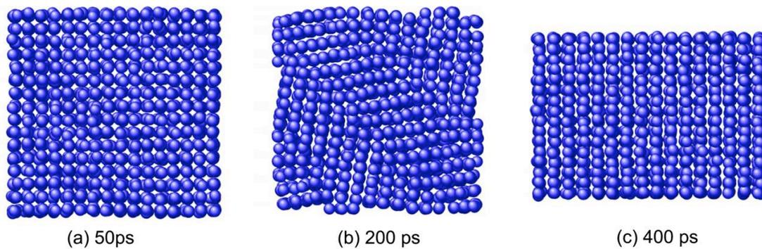
Figure 2-1 Cross-sectional view through the transforming crystallite ( $T=1400$  K) at various stages of the transformation process: (a) the initial fcc crystal at 50 ps; (b) the transformed bcc phase with twin structure; (c) the twin structure diminished in the final bcc grain [28].
