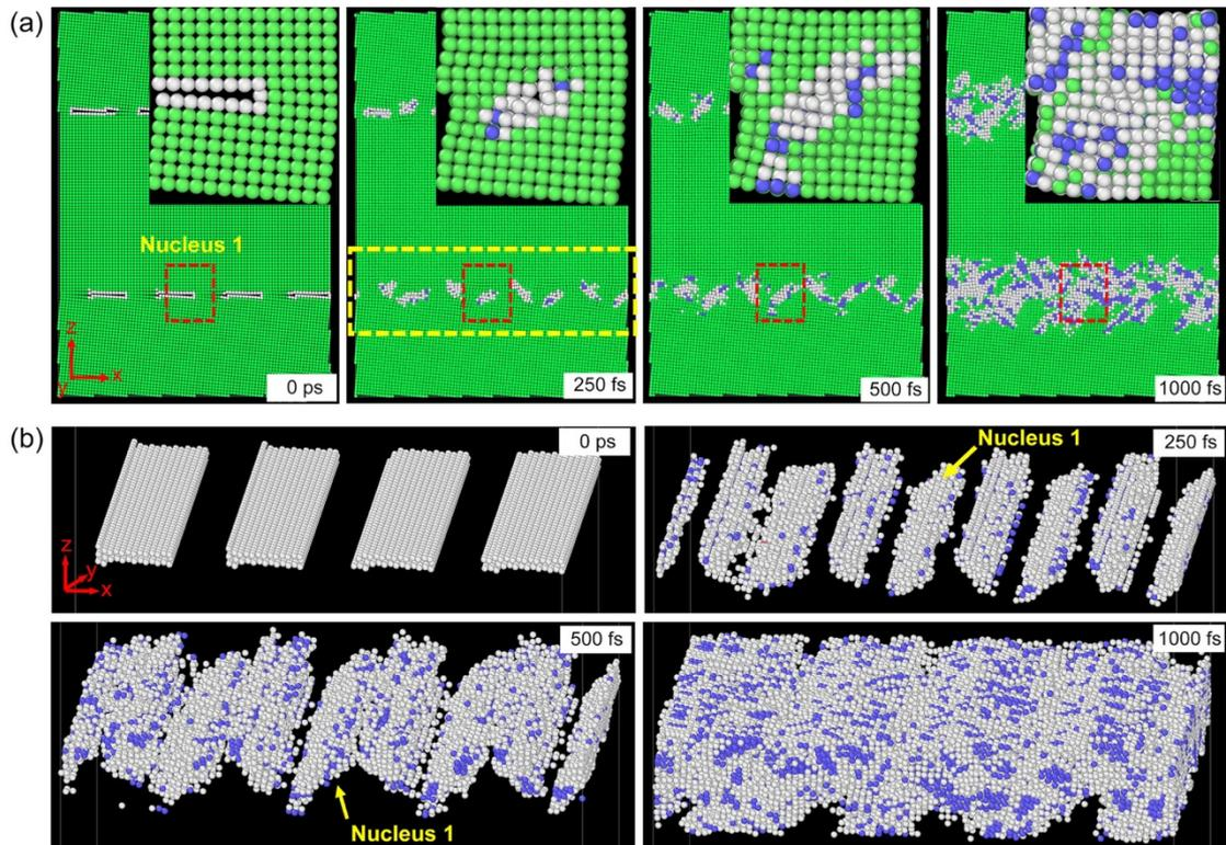
Figure 6-3 (a) Time evolution of the bcc nucleation at the edge dislocations at the LAGB at 0 fs, 250 fs, 500 fs and 1000 fs; (b) Time evolution of the bcc nucleation at the LAGB 2, as marked by the yellow dashed rectangle in figure (a), the fcc phase is excluded. Enlarged views of the regions marked by the dashed red rectangle are inserted in figure (a). Colours of atoms represent different phase structures: blue-bcc; green-fcc; red-hcp; white-unidentified.
