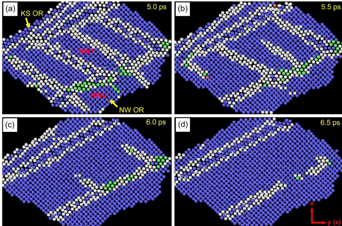
Figure 7-8 Enlarged snapshots of the grain coarsening by coalescence of bcc grains in identical orientation for the simulation cell at 100 K. The view direction is parallel to the  $[1\ \bar{1}\ 0]_{fcc}$  direction. The region in figures (a)-(d) corresponds to the area inside the yellow rectangle in figure 7-3. Colours represent different phase structures: blue-bcc; green-fcc; red-hcp; white-unidentified.
