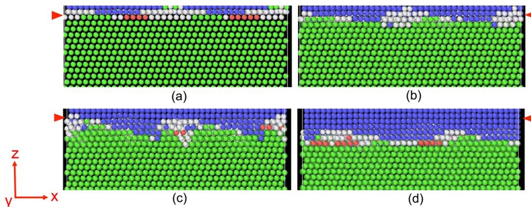
Figure 4-3 Propagation of one of the bcc/fcc interfaces in the NW OR in iron using the Ackland Potential [22] at different simulation times: (a) 0 ps; (b) 0.15 ps; (c) 0.5 ps and (d) 10 ps. The position of the original bcc/fcc interface is marked by a red triangle in each configuration. Colours represent different phase structures: blue-bcc; green-fcc; red-hcp; white-unidentified.
