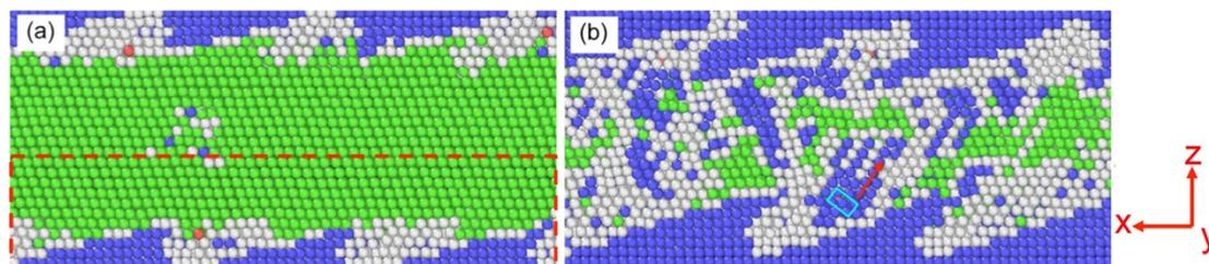
Figure 3-4 Time evolution of phase transformation in the original fcc part, which lies between the black and yellow lines in figure 3-3, (a) 0.5 ps, (b) 1.5 ps. The colours denote the local crystal structure as in figure 3-1.
