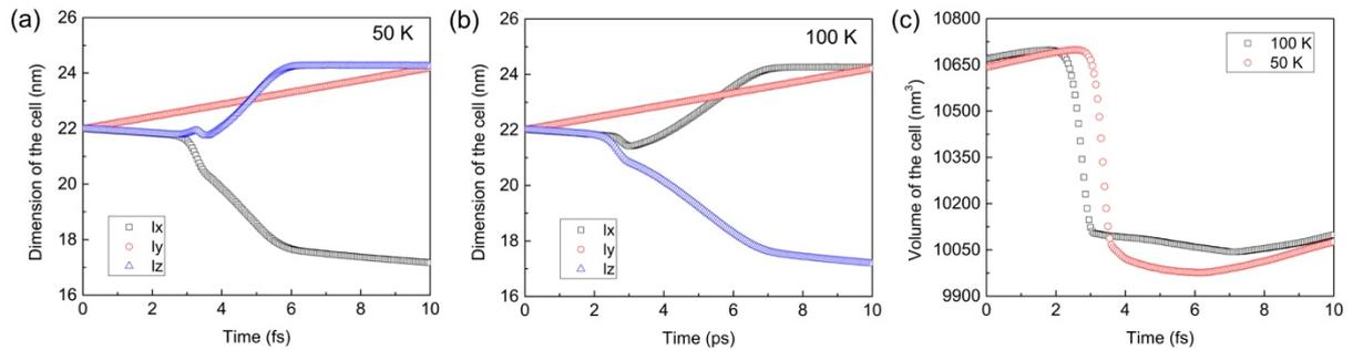
Figure 7-6 (a) Time evolution of the dimensions of the simulation cell at 50 K; (b) Time evolution of the dimensions of the simulation cell at 100 K; (c) Time evolution of the volume of the simulation cells both at 50 K and 100 K.  $l_x$ ,  $l_y$  and  $l_z$  represent the length of the simulation cell in the  $x$ ,  $y$  and  $z$  directions.
