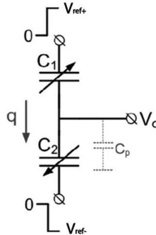
Fig. 7. Middle electrode sense scheme [21].
