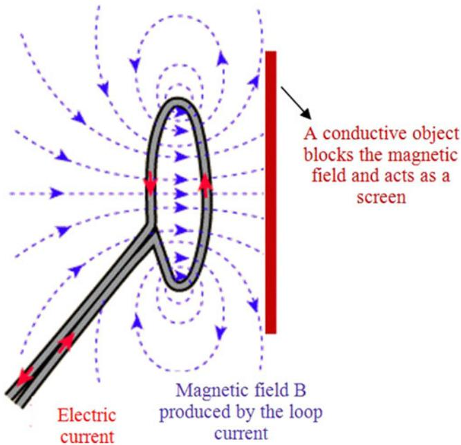
Fig. 14. Magnetic field  $B$  (dashed lines) created by an electric current through a loop.
