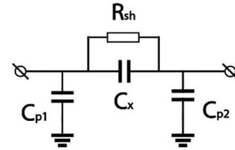
Fig. 2. Electrical model of a capacitive sensor [4].
