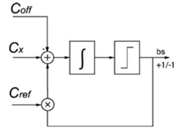
Fig. 11. Example of a CDC based on a first-order charge-balancing delta sigma modulator [32].
