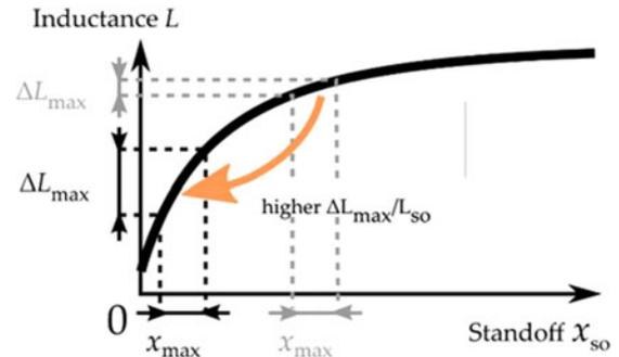
Fig. 15. Typical transfer characteristic  $L(x)$  of an ECS, showing the difference in the maximum variation of the inductance  $\Delta L_{\max}$ , for the same displacement  $x_{\max}$ , at different standoff distances.
