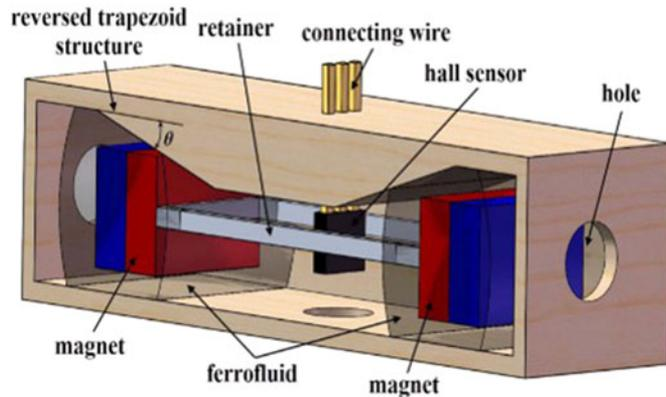
Fig. 23. Ferrofluid and Hall effect sensor-based inclinometer [71].
