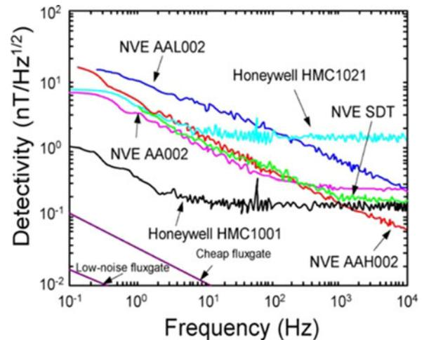
**Fig. 20.** Noise performance of various magnetic sensors [56]. NVE AAL002, NVE AA002, and NVE AAH002 are GMR-based sensors [62], while NVE SDT is a tunneling magnetoresistance (TMR) based sensor.
