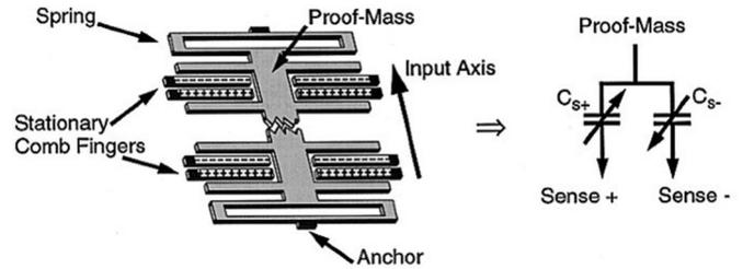
Fig. 3. Differential capacitive acceleration sensing element [22].
