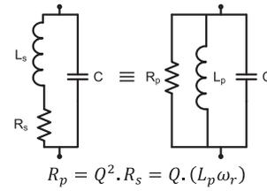
**Fig. 16.** Equivalent electric models of the sensing coil.
