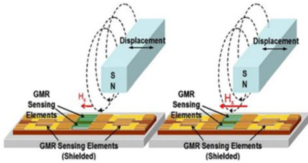
Fig. 21. GMR-based sensor for nanopositioning [54].
