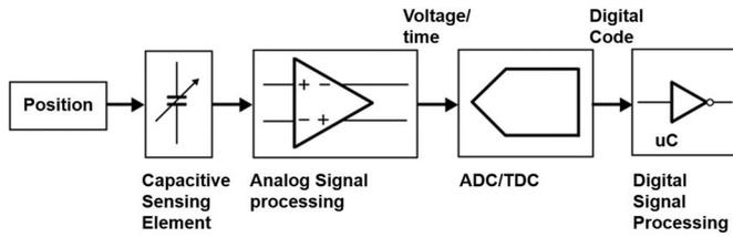
Fig. 4. Capacitance-to-voltage/time-to-digital converter.
