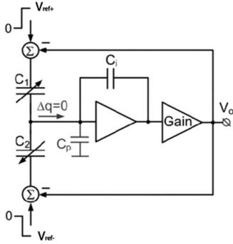
Fig. 8. Charge balanced capacitance-to-voltage converter [21].  $V_o$  is the output voltage.
