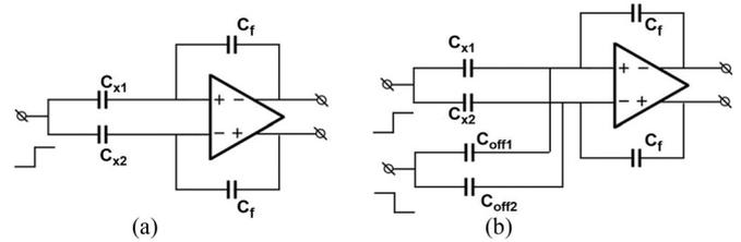
Fig. 6. Middle electrode drive scheme: (a) conceptual idea and (b) with common mode correction.
