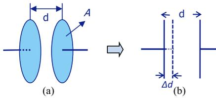
Fig. 1. (a) A parallel-plate capacitive position sensor and (b) working principle [2].
