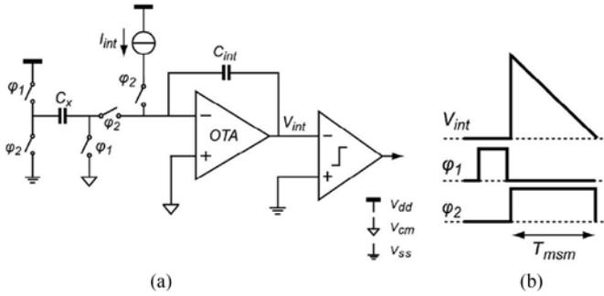
Fig. 9. Simple capacitance-to-time converter: (a) circuit and (b) timing diagram [28].
