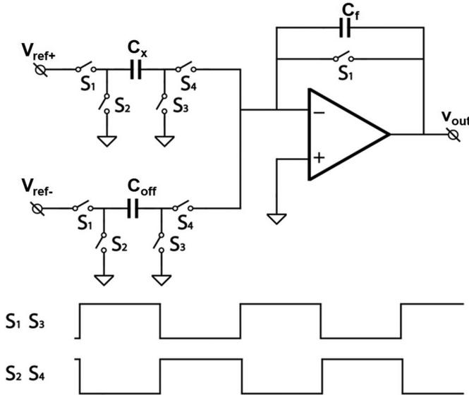
Fig. 5. Charge amplifier for the single-ended sensor.
