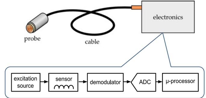
**Fig. 17.** Conventional architecture of an ECS interface.
