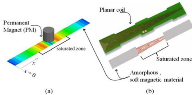
**Fig. 19.** Magneto-inductive position sensor. It uses (a) a PM and soft magnetic material, and (b) a planar coil, whose effective area is modulated depending on the position of the PM [52].
