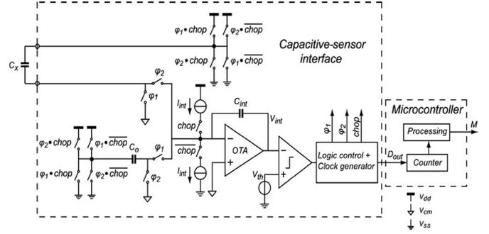
Fig. 10. Example of a capacitance-to-period modulator [29].
