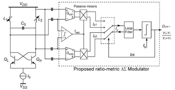
**Fig. 18.** Read-out circuit for an ECS-based displacement sensor with digital output (inductance-to-digital converter: IDC).
