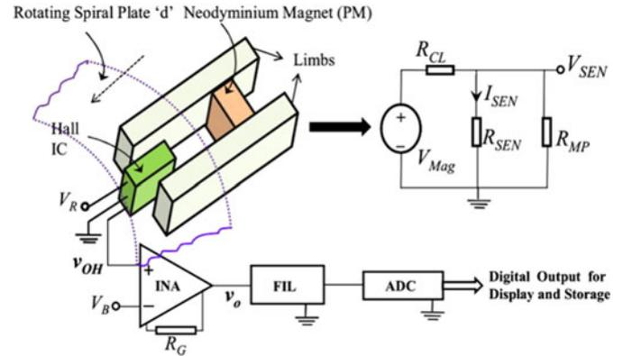
Fig. 22. Variable reluctance Hall effect angle sensor [60]. An electrical analogy is also shown.  $R_{MP}$  corresponds to the reluctance of the path through the moving part, while  $R_{SEN}$  and  $R_{CL}$  represent the reluctance of the section of path through the Hall sensor and the section of path through the limb.
