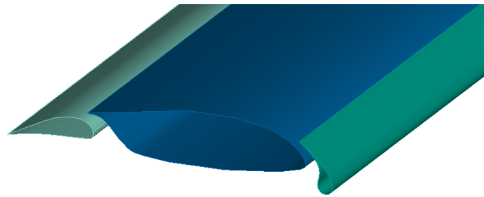
Figure 2.5: Multi-element wing generated using ParaWing.
