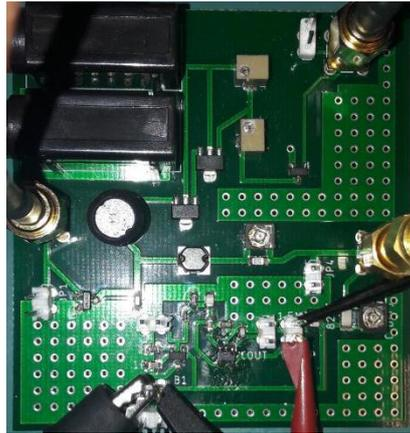
Figure 37. Transmitter PCB
