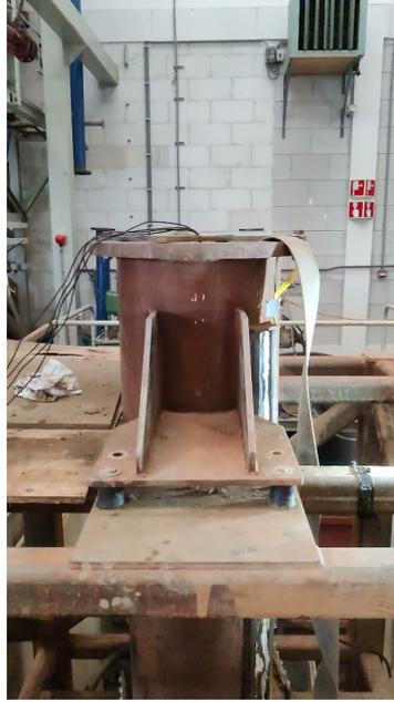
Figure 5.4: Front view of the set up. Up top the cables of the TEROS12 sensors as well as the PVD can be seen. Furthermore 2 dampening rubbers are presented, in total 8 were used for the entire set up
