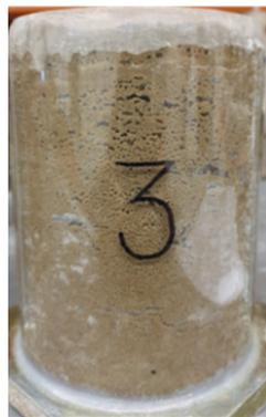
Figure 7.4: Sample showing gas distribution of treated sample, by: Stals 2020
