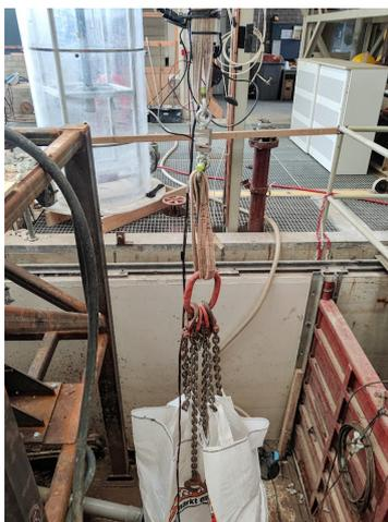
Figure 5.1: Load cell attached to a big bag
