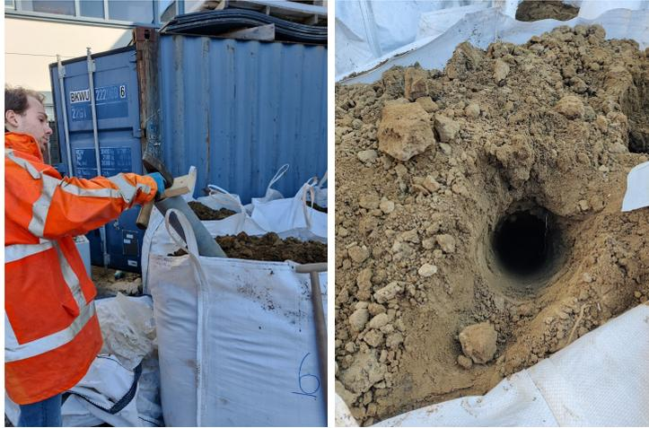
Figure 3.2: Sampling of big bag 6 on three different elevations in the big bag, by means of a PVC tube. Due to low cohesion of the soil the pvc tube was hammered in at an angle of roughly 30 degrees from the vertical.
