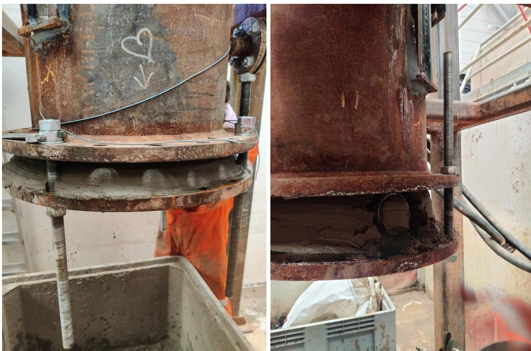
Figure 5.10: Tests U16N (left) and T16N2 (right), after compaction. Note how the bolts were inserted in the right image to keep the bolts as clean as possible. In the right image a sampling ring can be observed.
