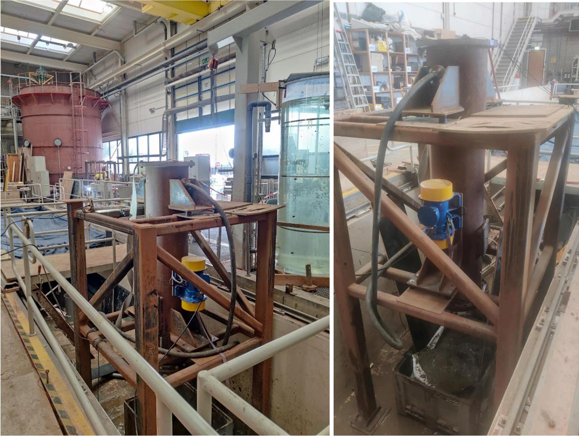
Figure 5.3: Images of the set up, note the vibrating engine in yellow and blue
