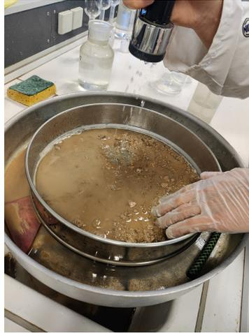
Figure 3.5: Sieving through the 63  $\mu\text{m}$  sieve to determine the fines fraction
