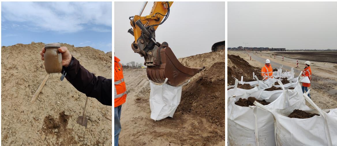
Figure 3.1: Sampling of test material by means of a visual settling test, left.
