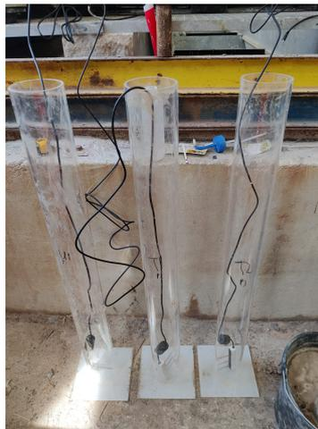
Figure 4.1: Empty 1m tubes, each with a TEROS12 sensor
