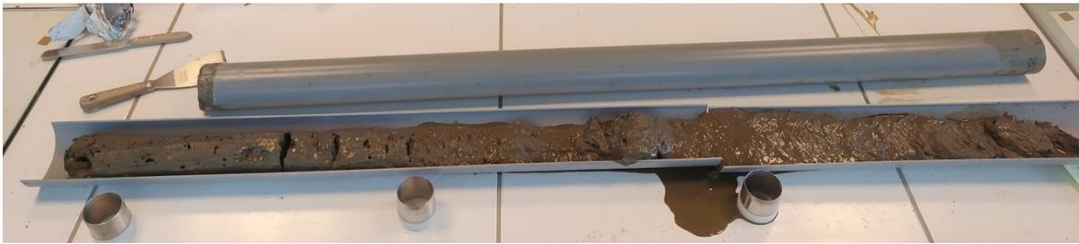
Figure 6.7: PVC samples after compaction. Left side is the lower part of the cylinder and right side the top of the cylinder. Test T1630
