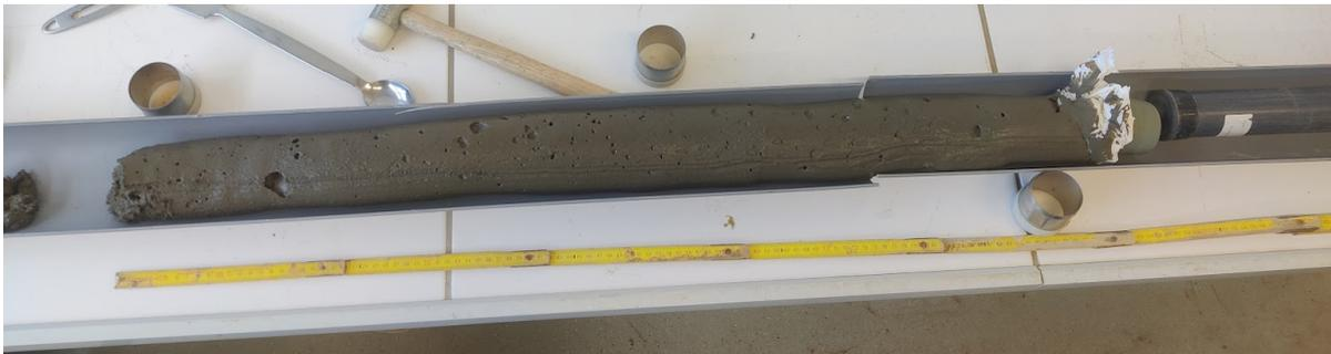
Figure 6.10: PVC samples after compaction. Left side is the lower part of the cylinder and right side the top of the cylinder. Test T16100\_2, note the gas volume that is still present in the lower part of the sample
