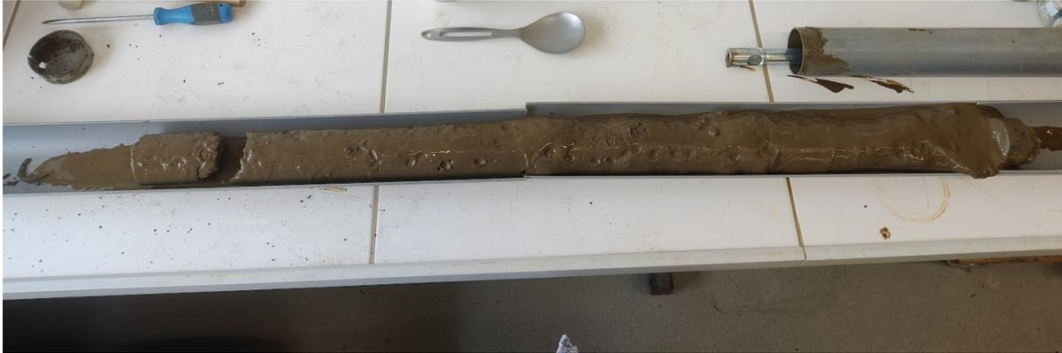
Figure 6.9: PVC samples after compaction. Left side is the lower part of the cylinder and right side the top of the cylinder. Test T16100
