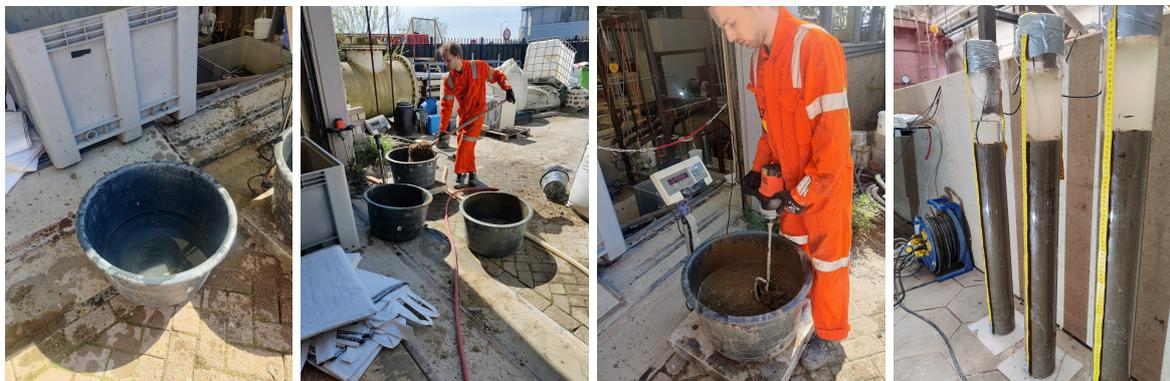
Figure 4.2: Methodology preparing a homogeneous sample. From left to right (1-4): The bucket being filled with water (1), followed by soil (2). Then mixing the slurry (3) and lastly pouring it in the tubes resulting in the final situation (4).
