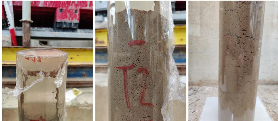
Bulging of sealing cap (left). Gas distribution in sample T2 (upper part middle and lower part right)
