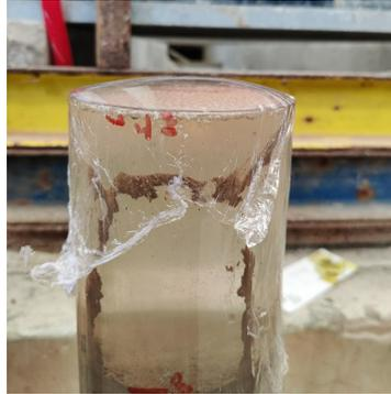
Figure 6.4: SH1 sample T2. Cling film bulging outwards due to gas production
