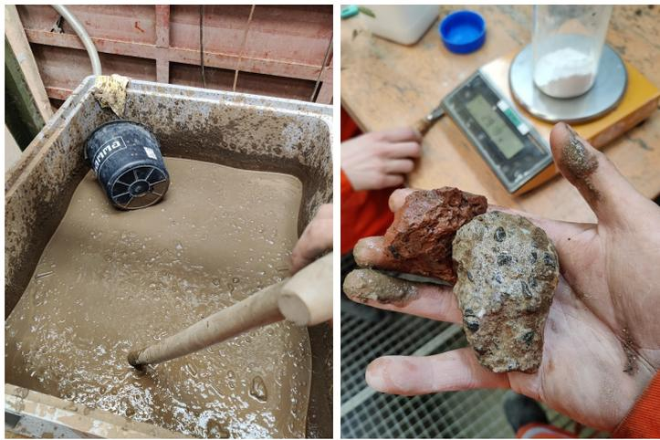
Figure 3.4: Mixed slurry, with lumps of organic material floating on top (left) and encountered rocks in the soil (right)
