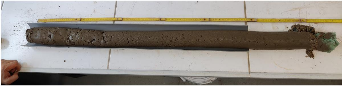
Figure 6.11: PVC samples after compaction. Left is the lower part of the cylinder and right the top of the cylinder. Test T16100sur, gas is still present in the lower part of the sample
