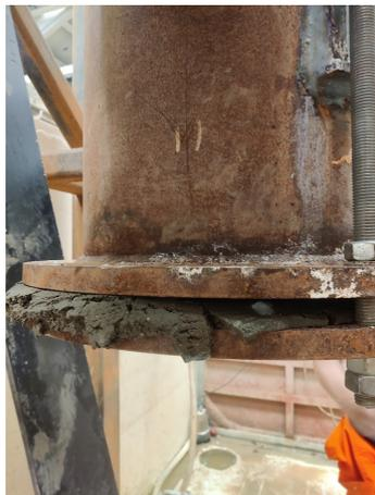
Compaction rating slurry to weakly compacted
