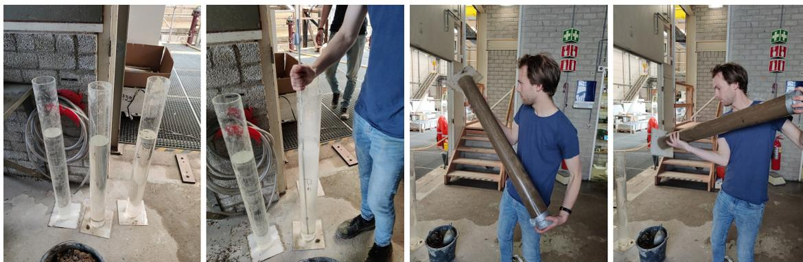
Figure 4.3: Placement methodology for a layered sample. From left to right (1-4): The water tubes filled with water (1), followed by the nutrients (2). Sequentially the tubes are filled with soil and mixed (3,4)
