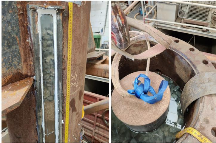
Figure 5.8: Set up of surcharge, layering of drainage sand and gravel on top of the soil sample (left). The leaden weight, left with some slack in the crane for safety, notice the waterlevel just below the overflow (right)
