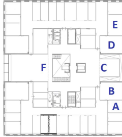
Figure 3.14: Floor-plan of group-positions of thirty devices in six groups at SF7 (gateway in group C).
