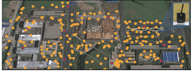
Figure 1.3: Partially deployment of CitySee: red nodes and yellow nodes represent carbon dioxide and temperature/humidity sensors, respectively [17].
