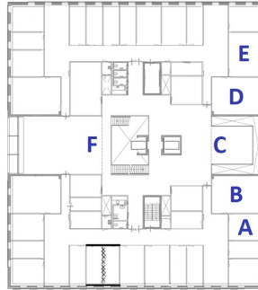
Figure 5.25: Thirty devices distributed per five devices per group in six groups. Floor-plan of campus building with group-positions according to their SF Gateway positioned with group C.
