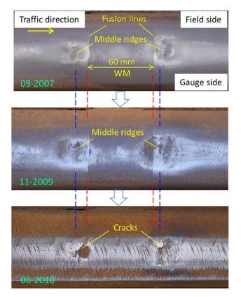
**Fig. 3.** Another example of thermite welds with duo squats in the first (09-2007), fifth (11-2009) and sixth (06-2010, after a rail grinding) observations, where the WM was approximately 60 mm in length. This is the same squat as that shown in Fig. 1(a).
