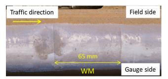
Fig. 5. Single squat at a thermite weld observed at Nijeveen in the Netherlands.
