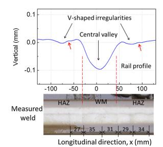
**Fig. 8.** Measured profile of a thermite weld without cracks: V-shaped irregularities were in both HAZs (the length of WM was approximately 73 mm). If the two small peaks indicated by the two red arrows are considered, each of the V-dips was evolving towards a W-shape. Waves were visible on the rail surface with the wavelength indicated in the photo. (For interpretation of the references to colour in this figure legend, the reader is referred to the web version of this article.)
