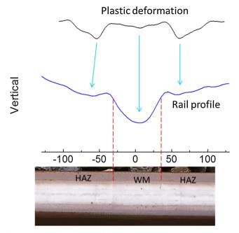
**Fig. 15.** Comparison of the calculated surface irregularities due to plastic deformation (upper curve) in Step 1 with the surface irregularities measured at the thermite weld of Fig. 7(b) (lower curve).
