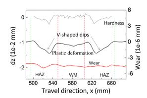
Fig. 14. Surface vertical plastic deformation dz and wear (average smoothing within a radius of 5.5 mm) of Step 1 along the center of the running band at the thermite weld (negative ordinates mean that the directions of deformation and wear are downwards relative to the initial (smooth) rail surface).
