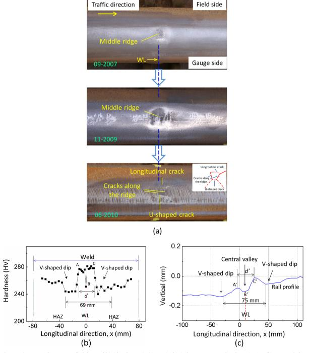
**Fig. 6.** (a) The growth process of a squat at a flash butt weld (with only one single squat). This is the same squat as that shown in Fig. 1(b). WL stands for Weld Line; (b) W-shaped hardness distribution measured at a virgin flash butt weld. The two V-shapes are on the two sides of the weld line; (c) Measured vertical-longitudinal rail profile in 09-2007. The length *d*' of A'B'C' corresponds to the width *d* in the hardness plateau ABC of (b), but they are not necessarily the same.
