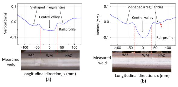
Fig. 7. Two thermite welds without cracks and their profiles. The length of the WM is approximately 64 mm in (a) and 67 mm in (b). If the small peak indicated by the red arrow is considered, the V-dip on the right side in (b) was evolving towards a W-shape. (For interpretation of the references to colour in this figure legend, the reader is referred to the web version of this article.)
