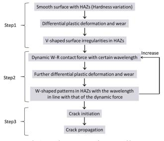
Fig. 10. Development process of squats at welds.
