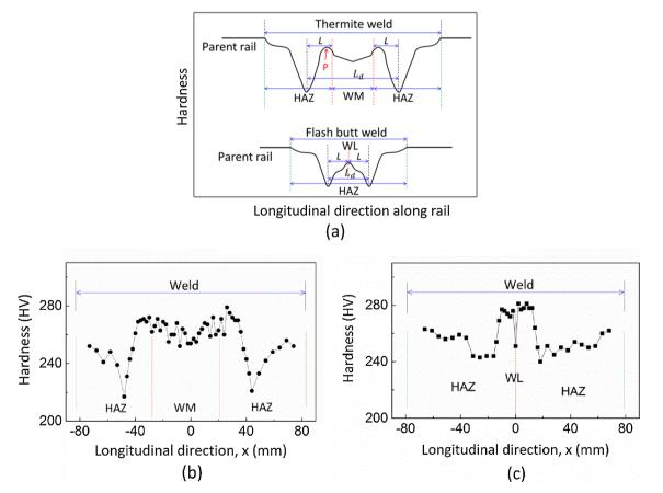
**Fig. 9.** Distributions of the hardness: (a) at a thermite weld and a flash butt weld, respectively (schematic diagram; the red dashed lines indicate the fusion lines); (b) at a virgin thermite weld (measured); (c) at a virgin flash butt weld (measured; this hardness distribution is the same as that in Fig. 6(b)). (For interpretation of the references to colour in this figure legend, the reader is referred to the web version of this article.)
