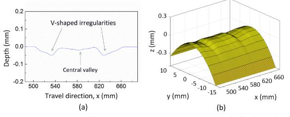
Fig. 16. Rail surface at the beginning of Step 2, obtained from the plastic deformation calculated in Step 1: longitudinal rail profile with two V-shaped irregularities at HAZs and one slight central valley at the WM. (a) Vertical-longitudinal profile and (b) the rail surface in 3D.
