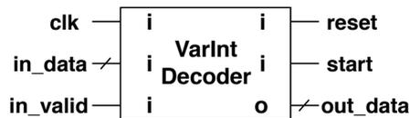
Figure 3.12: Top-level view of the VarIntDecoder module
