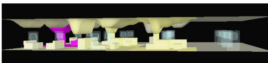
Fig 125: Light level variations displayed in the 3d section of the interface. Light levels are simulated in real-time via the control system.
