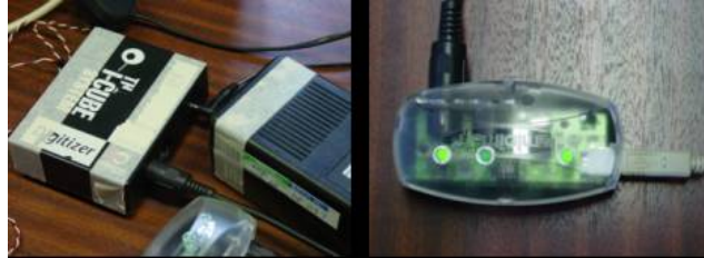
Figure 9. The I-Cube digitizer and the distributor of inputs from the digitizer
