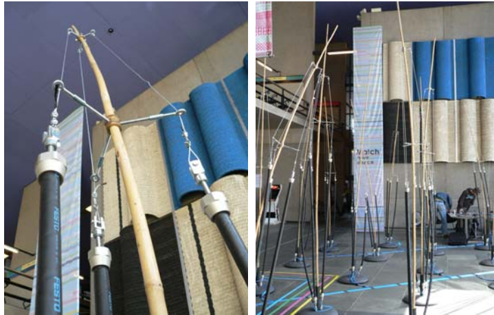
Fig.59. Components: bamboo stick, pneumatic muscles, two clamp assemblies woven together to create the kinetic construct.
