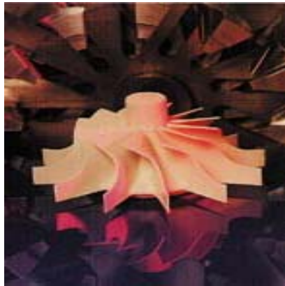
Turbine blades are among parts subject to wear that are made of ceramic material. This prototype gas turbine rotor is made of injection-moulded monolithic silicon nitride.
