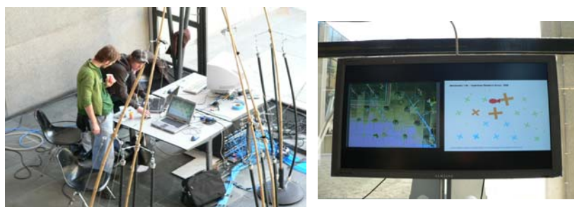
Fig.61. Images showing the computers hosting Vitriol's scripts connected to the black box (under the table) and the real time tracking of people and the gold fish.
