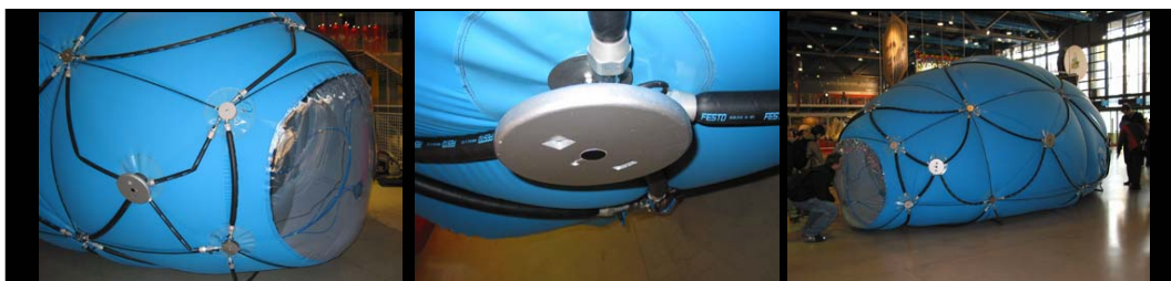
Fig. 9 The Muscle project: Kas Oosterhuis, an experimental prototype embedded with sensing and actuating devices, which responds to its surroundings by augmenting its form. The sensor disks, which create the nodes, are embedded with proximity and motion sensors, which sense user location and proximity and in turn via a programmed behaviour engine instruct the actuators (Festo pneumatic muscles) to contract/expand, hence causing the form to expand/contract.
