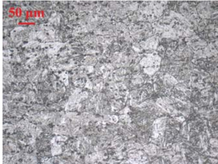
FIGURE 4.10. Optical micrographs of alloy CarCo after solution treatment at 1423 K for 15 minutes and quenching.
