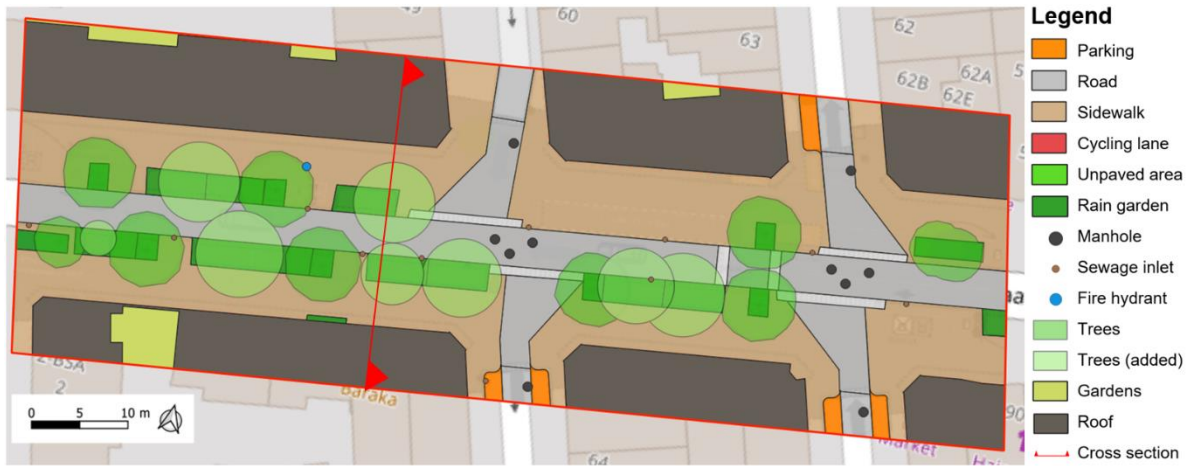
Figure 58 Aerial map (indicating land cover types) - Kanaalstraat – proposed design + no on-street parking + rain gardens (Sc3)
