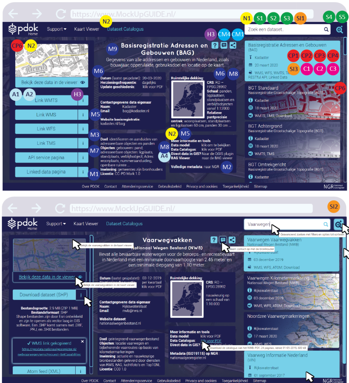
Figure 6.23: Catalogue page of the mock-up design according to the UI design elements as listed in the GUIDE. The lower part of the image is meant to indicate how the possible interactions look on the page.
