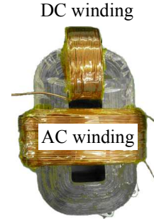
Figure 2-37: Experimental open-core FCL.
