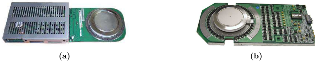
Figure 2-39: Semiconductor modules: (a) IGCT module; (b) SPETO module.
