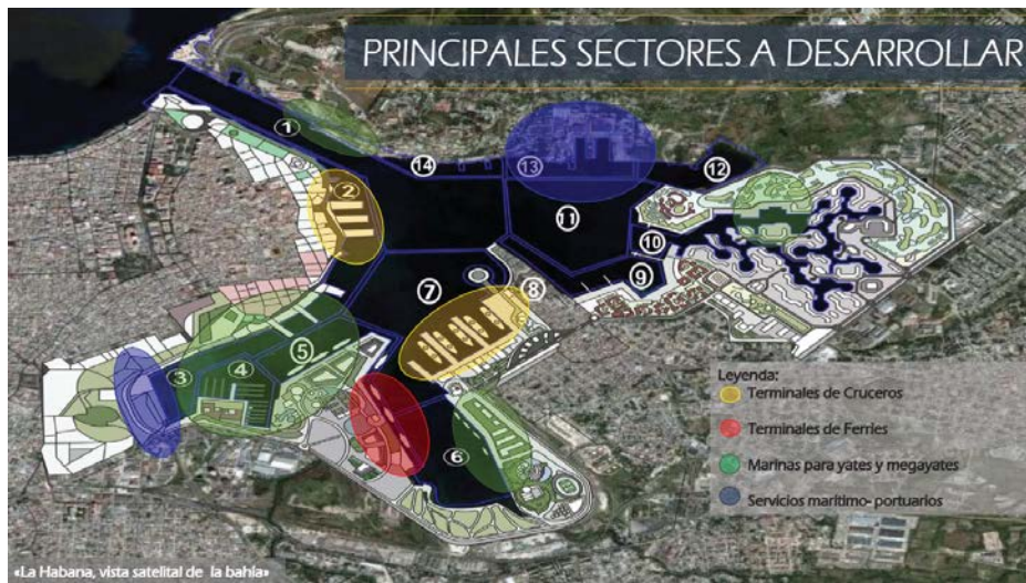
Figure 1 - Impression of the reference project: integral development plan of the bay of Havana. Legend: 1, 4, 5, 6, = marina for yachts and mega yachts, 2, 7 = cruise terminals, 3, 13 = maritime services (PID-BH, 2014)
