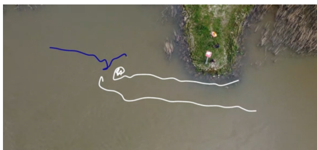
(a) Tracked path of the oranges around traditional groyne
