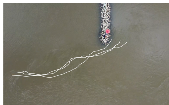
(b) Tracked path of the oranges around Xstream groyne
