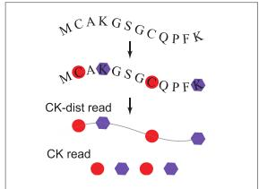
**Figure 1.** A single-molecule read-out. CK fingerprinting read: the order of C's and K's are detected. CK-dist fingerprinting read: the distances between C's and K's are additionally measured.
