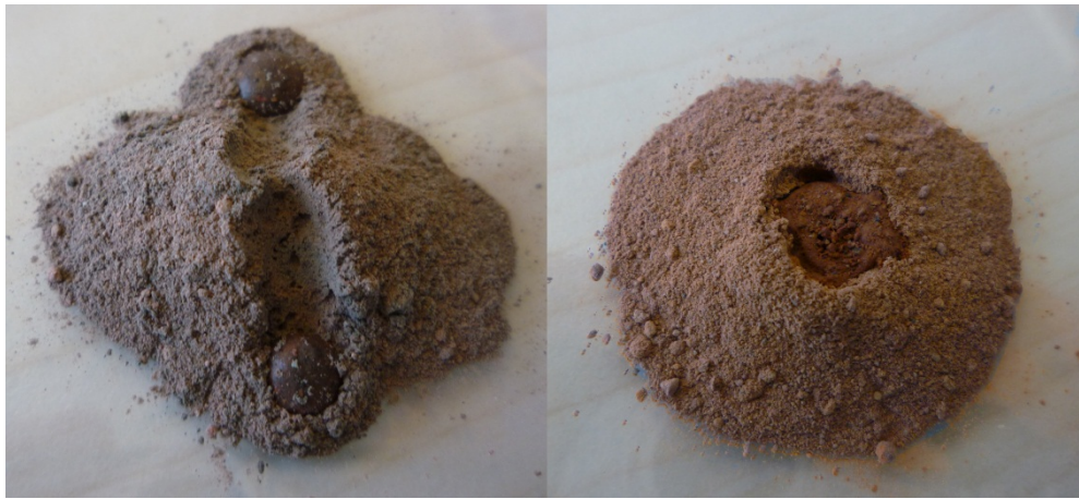
Figure 10. Sample with clear water repellent properties (left) and without these properties (right). A distinction can easily be made
