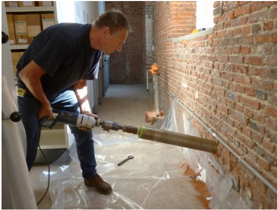
Figure 7. Drilling cores from treated and untreated masonry
