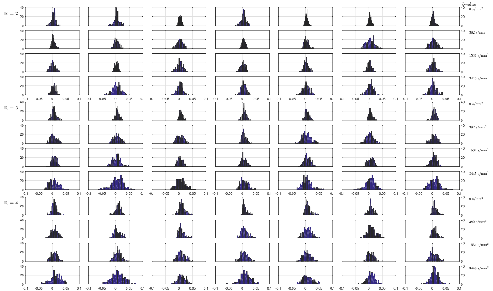
Figure B.2: Set of histograms visualizing the normalized difference in data between the PE undersampled vs full acquired after post-processing with the Roemer reconstruction in parameter-image space: equation (B.2). Each row depicts a different diffusion condition, each set of four rows a different acceleration factor ( R ), each column a different set of pseudo-random PE undersampling patterns for that R .
