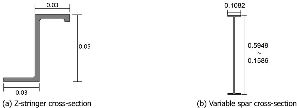
Figure 13.14: Stiffener cross-sections. All dimensions are in m.
