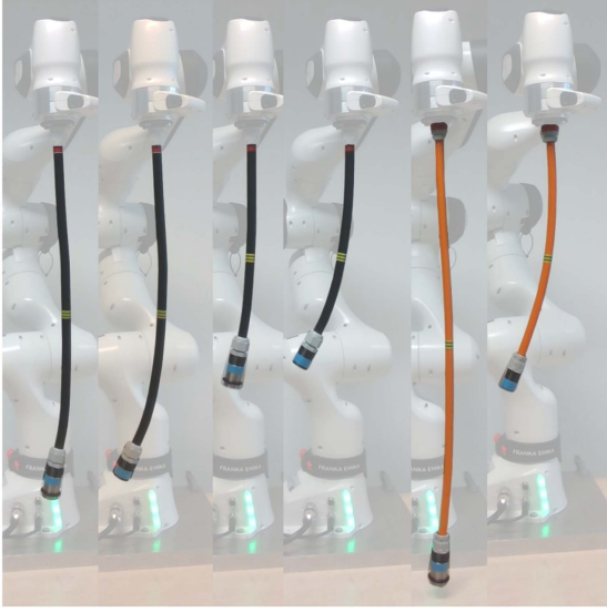
Fig. 3. Test objects used in the experiments, OB1-OB6 from left to right. These are high-voltage electric cables used in the context of the electric car industry. The cables end with a plug connector.
