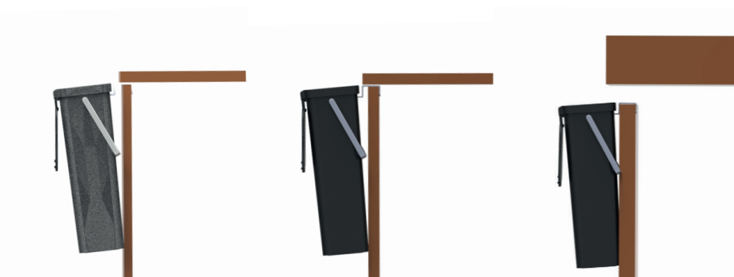
Figure 77 | Standard dimensions of kitchen counter and doors. Left: minimum distances. Middle: most common. Right: largest distances.
