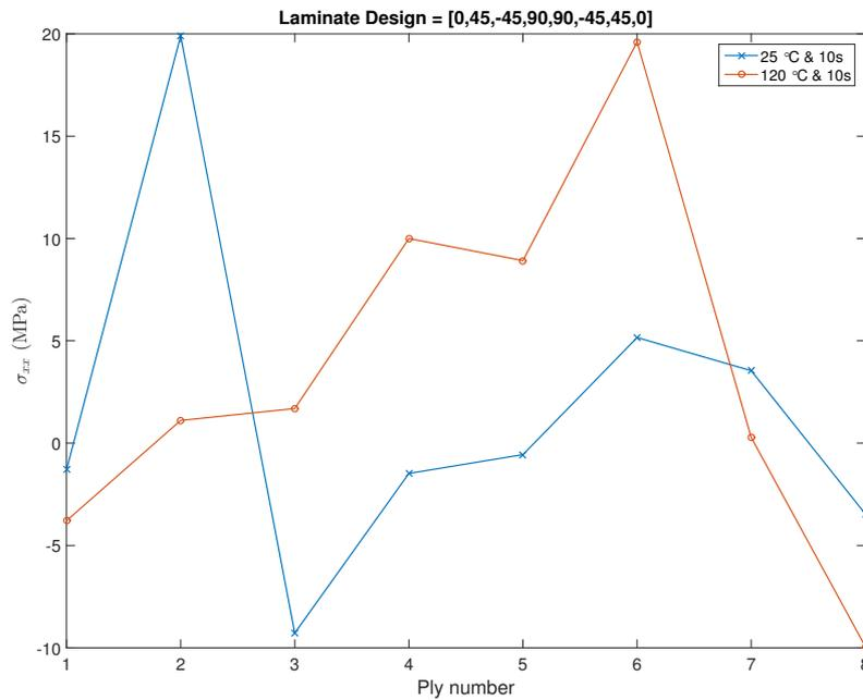
**Figure 7.5:** Residual Stress ( $\sigma_{xx}$ ) along the global X direction of each layer in the laminate at the end of the in - situ placement process.
