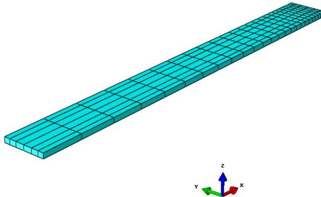
**Figure 4.16:** Biased mesh applied along the length of the tape part.
