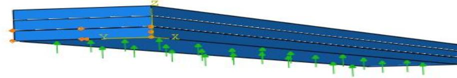
**Figure 4.4:** The heat flux load applied to the base of the first tape layer during the step 'S1', as shown by the green arrows.
