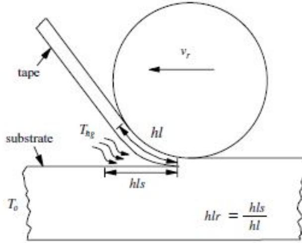
**Figure 2.5:** Various processing parameters in in - situ AFP technology [25]
