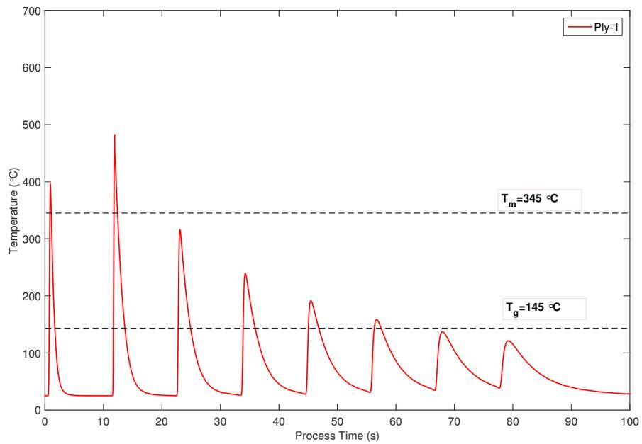
Figure 5.2: Thermal history of the first tape layer: Model-1.
