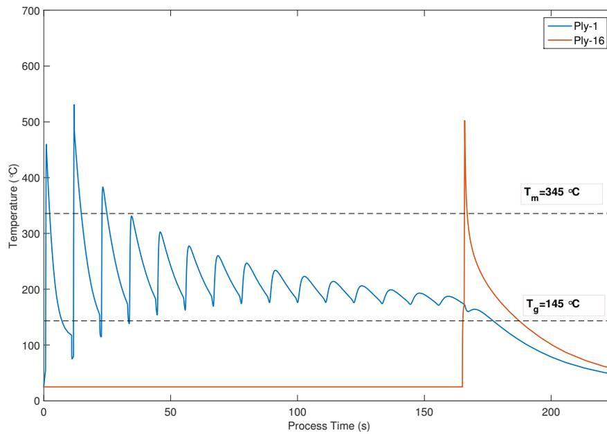
**Figure 5.25:** Comparison of the thermal history of the first tape layer and last placed layer: Model-12.
