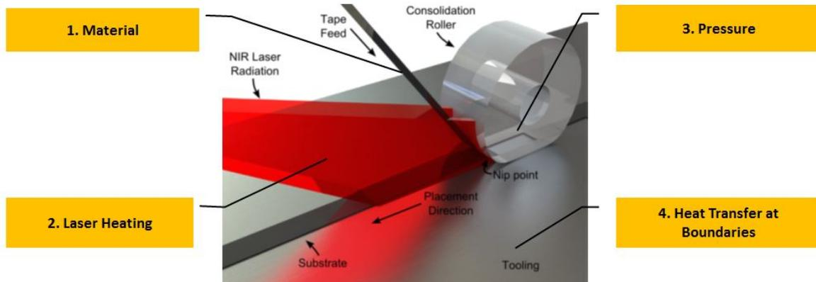
**Figure 3.1:** The four key modelling elements of the in - situ AFP process [20].
