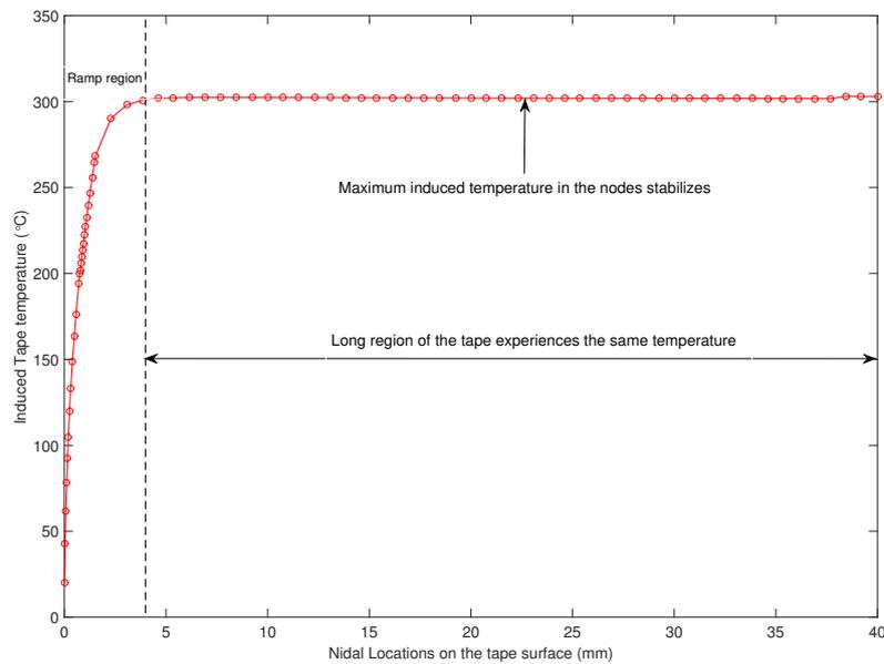
**Figure 4.12:** Maximum temperatures at the nodes for a 40 mm long tape length.
