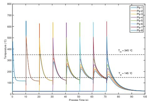
(f) Model v6 - 70 mm/s, 120 (°C) tool temperature & 3.1 mm heating length.
