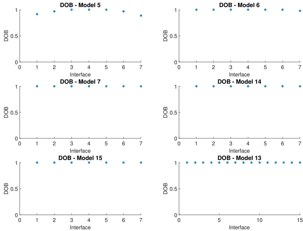
**Figure 6.7:** Degree of bonding achieved at each interface of the 8 ply laminate Models 5, 6, 7, 11, 14 and 15. (Tool return time = 1 s for all models)
