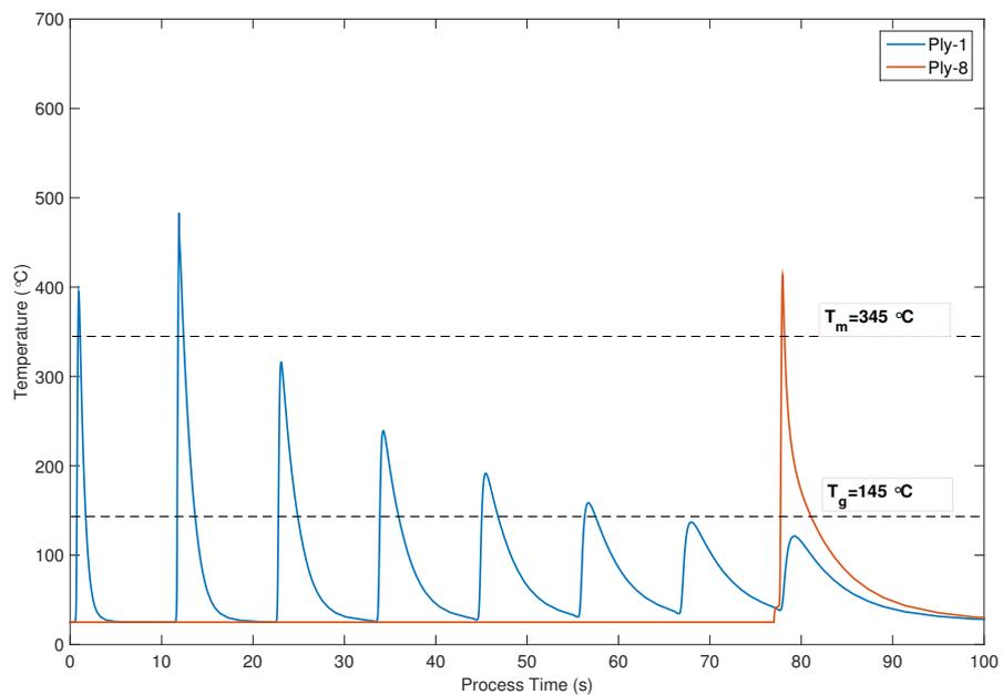
Figure 5.3: Comparison of the thermal history of the first tape layer and last placed layer: Model-1.
