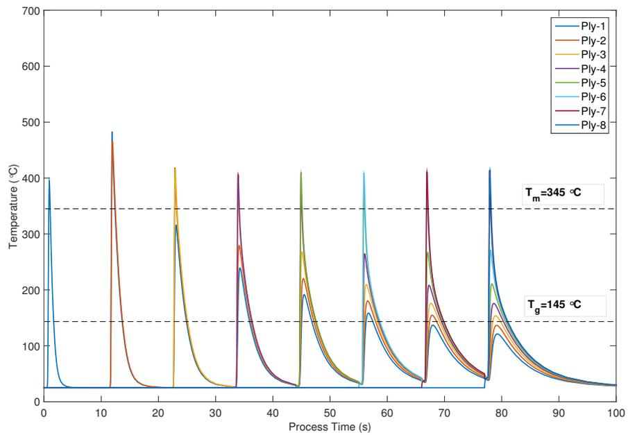
**Figure 5.33:** Thermal history of all tape layers of an 8 ply uni directional laminate,  $[0, 0, 0, 0]_s$
