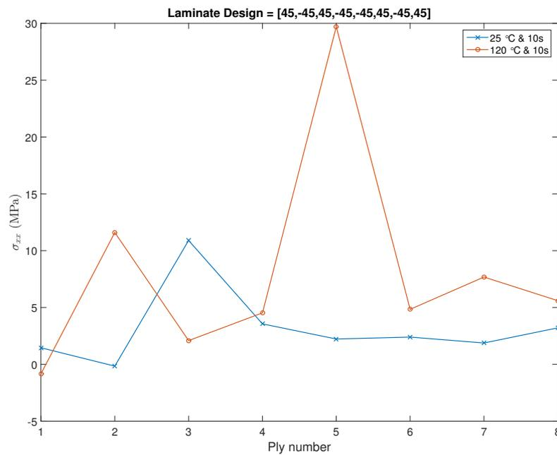
**Figure 7.9:** Residual Stress ( $\sigma_{xx}$ ) along the global X direction of each layer in the laminate at the end of the in - situ placement process.
