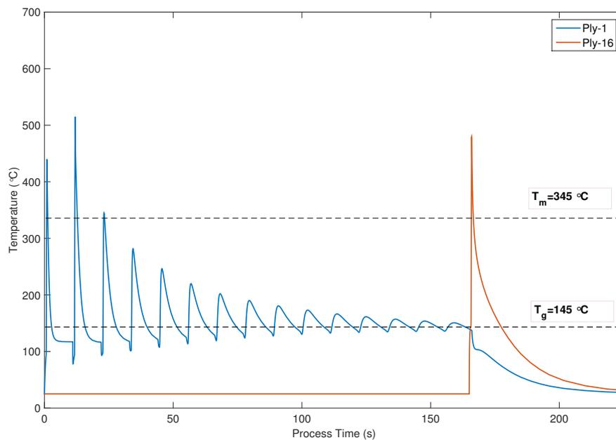
**Figure 5.10:** Comparison of the thermal history of the first tape layer and last placed layer: Model-9.
