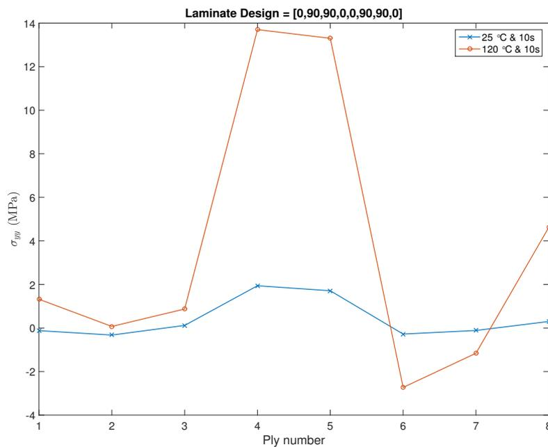
**Figure 7.4:** Residual Stress ( $\sigma_{yy}$ ) along the global Y direction of each layer in the laminate at the end of the in - situ placement process.
