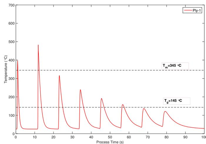
**Figure 5.36:** Thermal history of the first tape layer: Model-1.
