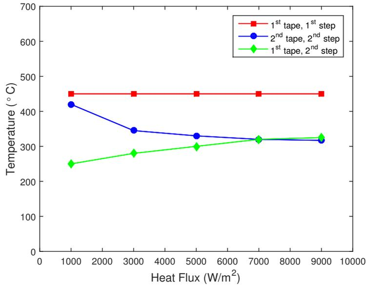
**Figure 4.21:** GAPCON sensitivity analysis for an interface between two layers
