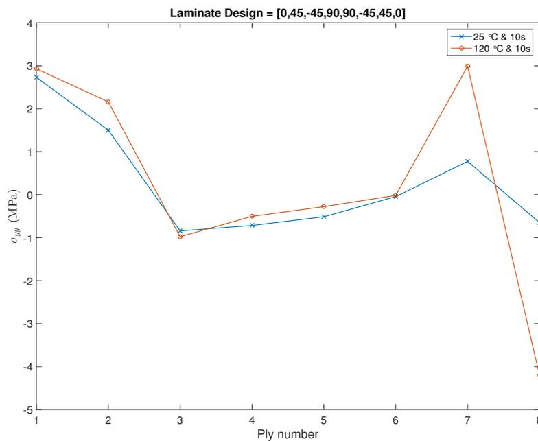
**Figure 7.6:** Residual Stress ( $\sigma_{yy}$ ) along the global Y direction of each layer in the laminate at the end of the in - situ placement process.
