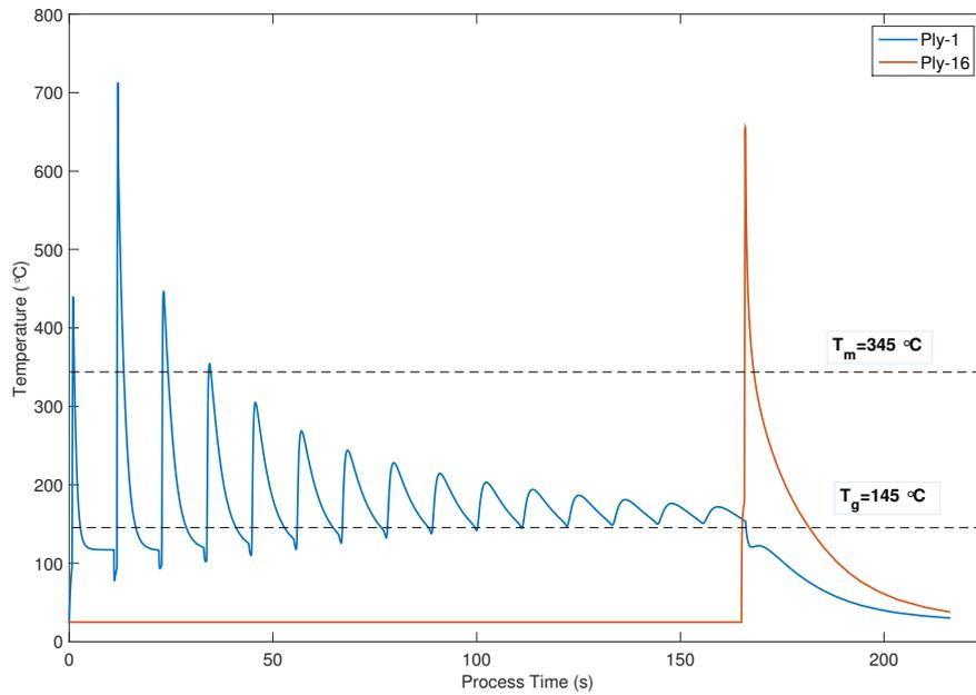
**Figure 5.14:** Comparison of the thermal history of the first tape layer and last placed layer: Model-10.
