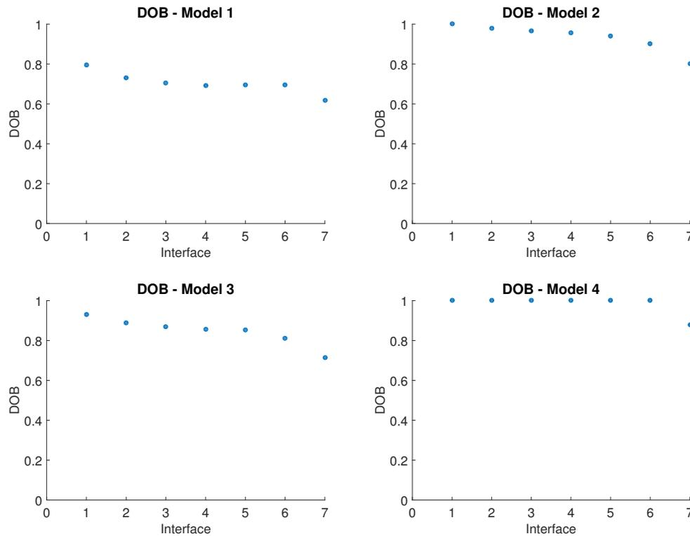
**Figure 6.5:** Degree of bonding achieved at each interface of the 8 ply laminate Models 1, 2, 3 and 4.
