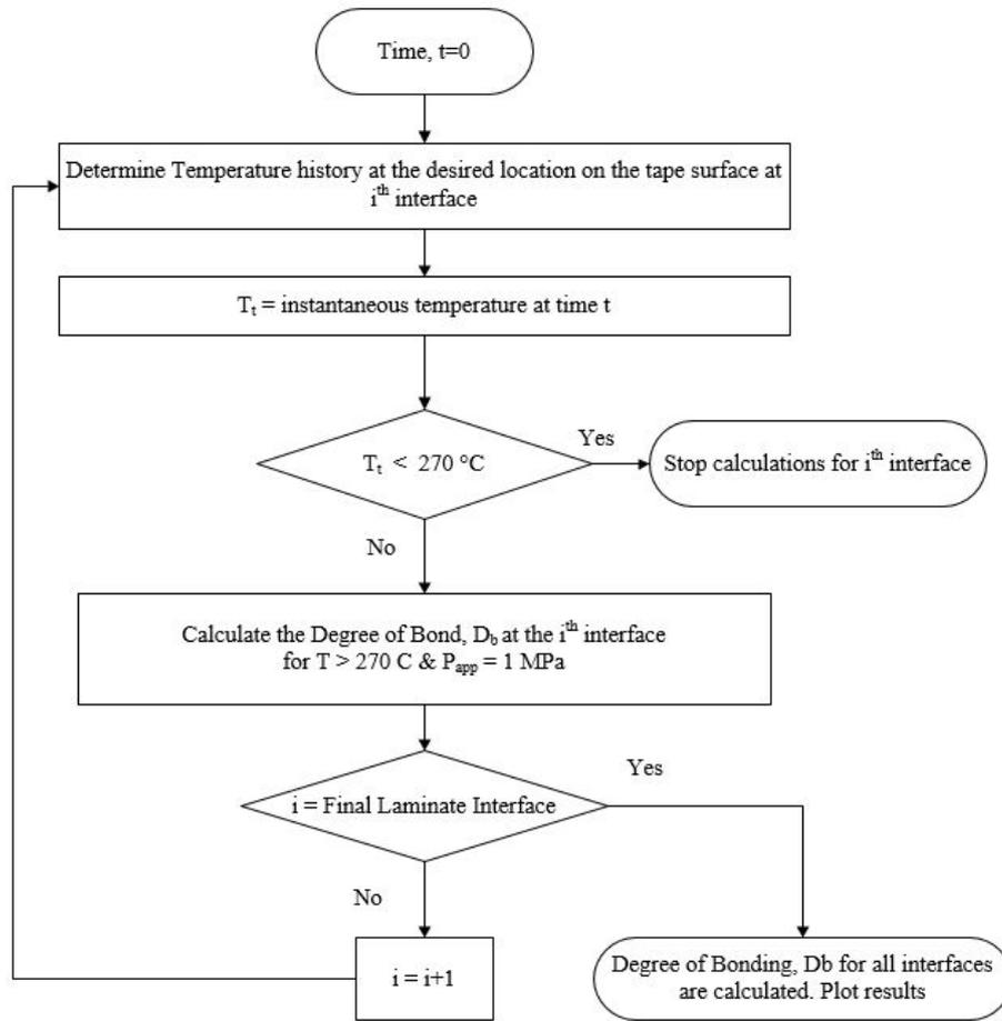
**Figure 6.1:** The solution procedure for calculating the Degree of Bonding,  $D_b$  at the interface of the tape layers.
