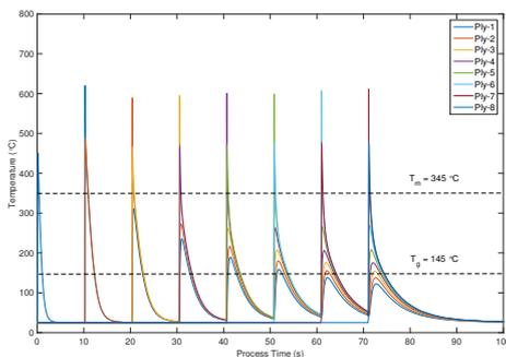
(e) Model v5 - 70 mm/s, 25 (°C) tool temperature & 3.1 mm heating length.
