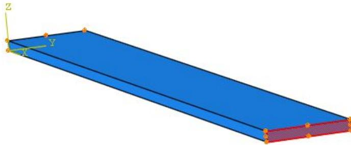
**Figure 4.9:** Boundary condition, Laid, at the end of the length, created in the tool return steps.
