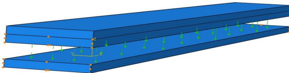
**Figure 4.6:** The heat flux load applied to the top surface of the first tape layer during the step 'S2', as shown by the green arrows. (Tape layers shown here are in an exploded view.)
