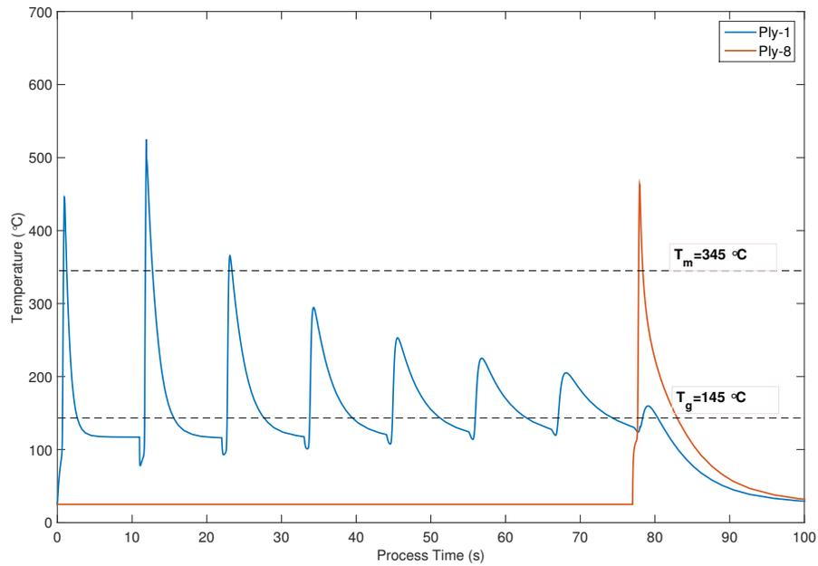
**Figure 5.9:** Comparison of the thermal history of the first tape layer and last placed layer: Model-3.
