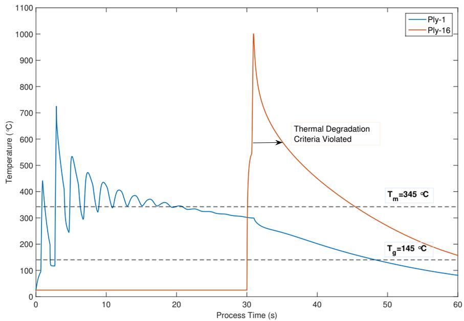
**Figure 5.20:** Comparison of the thermal history of the first tape layer and last placed layer: Model-11.
