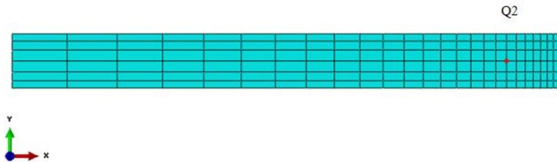
**Figure 3.10:** The positions of the query nodes Q2 - Top view of the tape part.
