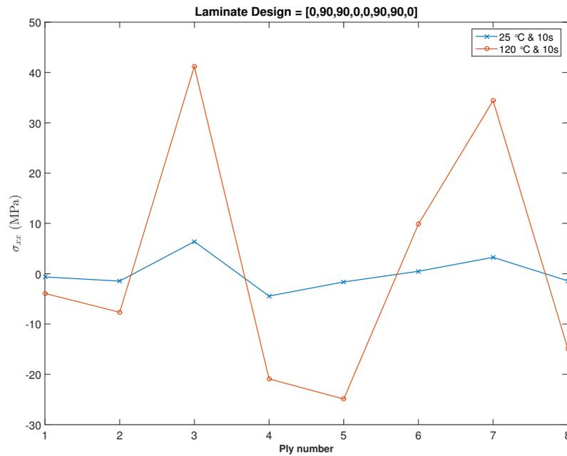
**Figure 7.3:** Residual Stress ( $\sigma_{xx}$ ) along the global X direction of each layer in the laminate at the end of the in - situ placement process.
