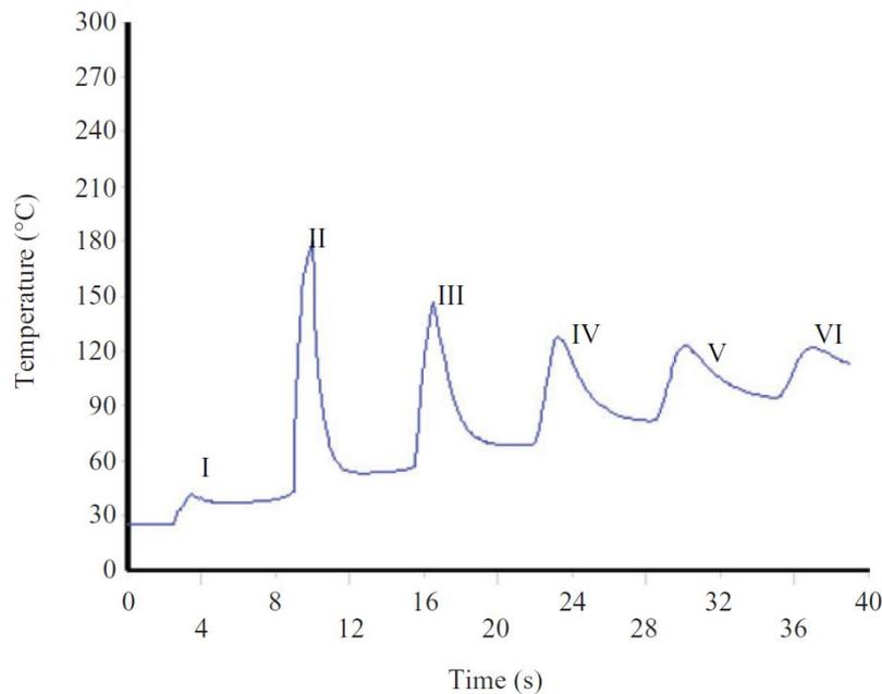
**Figure 5.35:** Temperature history in the first tape layer of a 6 layer placement process [49].
