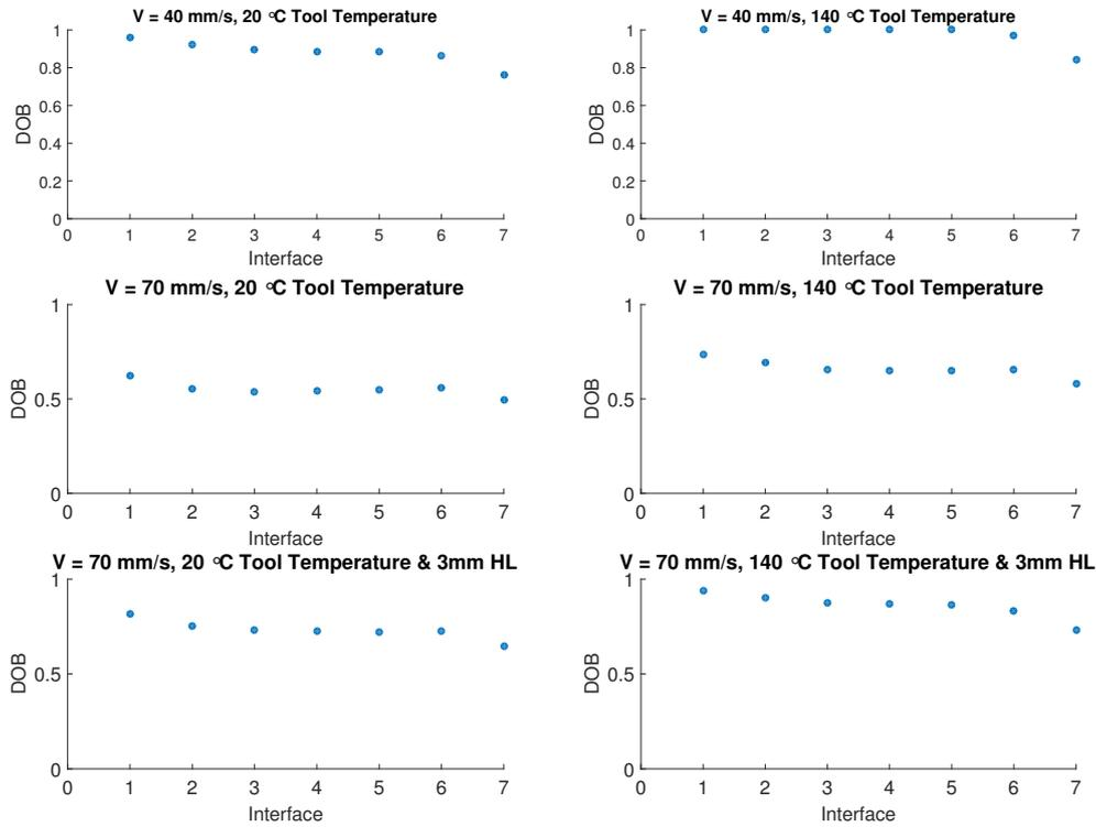
**Figure 6.8:** Degree of bonding achieved at each interface of the 8 ply laminate models v1, v2, v3, v4 v5 and v6.
