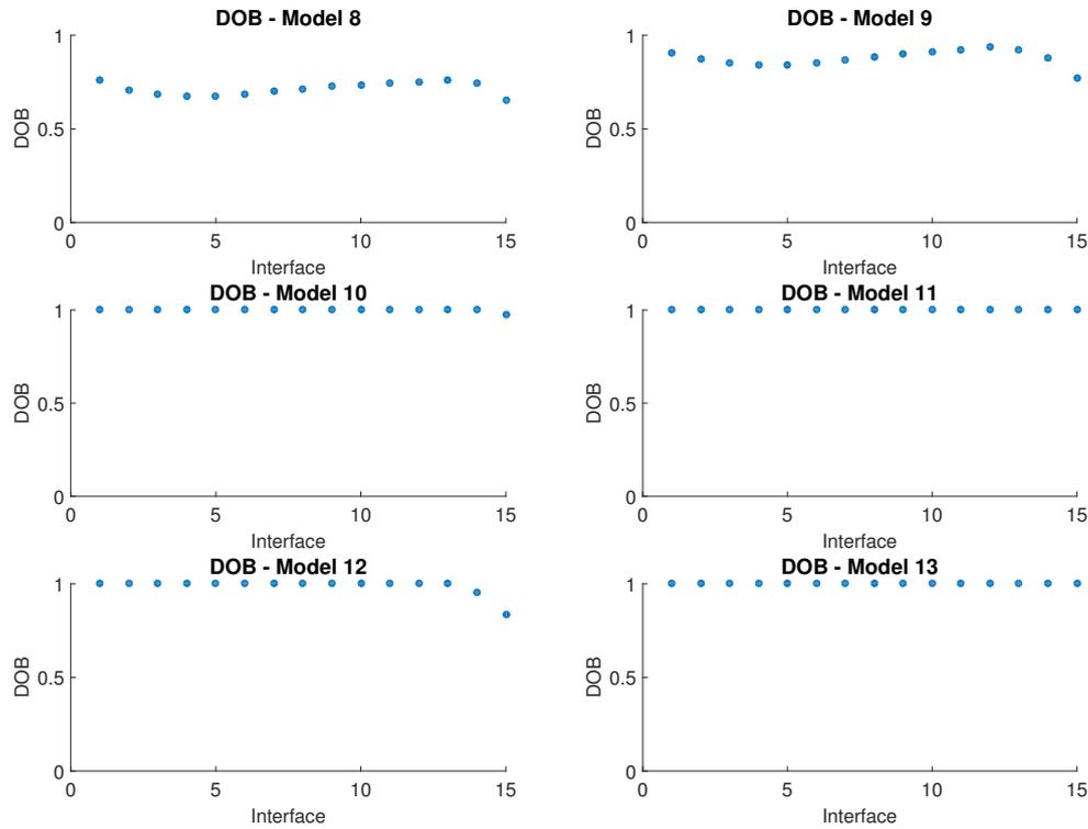
**Figure 6.6:** Degree of bonding achieved at each interface of the 8 ply laminate Models 8, 9, 10, 12 and 13.
