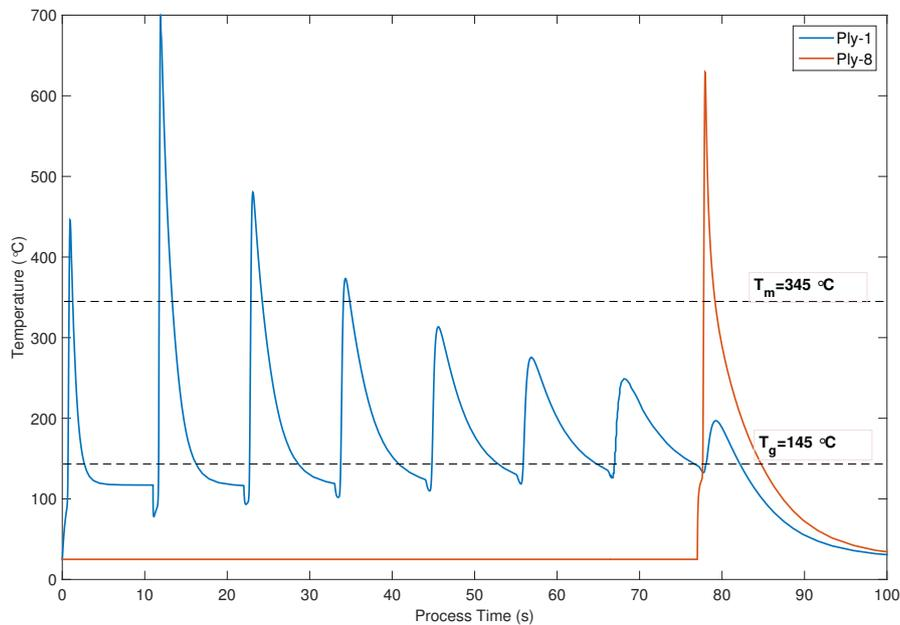
**Figure 5.13:** Comparison of the thermal history of the first tape layer and last placed layer: Model-4.
