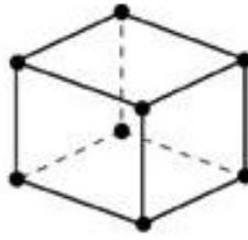
**Figure 3.5:** Linear 8 - node brick element (C3D8). Source: ABAQUS Online Documentation.
