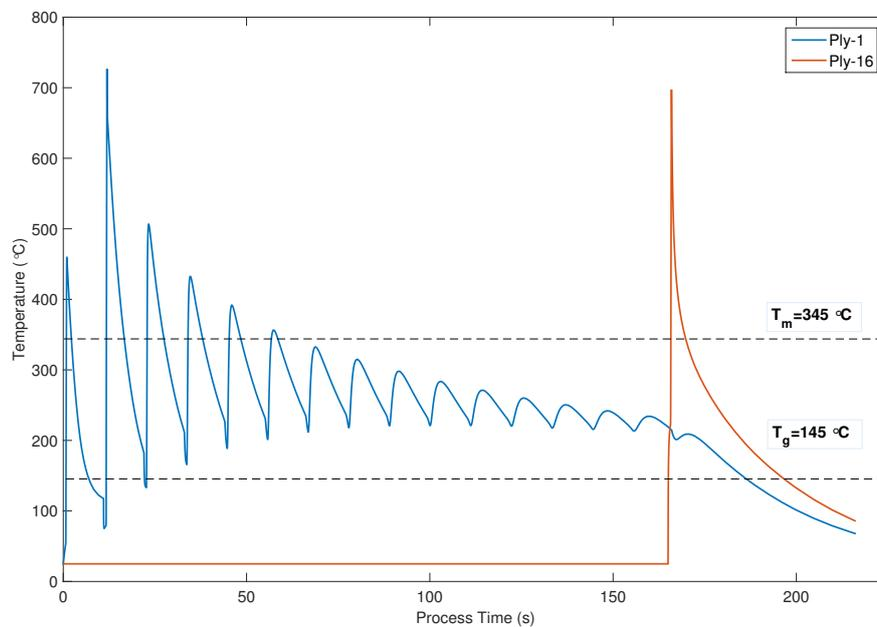
**Figure 5.26:** Comparison of the thermal history of the first tape layer and last placed layer: Model-13.
