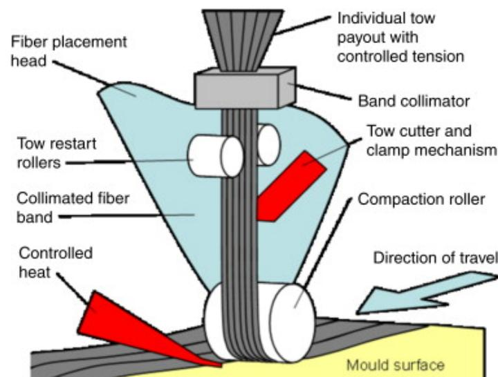
**Figure 2.1:** The In - Situ Automated Fibre Placement Process [9].
