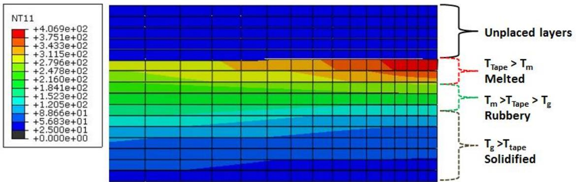
**Figure 5.1:** Temperature distributions in a 16 layer laminate (Model-8) simulation at the end of the 11<sup>th</sup> ply placement step 'S11'.
