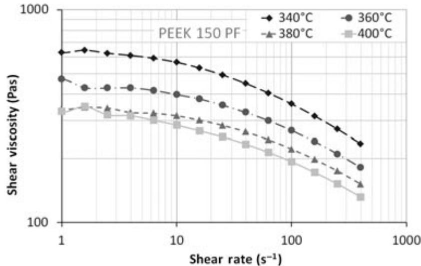
**Figure 2.4:** Viscosity plot for Victrex PEEK 150PF at different temperatures measured with a parallel plate rheometer [26].
