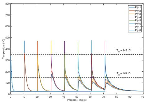
(c) Model v3 - 70 mm/s, 25 (°C) tool temperature & 2.1 mm heating length.
