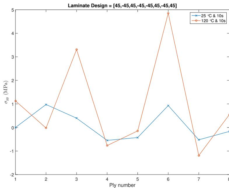
**Figure 7.10:** Residual Stress ( $\sigma_{yy}$ ) along the global Y direction of each layer in the laminate at the end of the in - situ placement process.
