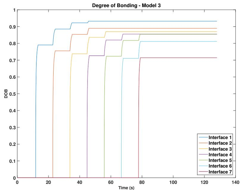
**Figure 6.3:** Degree of bonding achieved at each interface of the laminate for Model 3.
