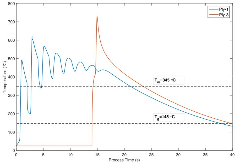
**Figure 5.27:** Comparison of the thermal history of the first tape layer and last placed layer: Model-14.
