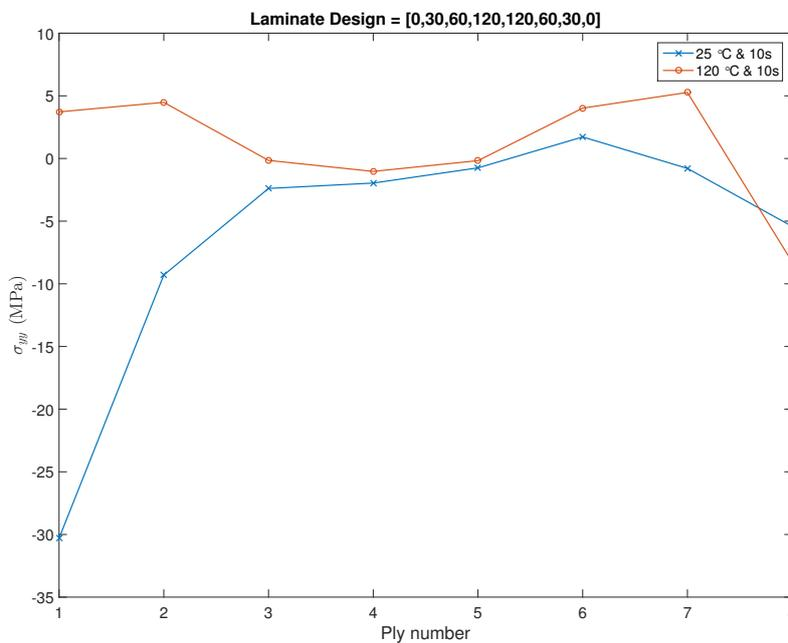
**Figure 7.8:** Residual Stress ( $\sigma_{yy}$ ) along the global Y direction of each layer in the laminate at the end of the in - situ placement process.
