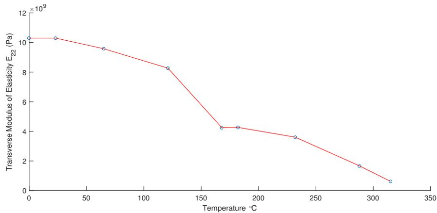
**Figure 4.2:** Variation of the transverse modulus of APC-2 with respect to temperature [11].
