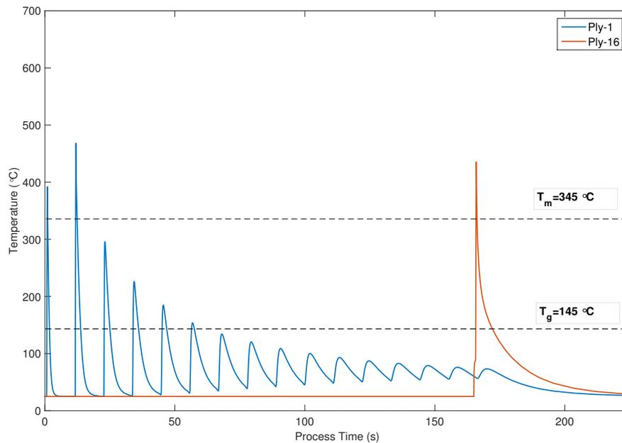
Figure 5.5: Comparison of the thermal history of the first tape layer and last placed layer: Model-8.
