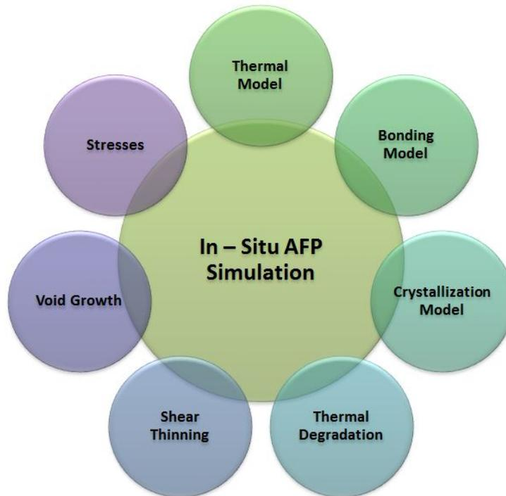
**Figure 2.3:** Various process models for the simulation of in - situ AFP process.
