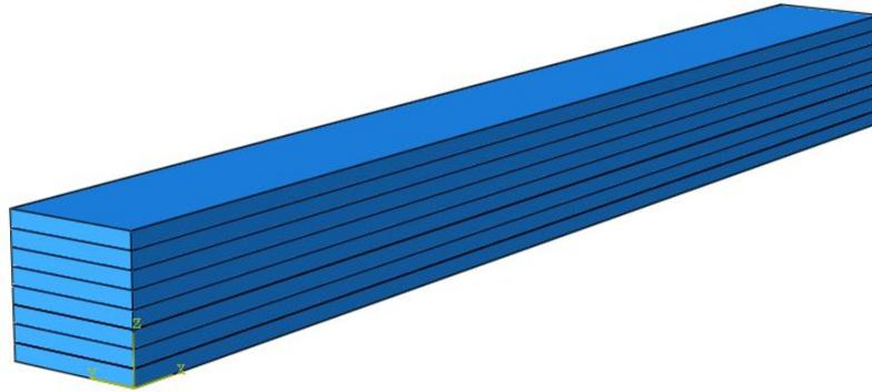
**Figure 3.4:** The 3D laminate model in ABAQUS consisting of 8-ply laminate.
