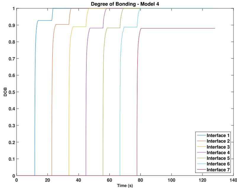
**Figure 6.4:** Degree of bonding achieved at each interface of the laminate for Model 4.
