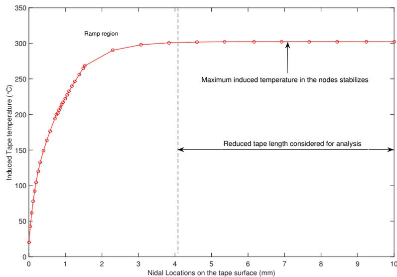
**Figure 4.13:** Maximum temperatures at the nodes for a 10 mm long tape length.
