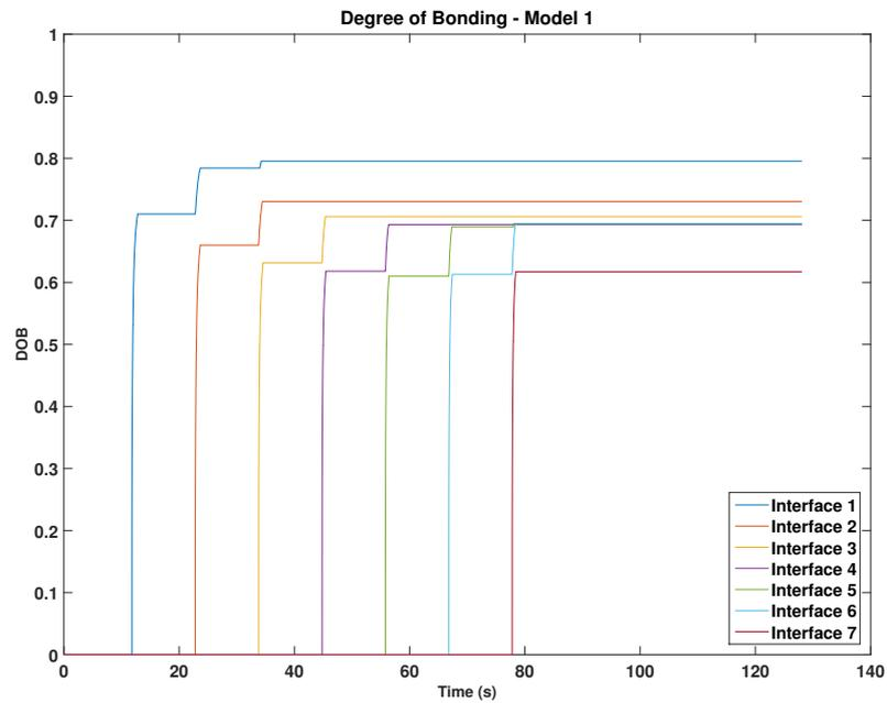
**Figure 6.2:** Degree of bonding achieved at each interface of the laminate for Model 1.
