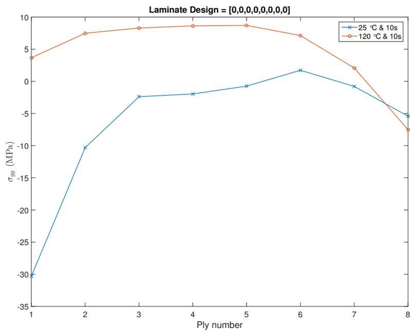
**Figure 7.2:** Residual Stress ( $\sigma_{yy}$ ) along the global Y direction of each layer in the laminate at the end of the in - situ placement process.
