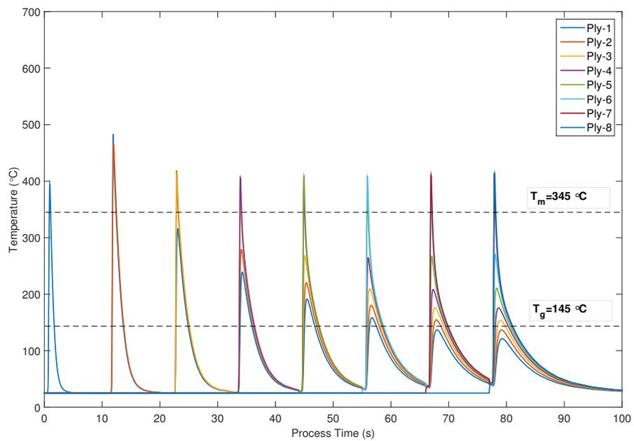
**Figure 5.34:** Thermal history for all tape layers of an 8 ply cross ply laminate,  $[0, 90, 90, 0]_s$
