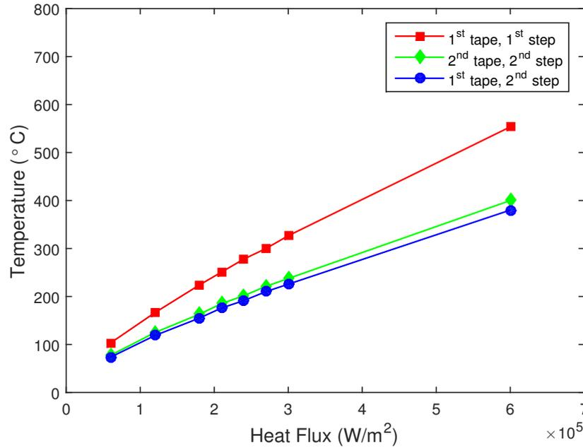
**Figure 4.17:** Heat sensitivity analysis for low heat fluxes on two tape layers.
