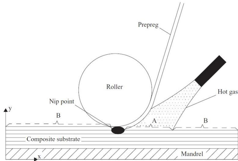
**Figure 3.3:** The schematic diagram of the 2D modelling of the thermoplastic composite prepreg lay-up process (A - Boundary impacted by heat, B - Boundary under natural convection). [49]
