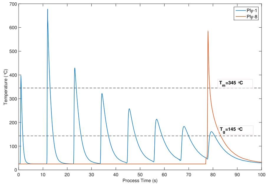
**Figure 5.7:** Comparison of the thermal history of the first tape layer and last placed layer: Model 2 - No tool heating, 10 seconds pass time and variable heat flux.
