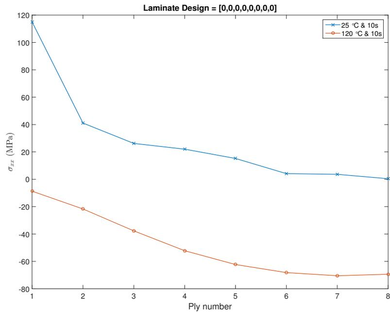
**Figure 7.1:** Residual Stress ( $\sigma_{xx}$ ) along the global X direction of each layer in the laminate at the end of the in - situ placement process.
