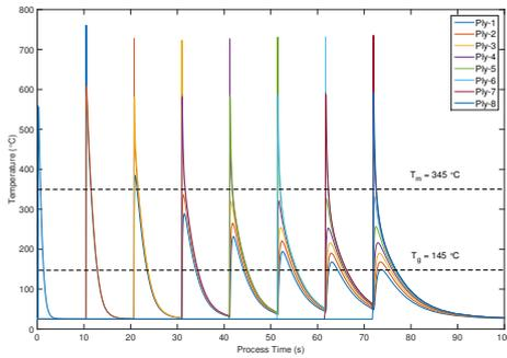
(a) Model v1 - 40 mm/s, 25 (°C) tool temperature & 2.1 mm heating length).
