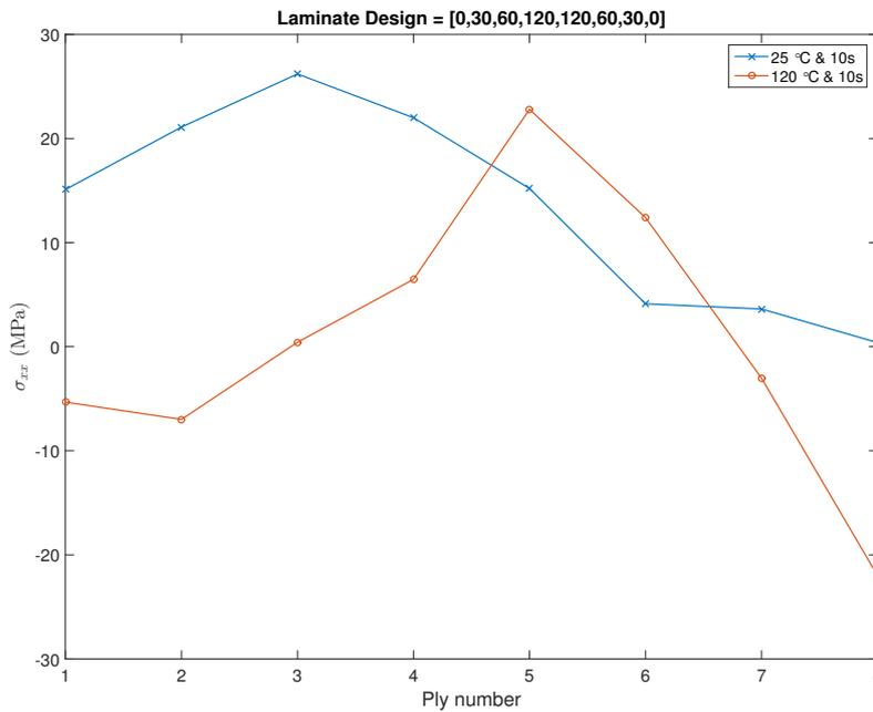
**Figure 7.7:** Residual Stress ( $\sigma_{xx}$ ) along the global X direction of each layer in the laminate at the end of the in - situ placement process.
