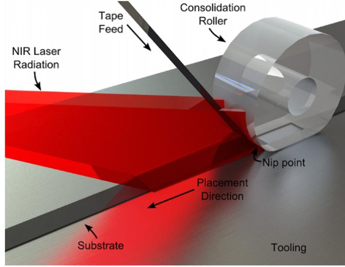
Figure 2.2: The in - situ consolidation technique in AFP process [20].
