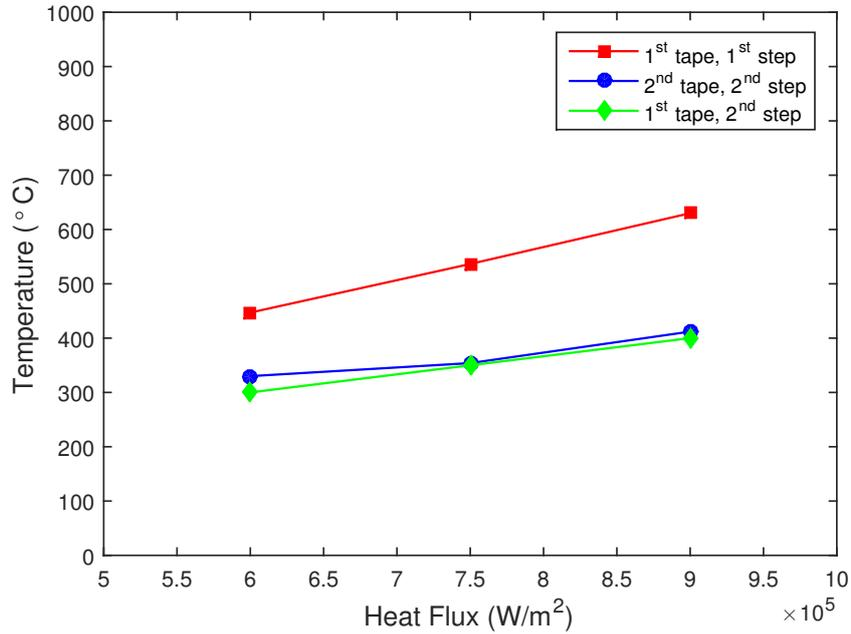
**Figure 4.18:** Heat sensitivity analysis for high heat fluxes on two tape layers.
