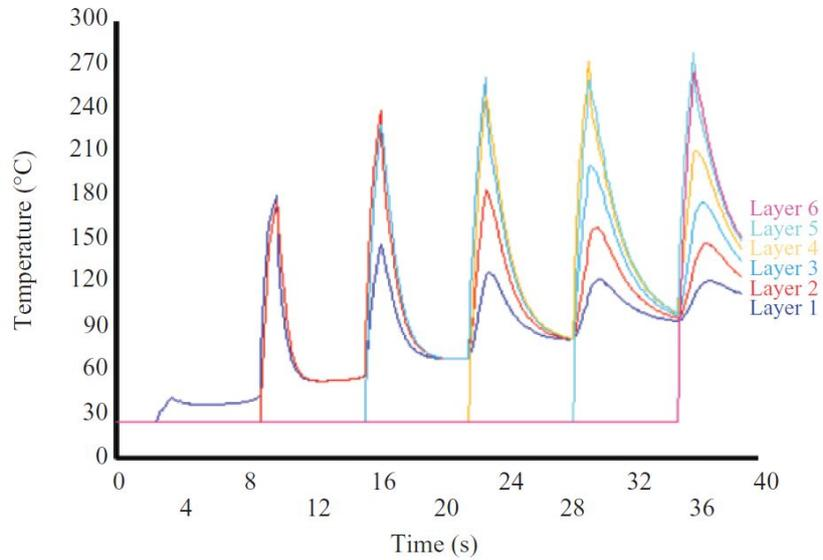
**Figure 5.37:** Temperature history in the all tape layer of a 6 layer placement process. [49]
