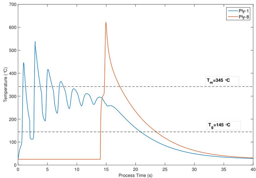
**Figure 5.18:** Comparison of the thermal history of the first tape layer and last placed layer: Model-6.
