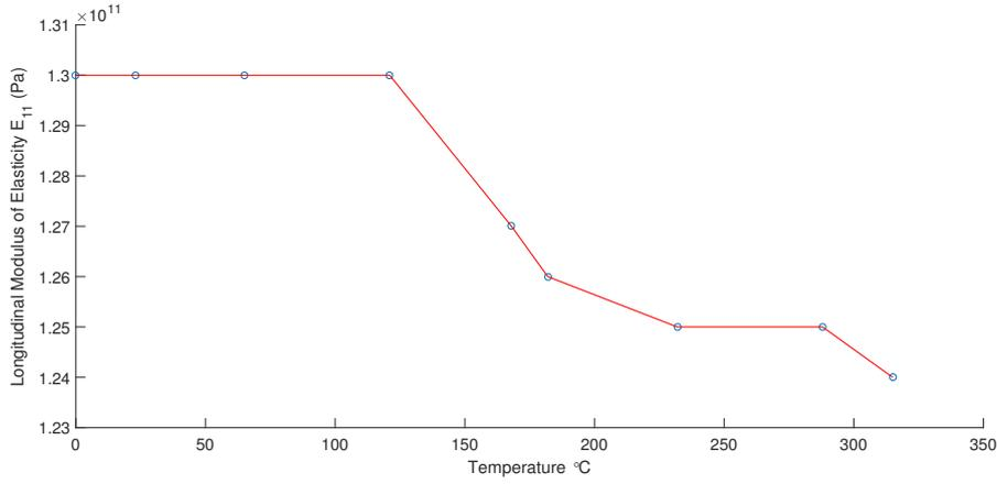
**Figure 4.1:** Variation of the longitudinal modulus of APC-2 with respect to temperature [11].
