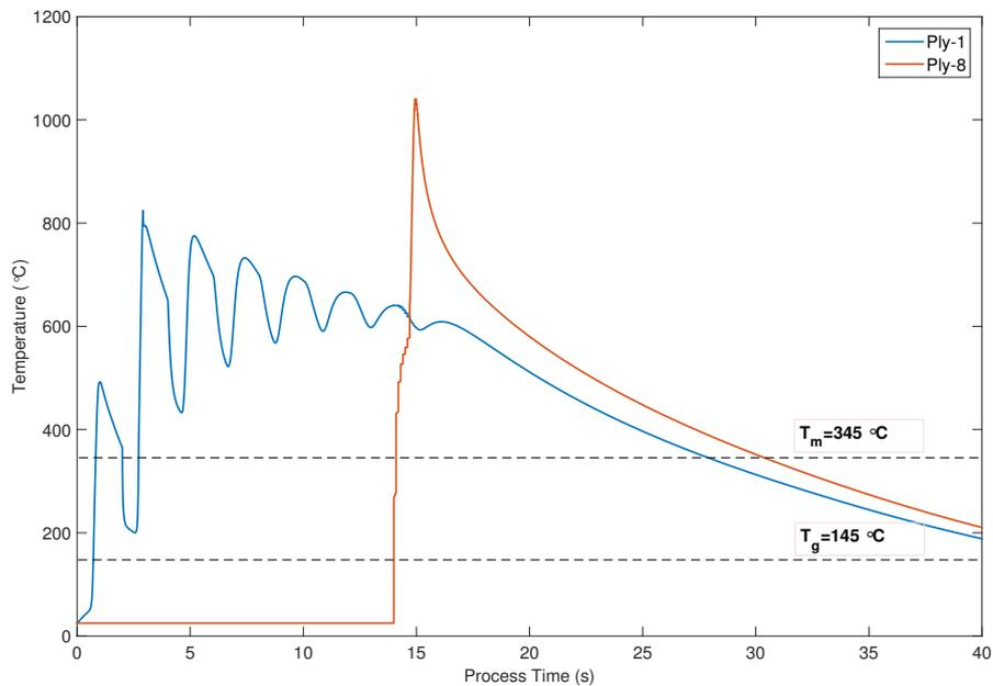
**Figure 5.28:** Comparison of the thermal history of the first tape layer and last placed layer: Model-15.
