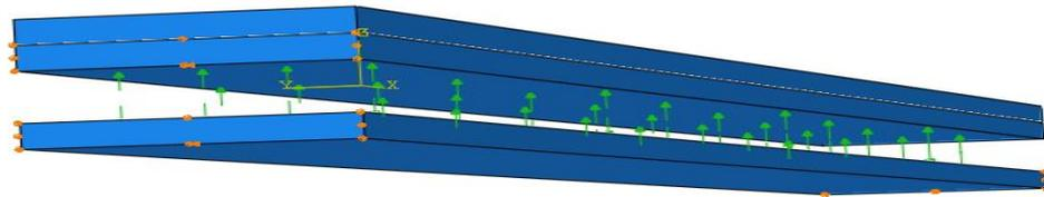
**Figure 4.5:** The heat flux load applied to the base of the second tape layer during the step 'S2', as shown by the green arrows. (Tape layers shown here are in an exploded view.)
