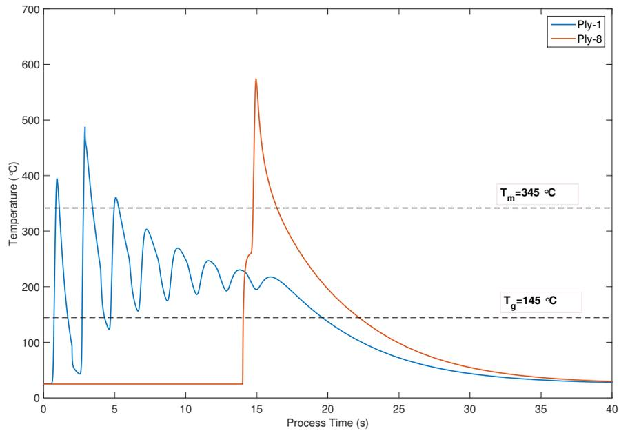
**Figure 5.17:** Comparison of the thermal history of the first tape layer and last placed layer: Model-5.
