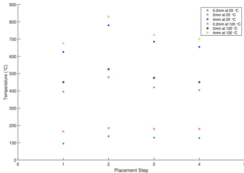
**Figure 4.19:** The maximum temperature induced in the tape surfaces for heating lengths: 0.2mm, 2mm and 4mm with tool temperature at 25 °C and 120 °C.
