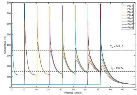
(b) Model v2 - 40 mm/s, 120 (°C) tool temperature & 2.1 mm heating length.
