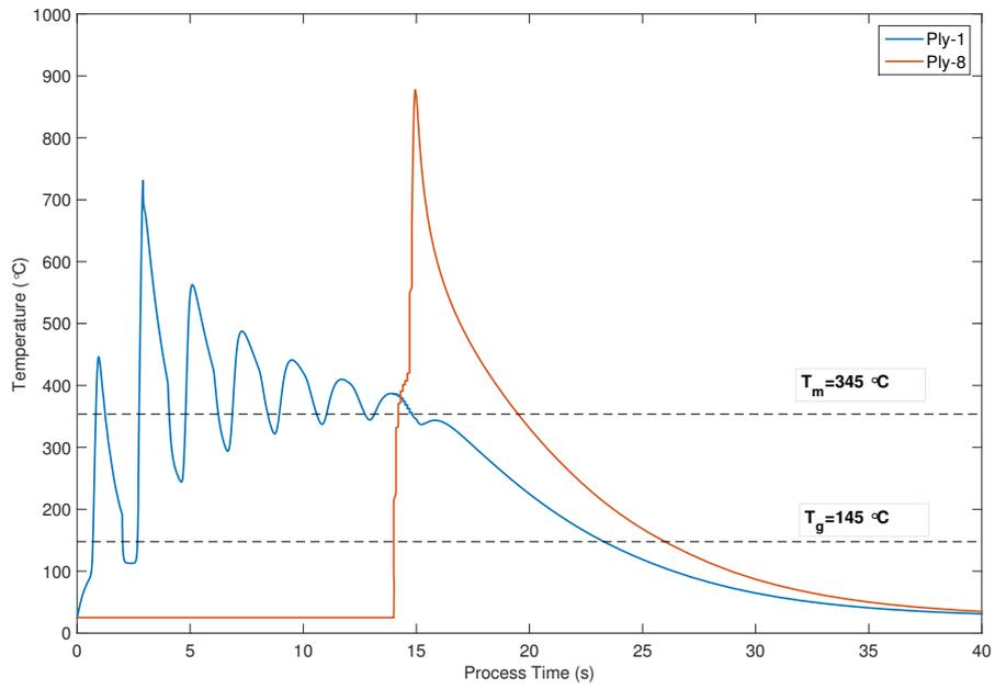
**Figure 5.19:** Comparison of the thermal history of the first tape layer and last placed layer: Model-7.
