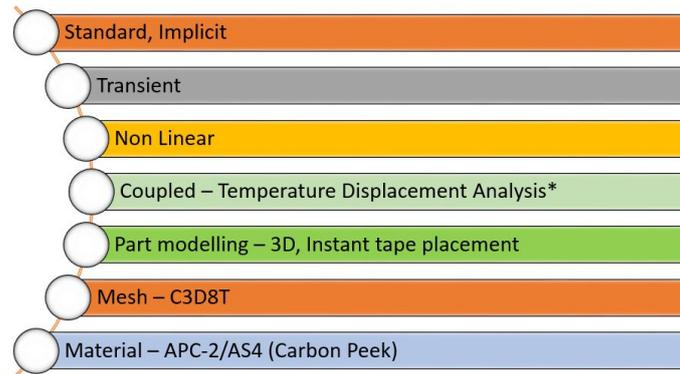
**Figure 3.2:** Simulation strategies for modelling the in - situ AFP process using ABAQUS FE software.
