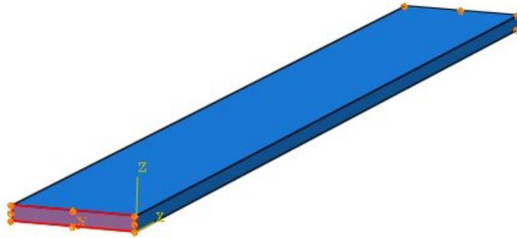
**Figure 4.8:** Boundary condition, BC-1, at the start of the tape length, created in the placement step.
