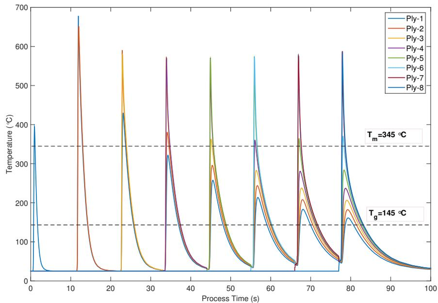
**Figure 5.8:** Thermal history of all tape layers: Model 2 - No tool heating, 10 seconds pass time and variable heat flux.
