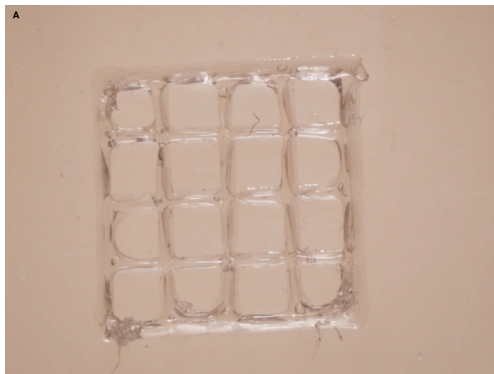
Figure 21: (a) Top view close-up of the M927 3D printed 32 layered construct. Image derived with Olympus SZ61. (b) Slanted view of the M927 3D printed 32 layered construct
