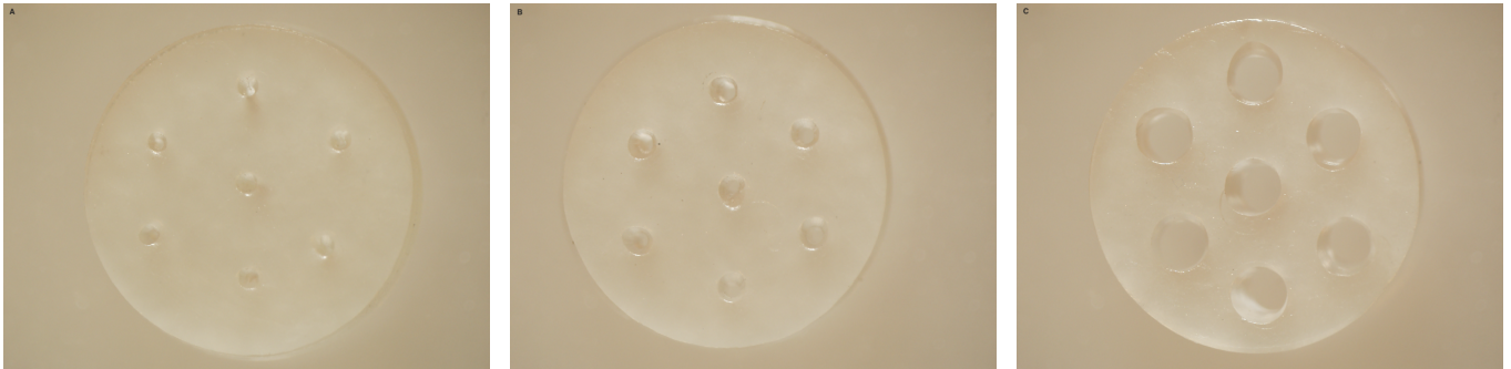
Figure 11: Top view close-up of \varnothing 6 mm M927 samples with 7 punched 350 \mu\text{m} (a), 500 \mu\text{m} (b), and 1000 \mu\text{m} holes (c). Image derived with Olympus SZ61.
