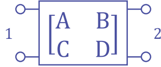
Figure D.2 – ABCD-matrix representation of a two-port network.
