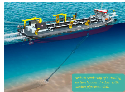
Figure 3.2: Mechanical-Hydraulic dredger: Trailing Suction Hopper. Hydraulic suction and mechanical are combined in this method. (IADC, 2014b).
