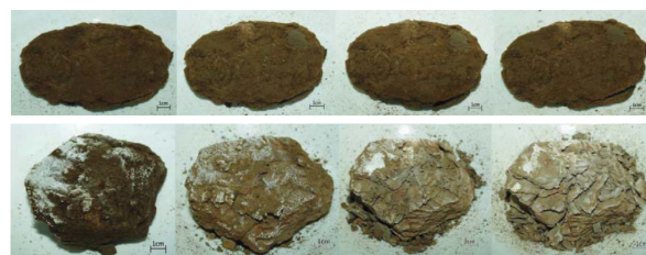
Figure 2.12: Lump submerged in water (top); lump exposed to 4 wetting-drying cycles (bottom) (Kostkanová et al., 2014).
