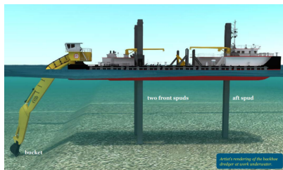
Figure 3.1: Mechanical dredger: Backhoe. A backhoe dredges the material by a single dredging bucket. (IADC, 2014a).
