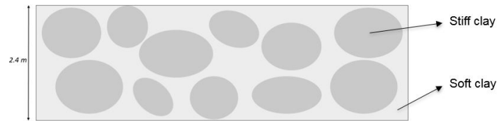
Figure 1.2: Schematic profile of clay lumps before preloading: a matrix of stiff lumps and interlump void space filled by water.
