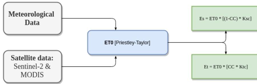
Figure 3: Atmospherically corrected Sentinel 2a, MODIS LST and Albedo products, and meteorological data have been used to construct potential evaporation estimates for the study area. Within the evaporation framework the canopy cover [CC] is used to derive between potential soil evaporation and transpiration.
