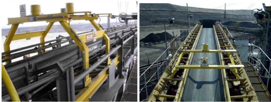
**Fig. 6** Radiometric sensor measurement device, installed on the conveyor belt, measuring blend of coal resulting from multiple excavators, just before the stock pile
