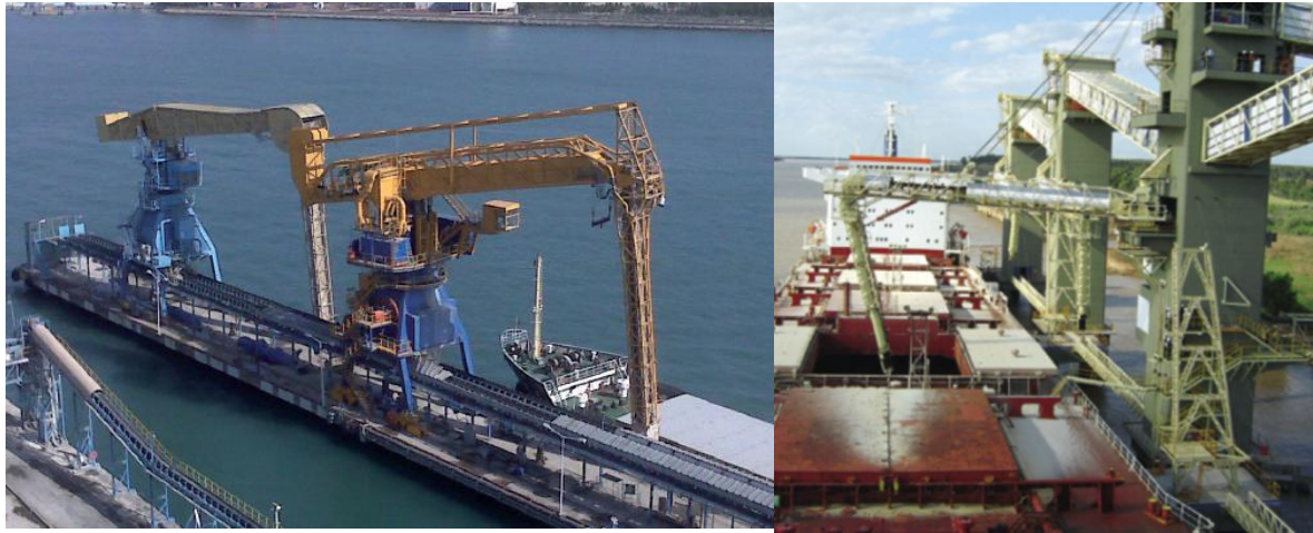
Figure 61 - Left: Multibelt ship unloader [Neuero]. Right: Portaloader ship loader [Bühler]
