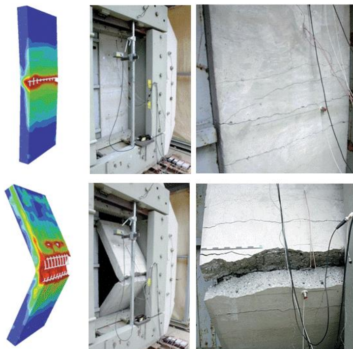
Figure 2.2: Walls after the blast. Top wall: NRC-3. Bottom wall: NRC-4
