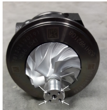
(b) Modified turbocharger rotor-bearing system: front view. Grub screws can be inserted in the holes indicated by the arrows.
