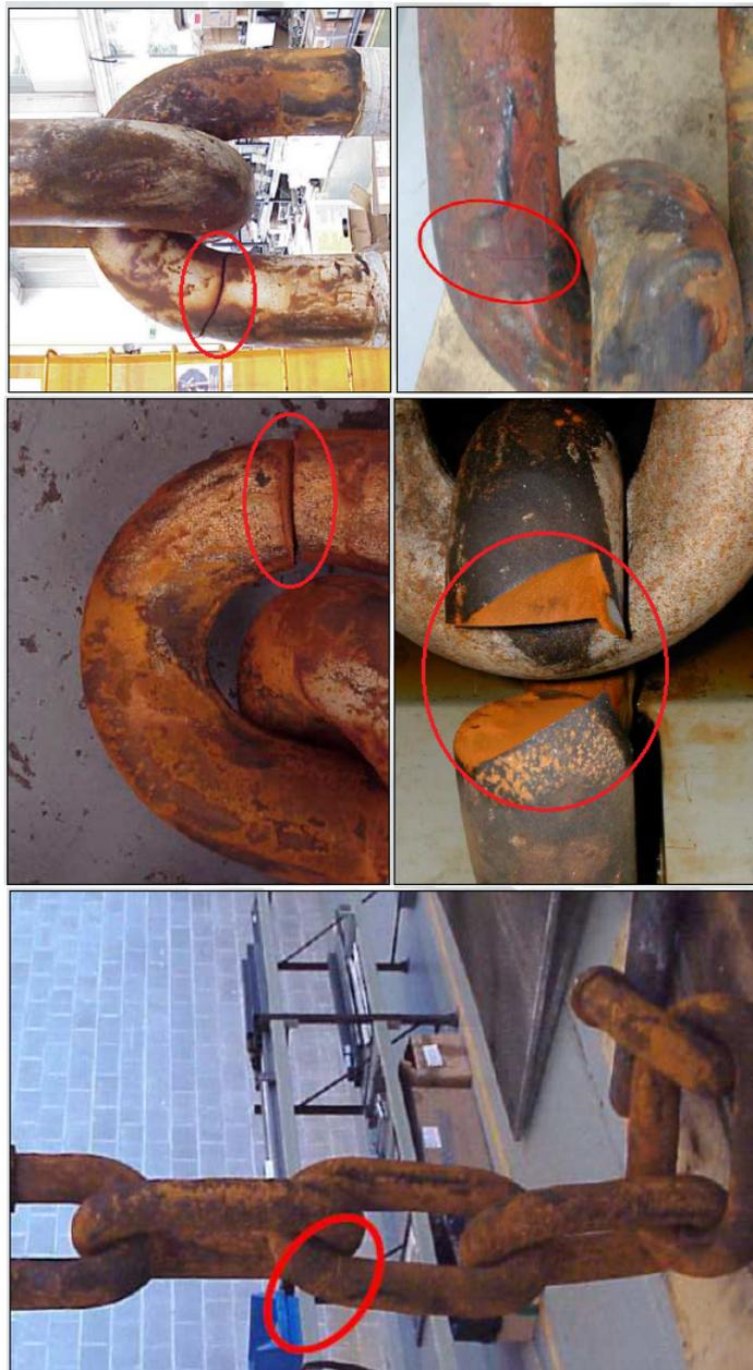
Figure 6.18: The fracture locations on the link, from different angles [Fernandez, 2008]
