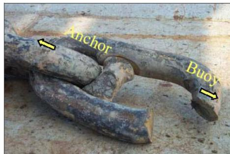
Figure 6.17: The fracture location on a chain link [Fernandez, 2008]
