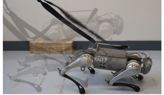
Fig. 4: Real Go1 Quadruped performing a jumping motion.
