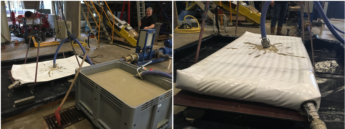
Figure 3.18: Left photo showing the set up of the filling tests. Right photo shows the square mattress filled with the fluid.
