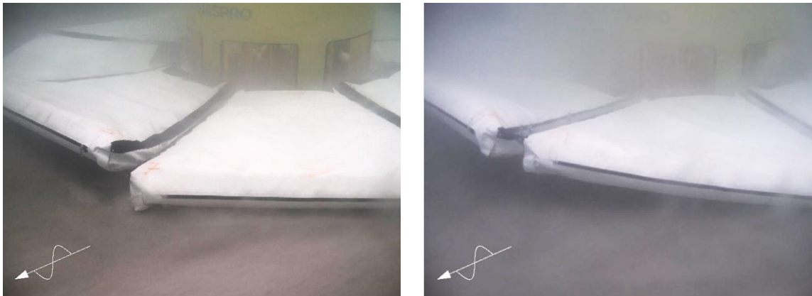
Figure 7.1: Left photo showing loose ballast filled mattress components, right photo showing the ballast filled mattress connected to each other
