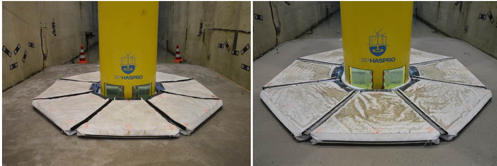
Figure 3.13: Left figure showing loose BFMs around the monopile, right showing the connected BFMs around the monopile
