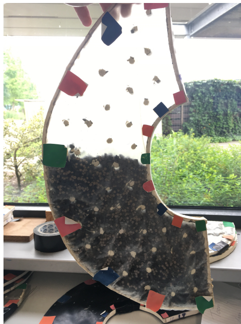
Figure 3.5: Photo showing the partly filled flexible ballast filled mattress
