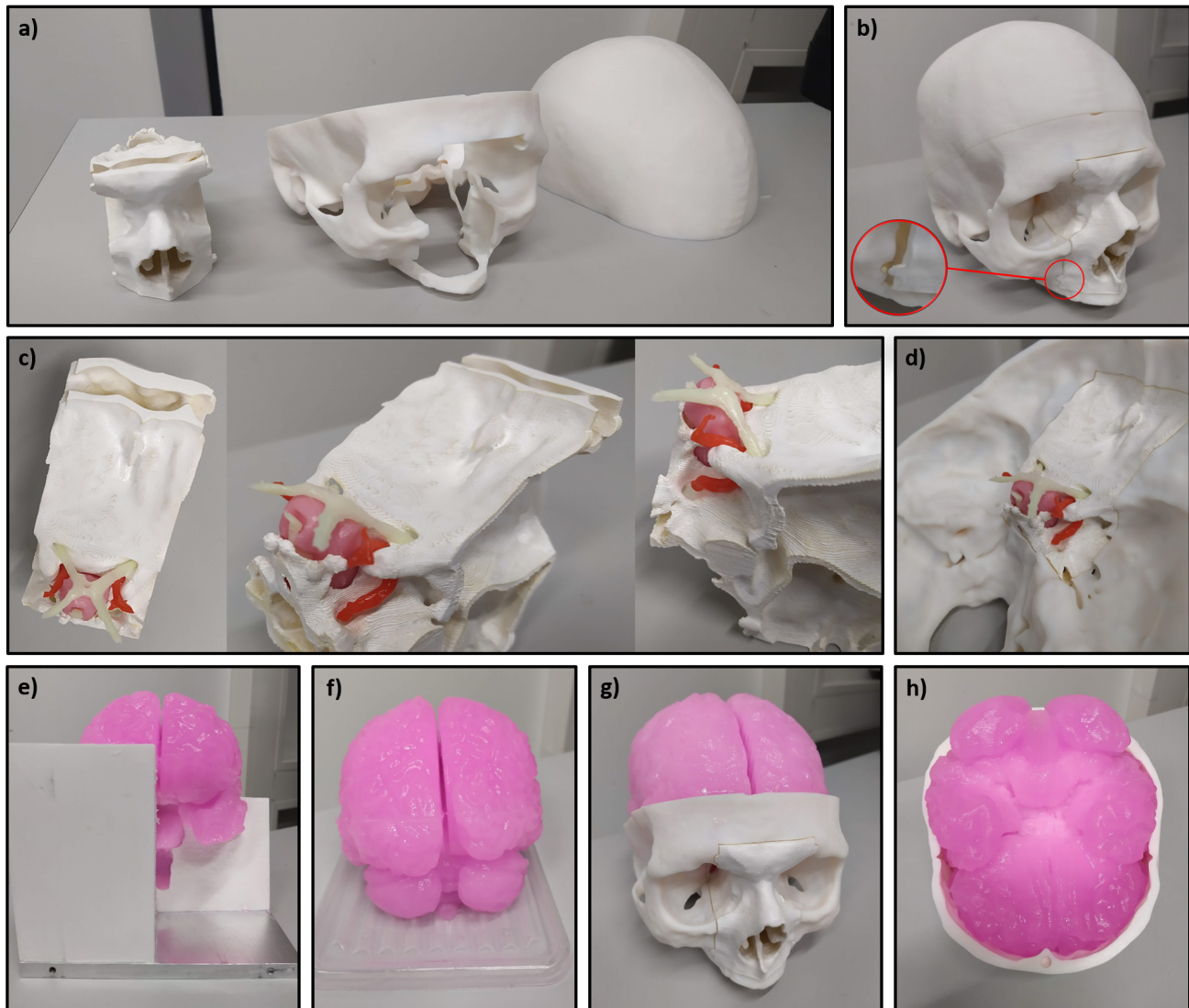
Figure 7. Final head phantom. a) Skull phantom disassembled into its three parts. b) Assembled skull and zoom-in view on the side groove of the maxilla that improves the fitting of the nasal cavity insert into the skull phantom. c) Upper and side views of the nasal cavity and skull-base inserts. d) Back view of the nasal cavity inserted inside the skull. e) Front view of the brain phantom, partially inside the mold. f) Back view of the brain phantom. g) Brain phantom placed inside the skull. h) Brain phantom viewed from below, inserted inside the calvarium of the skull.
