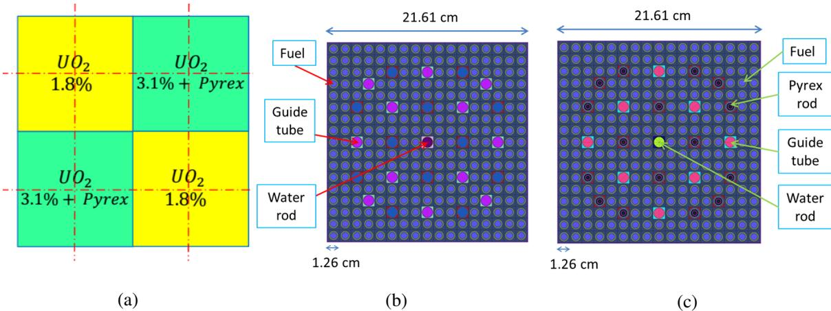
**Figure 1:** Assembly-set under study (a) and layout of  $UO_2$  fuel assemblies with 1.8 % enrichment (b) and 3.1 % enrichment and Pyrex (c). Symmetry axis along which reflective boundary conditions are set are shown in (a). A nodalization of  $2 \times 2$  nodes per assembly is chosen.
