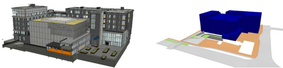
1 Example of a BIM model of building design (left) and a BIM model of a Detailed Plan (right). Figure by Future Insight Group (2023).
