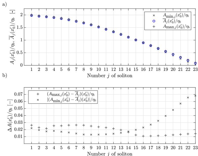
**Fig. 15.** Comparison of the tKdV-NFT results from the different 206 time series of experiment No.20: a) Relative values of mean amplitude  $\bar{A}_j(x'_0)/\eta_b$ , minimum and maximum amplitudes  $A_{\min,j}(x'_0)$  and  $A_{\max,j}(x'_0)$  for each of the largest 23 solitons,  $1 \leq j \leq 23$ , calculated at the 206 gauge positions. b) Deviations between mean and minimum value and between mean and maximum value for each soliton.
