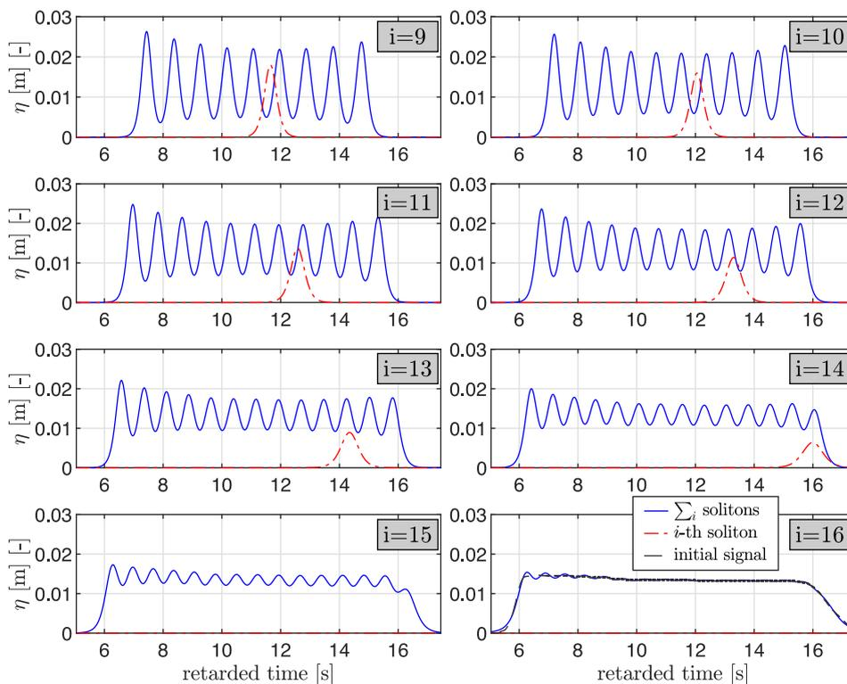
**Fig. 19.** The inverse KdV-NFT of a stepwise completed spectrum for the data at CG1' (part 2): The solitons are added one by one to the spectrum in order of amplitude, starting from the tallest ( $j = 1$ ). The inverse KdV-NFT of the first twelve spectra is presented in Fig. 18. The blue lines here show those of the remaining spectra. (For interpretation of the references to colour in this figure legend, the reader is referred to the web version of this article.)
