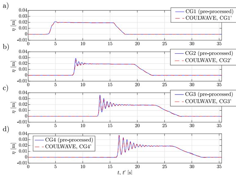
**Fig. 5.** Comparison of pre-processed near-field data  $\eta(x_0, t)$  for experiment No.20 obtained from gauges CG1 to CG4 (filtered and scaled data with zero extension, blue lines) and  $\eta(x'_0, t')$  from numerical simulation gauges CG1' to CG4' (red lines) at numerical flume positions  $x' = 0.01$  m, 4.694 m, 9.689 m and 13.676 m. (For interpretation of the references to colour in this figure legend, the reader is referred to the web version of this article.)
