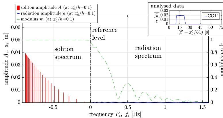
**Fig. 11.** Periodic KdV-NFT spectrum of the time series at numerical wave gauge CG1' in experiment No.20 (see upper-right plot within the figure), with the amplitudes  $A_j$  of the solitons (red bars), the amplitudes  $a_k$  of the oscillatory waves (blue triangles, both on upper left axis), and the moduli  $m_i$  (green-dashed curve, upper right axis). (For interpretation of the references to colour in this figure legend, the reader is referred to the web version of this article.)
