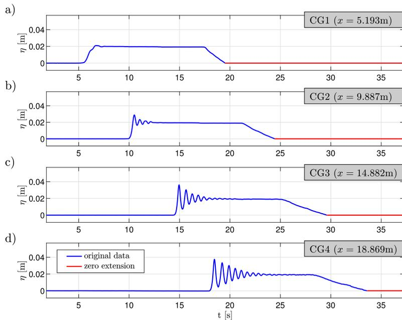
**Fig. 4.** Pre-processed free surface at CG1 to CG4 from experiment No.20 after cutting and replacing the negative elevations: Original samples after zero correction, filtering and scaling (blue lines) extended by zeros (red lines) in order to eliminate negative elevations at the back of the bore and to provide identical sample numbers in the data. (For interpretation of the references to colour in this figure legend, the reader is referred to the web version of this article.)
